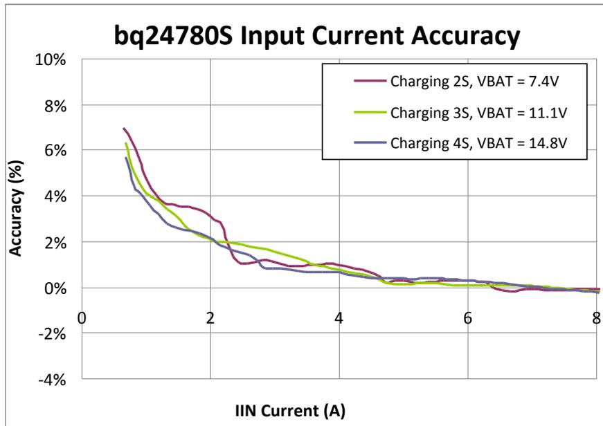
**Figure 6. TIDA-00657 Input Current Accuracy**
