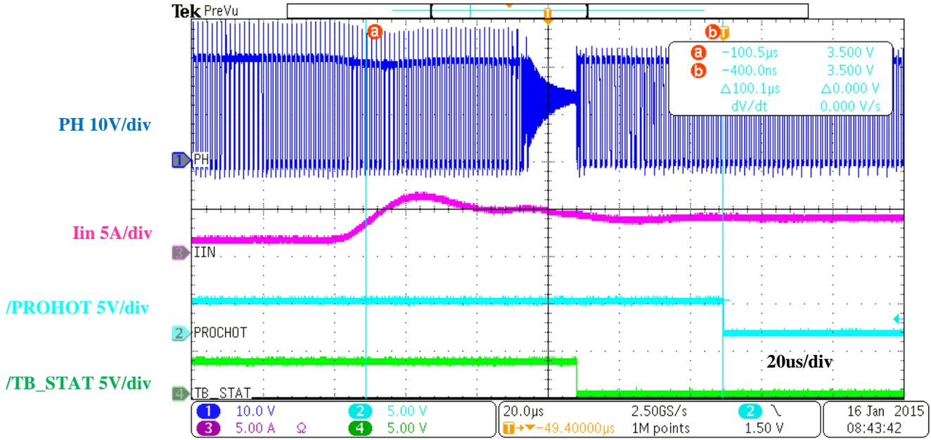
Vin=20V, VBAT = 13.3V, IIN = 2048mA, ICRIT threshold = 150%
