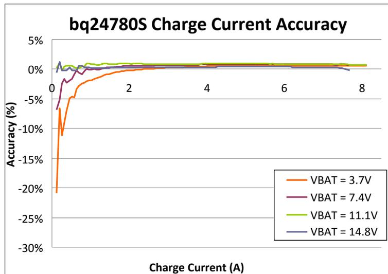
**Figure 5. TIDA-00657 Charge Current Accuracy**
