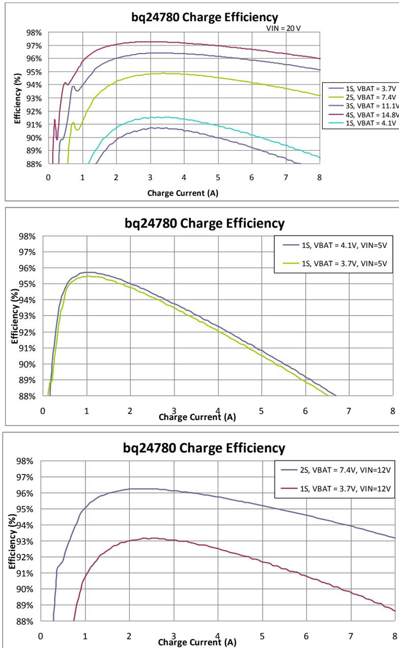
**Figure 3. TIDA-00657 Charging Efficiency**
