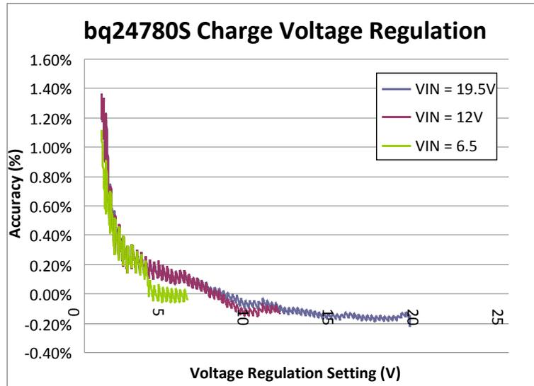
**Figure 4. TIDA-00657 Charge Voltage Accuracy**
