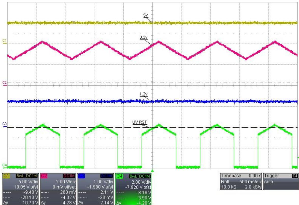
Figure 5: Reset asserted for an undervoltage fault on the 3.3 V rail
