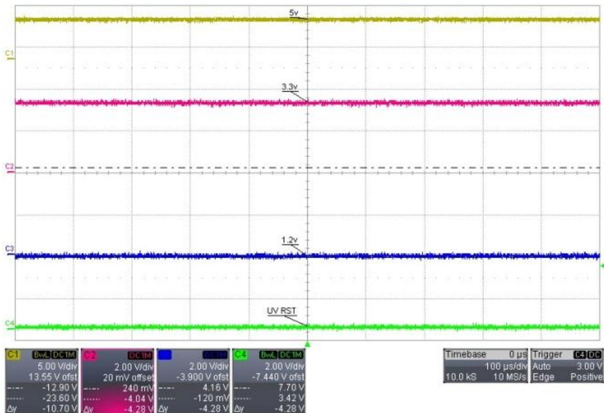
Figure A-9: Reset asserted while 3.3V rail is high and 1.2V rail is low
