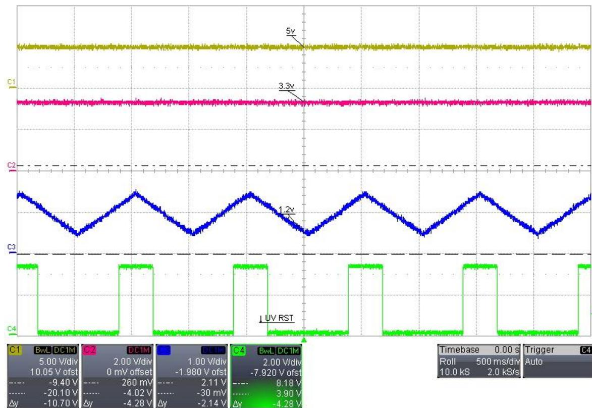
Figure 7: Reset asserted for an undervoltage fault on the 1.2 V rail
