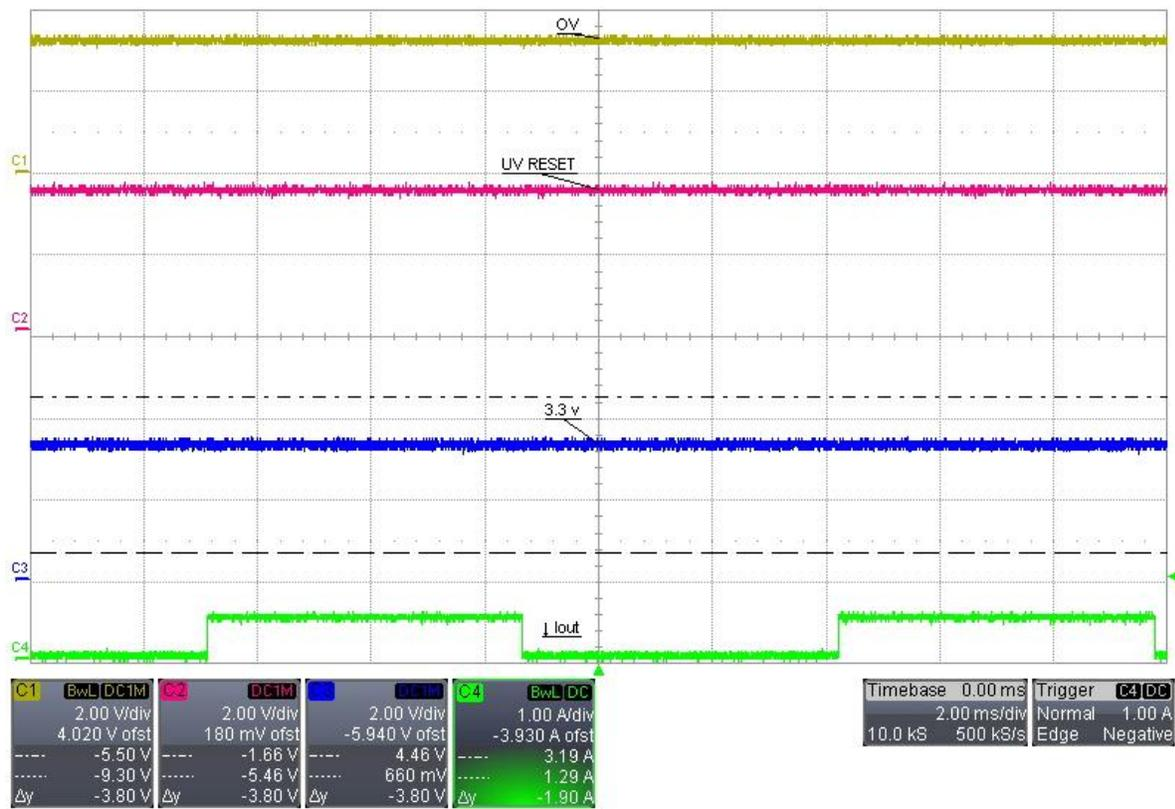
Figure A-3: Load Transient Response – 0 mA to 500 mA on 3.3 V rail
