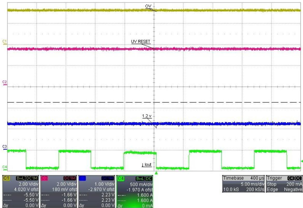
Figure A-7: Load Transient Response – 30 mA to 480 mA on 1.2 V rail
