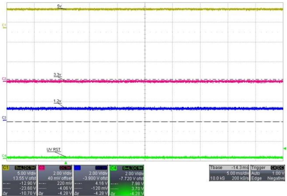
Figure A-8: Reset asserted while 3.3V rail is low and 1.2V rail is high
