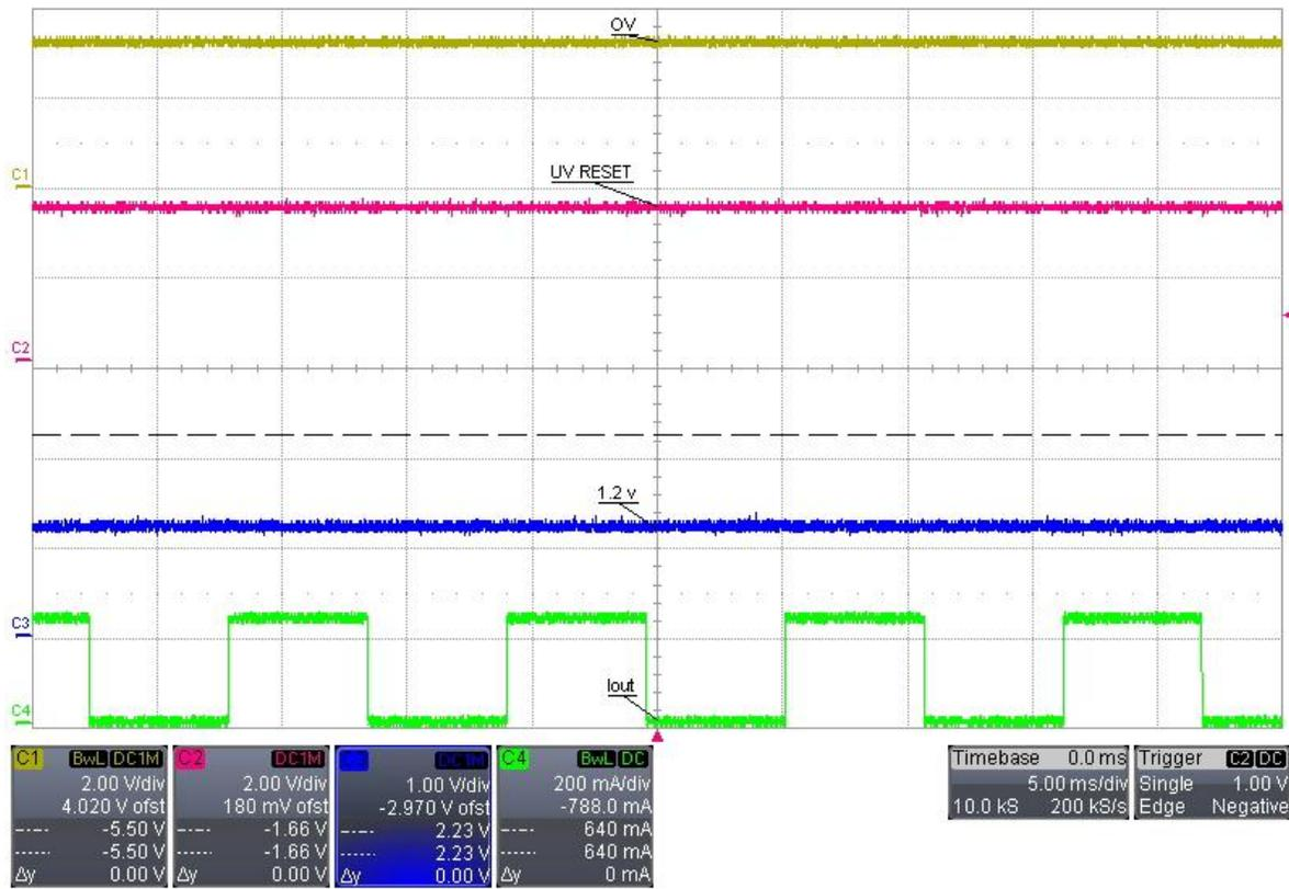
Figure A-5: Load Transient Response – 0 mA to 250 mA on 1.2 V rail
