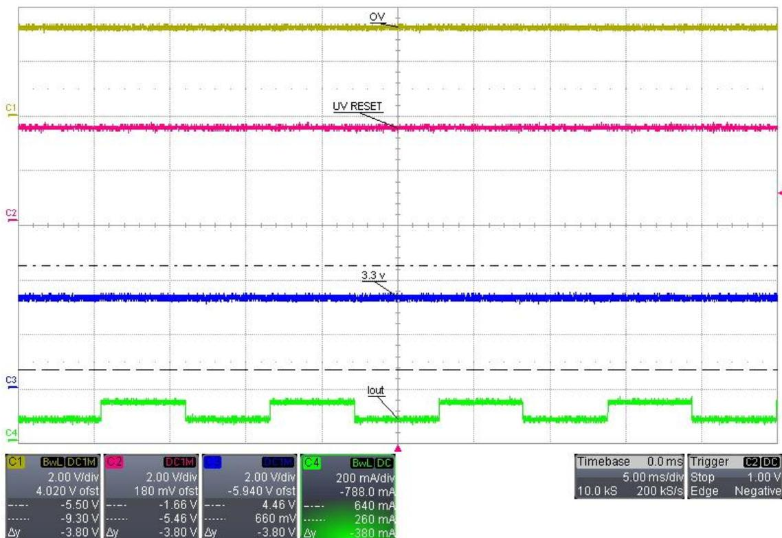
Figure A-4: Load Transient Response – 77 mA to 140 mA on 3.3 V rail
