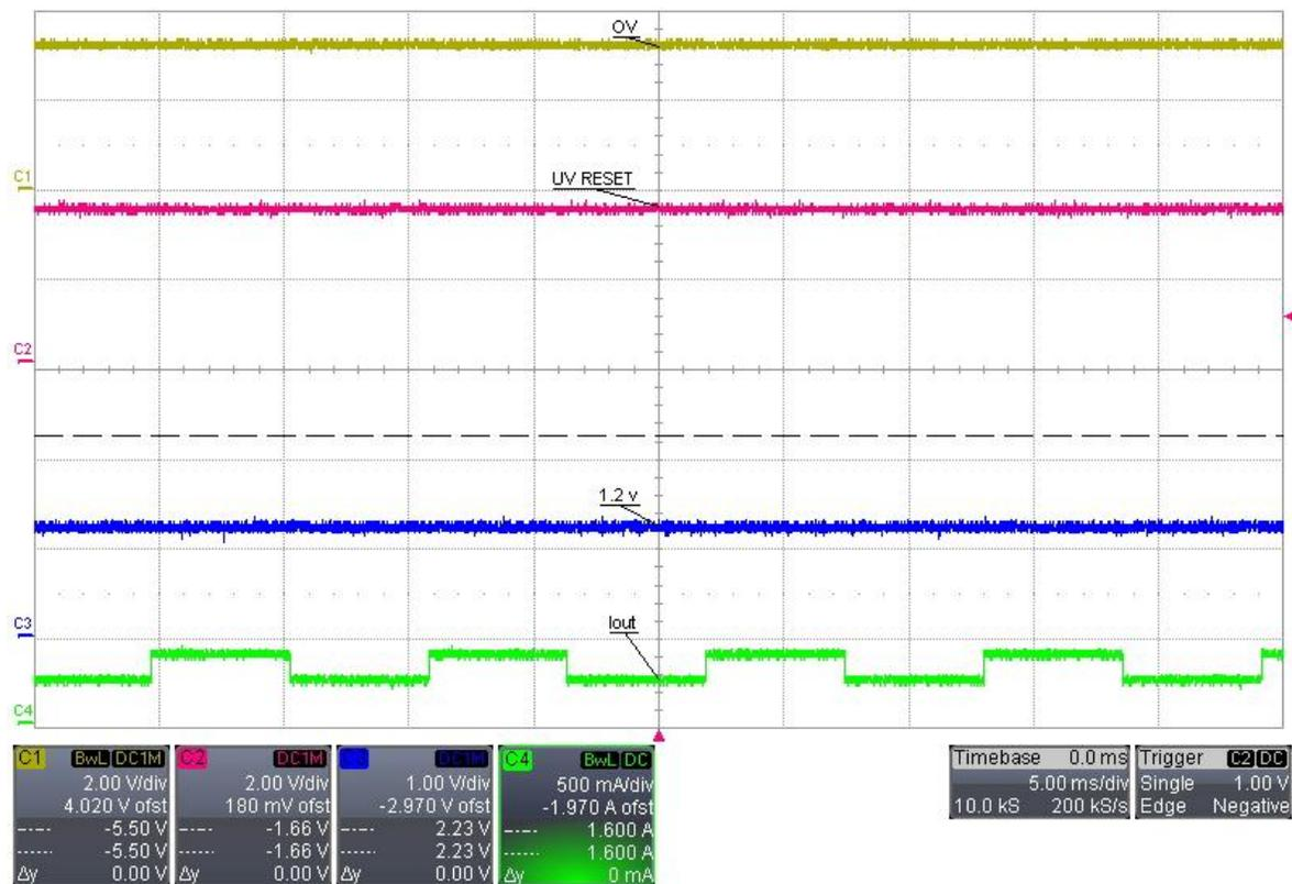
Figure A-6: Load Transient Response – 250 mA to 400 mA on 1.2 V rail.
