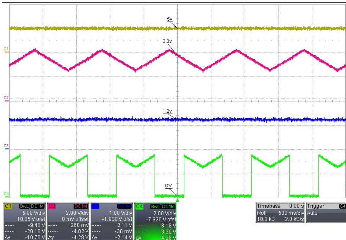
Figure 6: Reset asserted for an overvoltage fault on the 3.3 V rail
