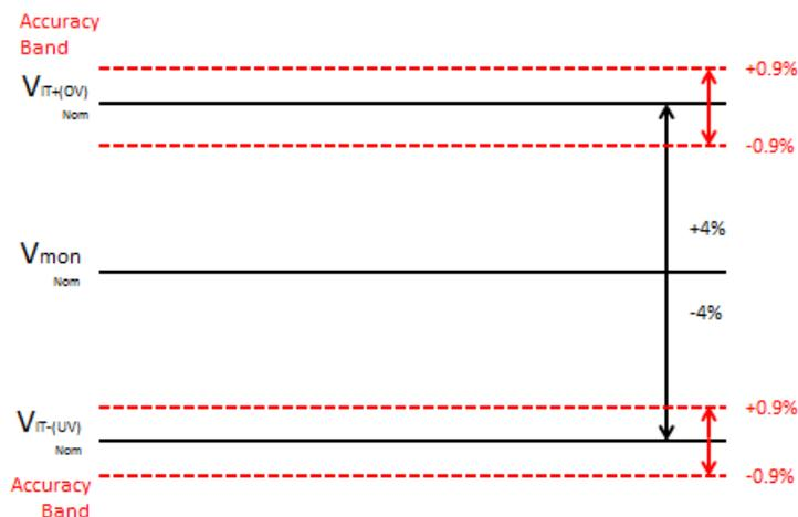
**Figure 1: TPS3702 voltage thresholds**
