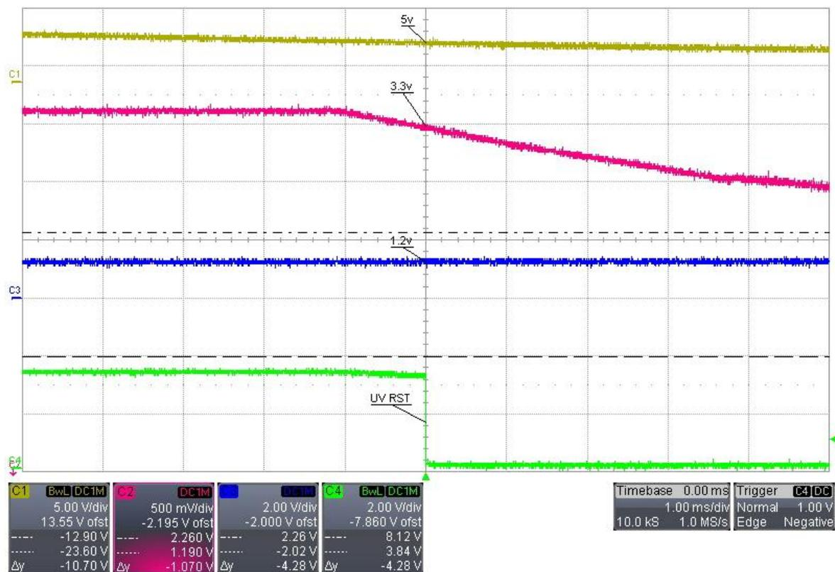
Figure A-10: Displaying how low 3.3V rail reaches until reset is asserted.
