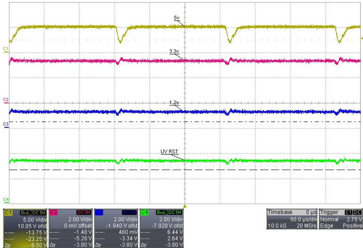
Figure 10: Brownout condition – 5 V input voltage dropping to 2.4 V for 10 µs
