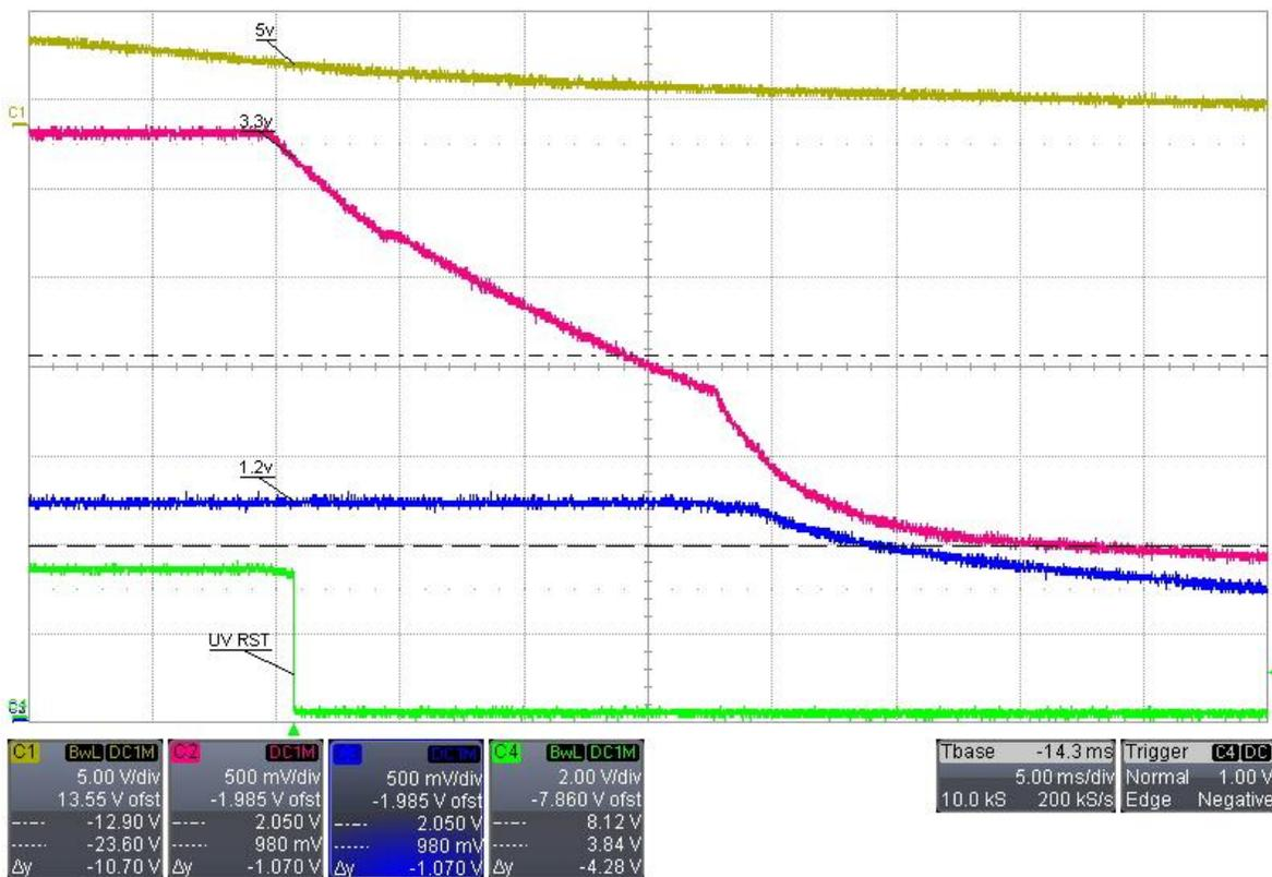
Figure 11: Slow shut down with diode maintaining bias between 3.3 V and 1.2 V rails
