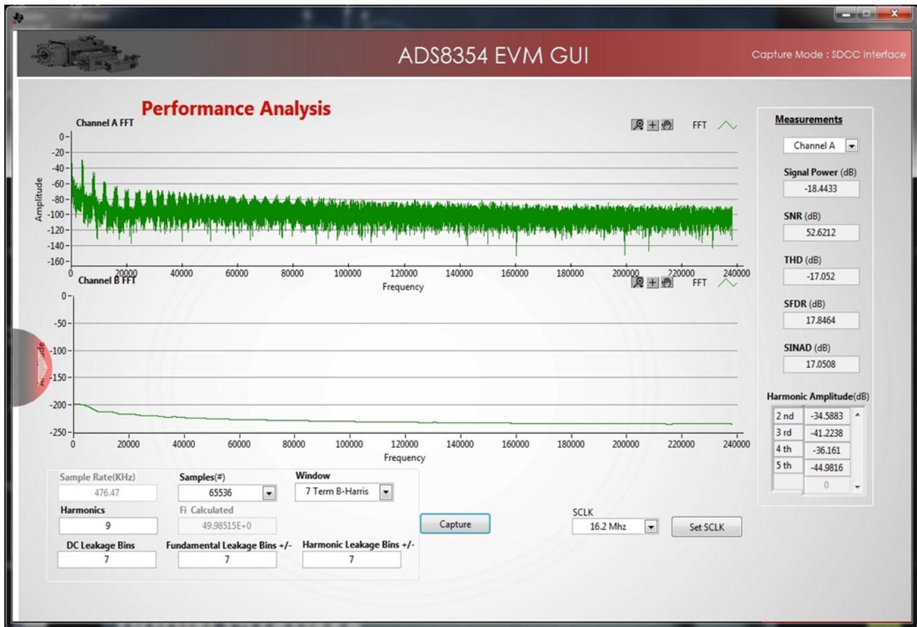
Figure 58. FFT of Motor Current (Measured Using ADS8354 EVM GUI)
