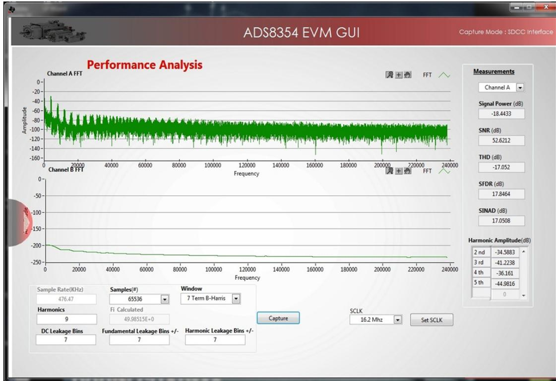
Figure 50. FFT Captured With ADS8354EVM GUI
