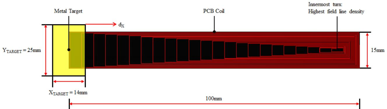
**Figure 17. Starting Position:  $d_x = 0$  mm (Top View)**
