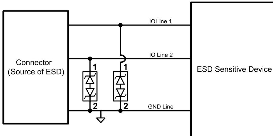
Figure 2. TPD1E10B06 Block Diagram
