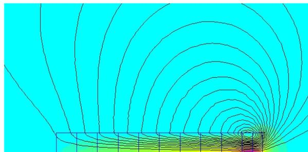
Figure 16. Simulated Magnetic Field of Asymmetric Coil
