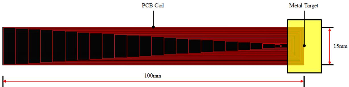
**Figure 18. Final Position:  $d_x = 100$  mm (Top View)**
