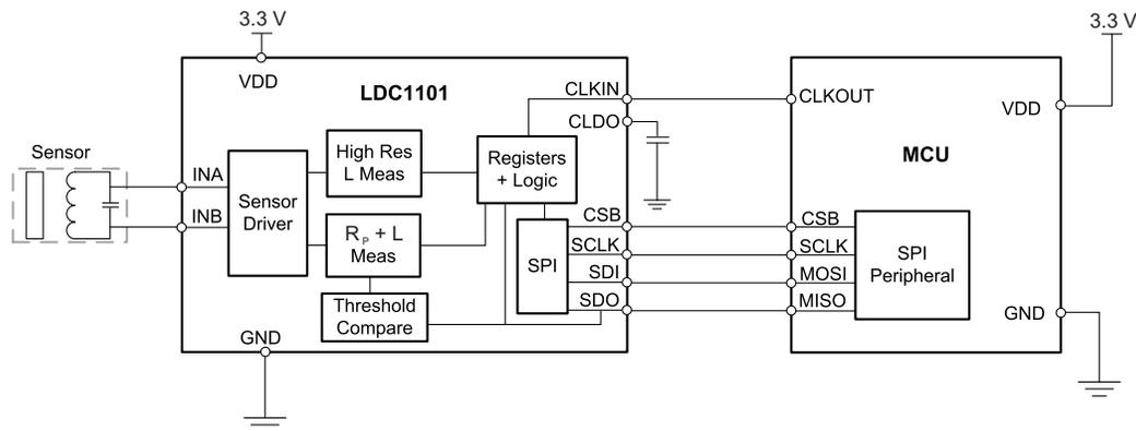
**Figure 5. LDC1101 Functional Diagram**
