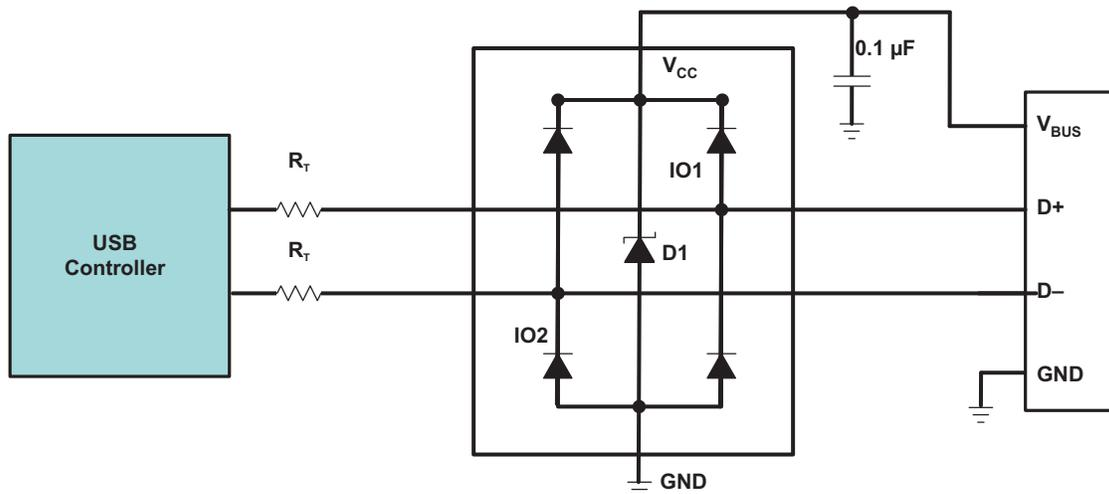
Figure 3. TPD2E001 Block Diagram
