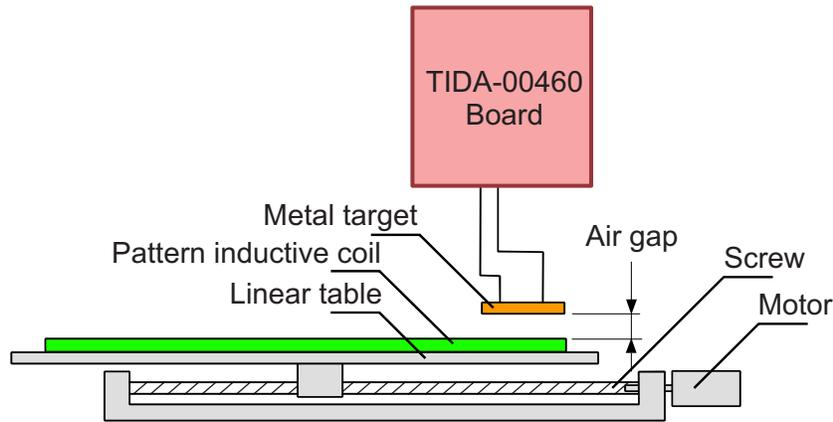
**Figure 21. Motorized Linear Table Test Setup**
