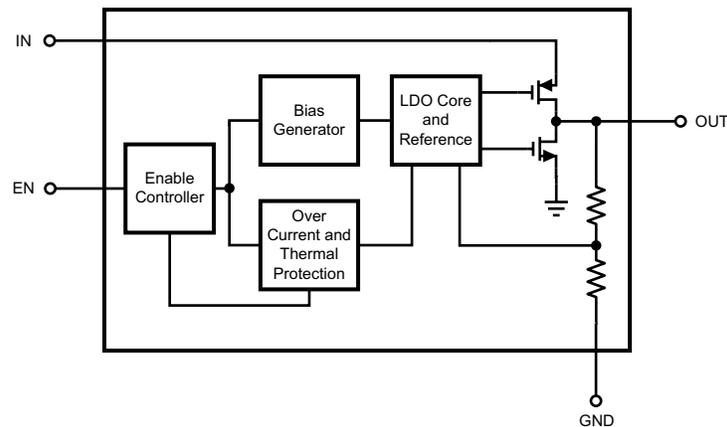
**Figure 7. LP5951 Block Diagram**
