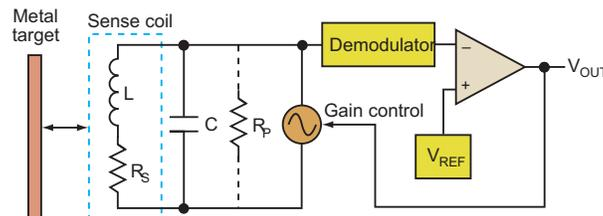
Figure 13. Oscillation Amplitude Regulation
