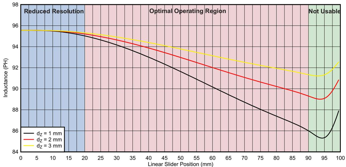
**Figure 22. Sensor Inductance Versus Distance**
