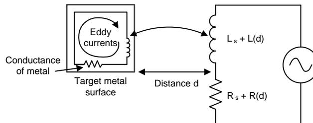
Figure 11. Metal Target Modeled as L and R With Circulating Eddy Currents
