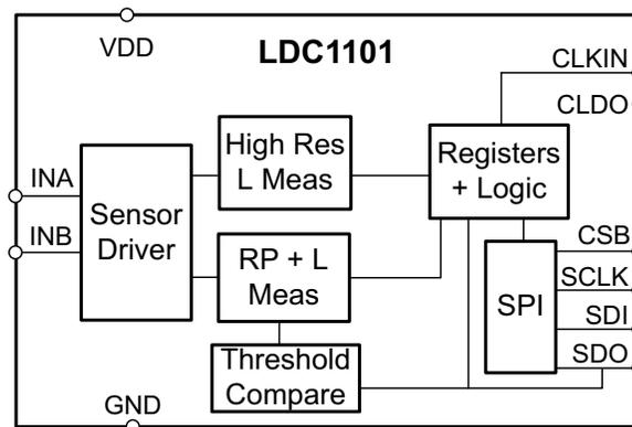
Figure 1. LDC1101 Block Diagram
