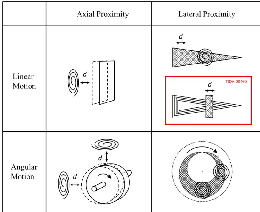
**Figure 14. Commonly Used Sensor-Target Configurations**
