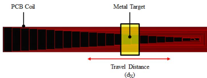
Figure 15. Lateral Movement of Rectangular Target at Position  $d_x$  (Top View)
