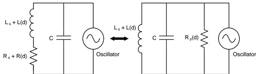
Figure 12. Series and Parallel LC Tank Circuits Connected With Oscillator
