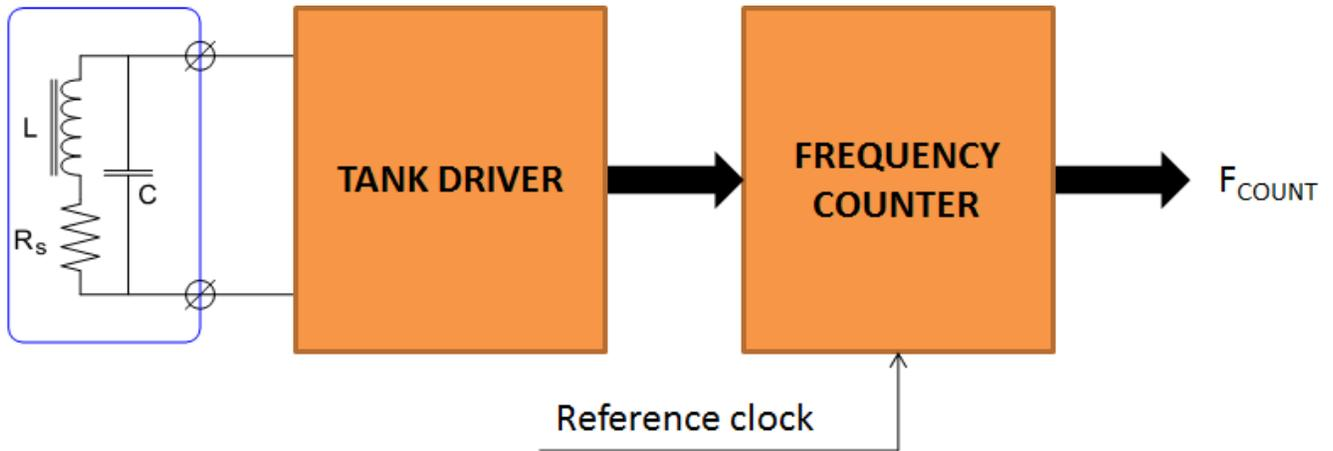
**Figure 20. Sensor Frequency Measurement**
