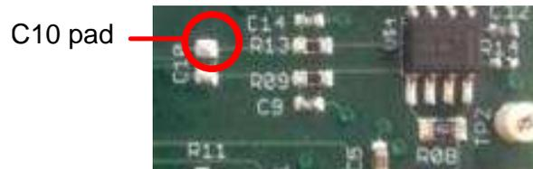
**Figure 6. Probe C10 Pad**
