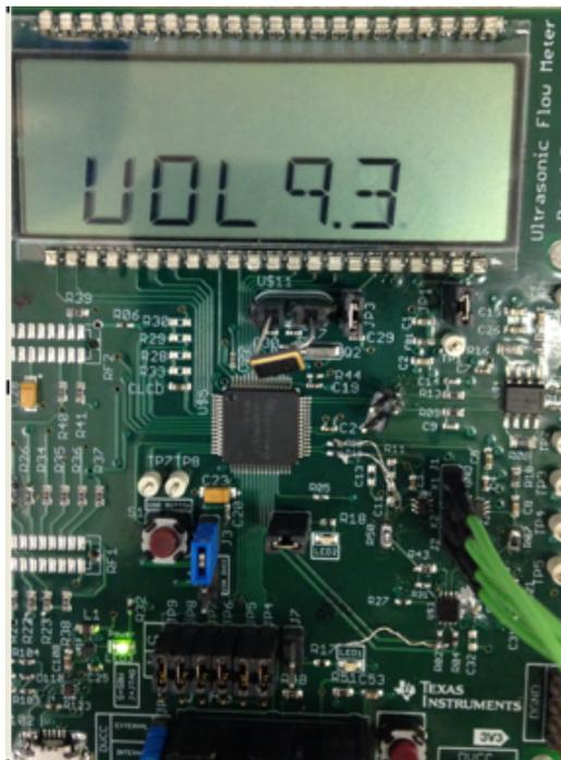
**Figure 9. Volume Displayed on LCD**
