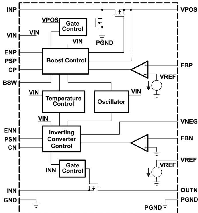
Figure 7. TPS65131 Functional Block Diagram
