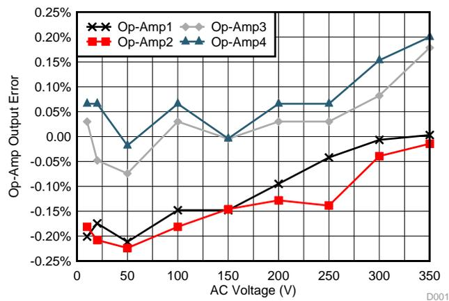
**Figure 23. AC Voltage Input versus Amplifier Output**
