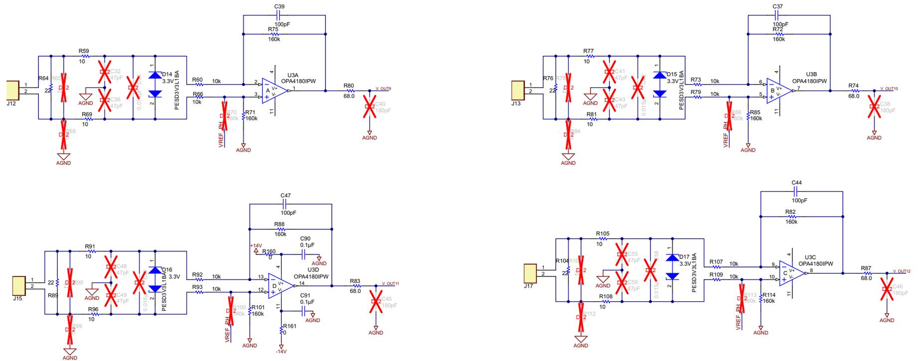
Figure 33. Differential CT Input
