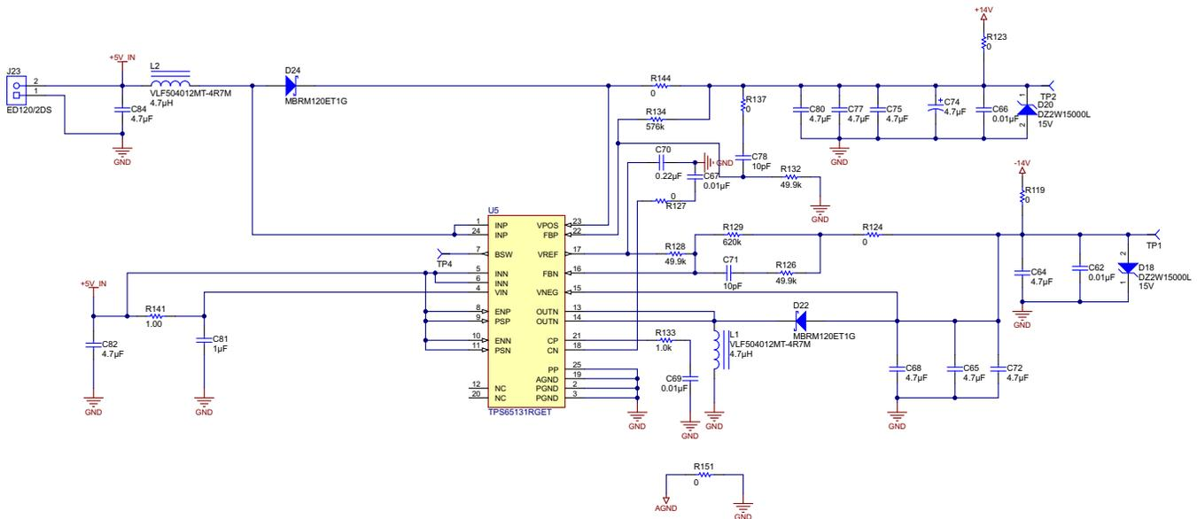
Figure 9. Dual Output DC Power Supply
