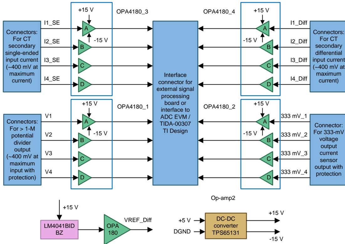
Figure 6. Voltage and Current Measurement AFE
