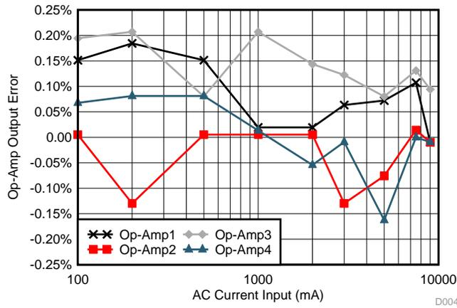
Figure 26. AC Current Input versus Amplifier Output
