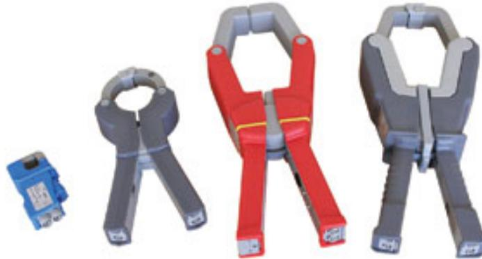
**Figure 4. Clamp-On Current Sensors**
