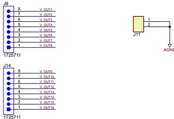
**Figure 15. External ADC Interface Connector**
