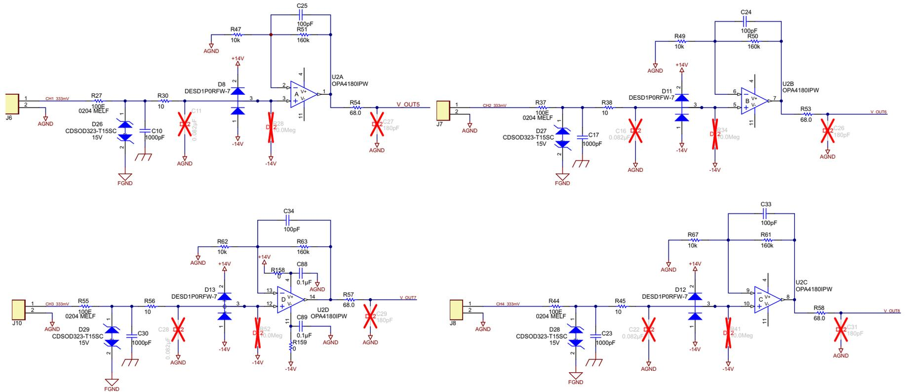
Figure 12. 333-mV Voltage Output Current Sensor Input
