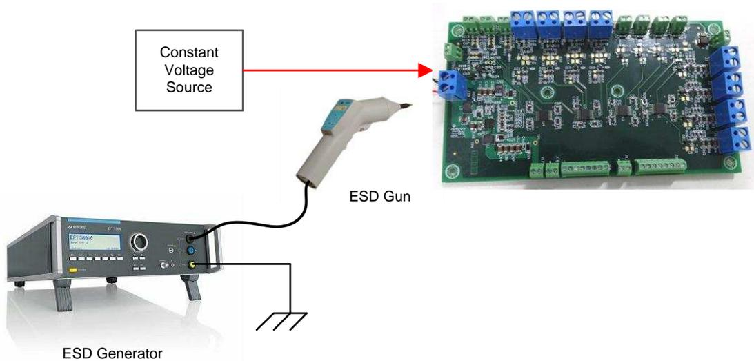
**Figure 28. ESD Setup for AFE**
