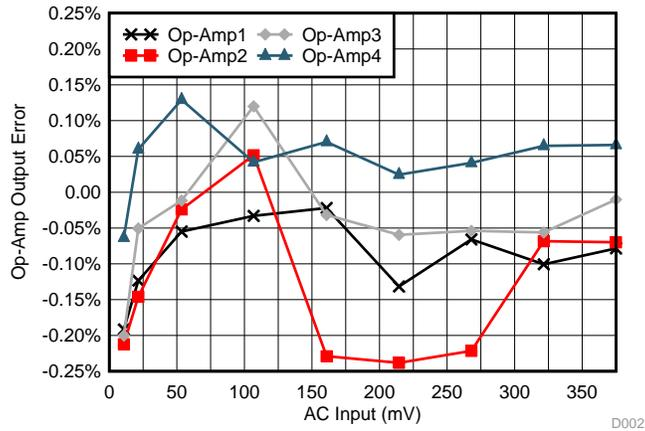
**Figure 24. 333-mV Input versus Amplifier Output**
