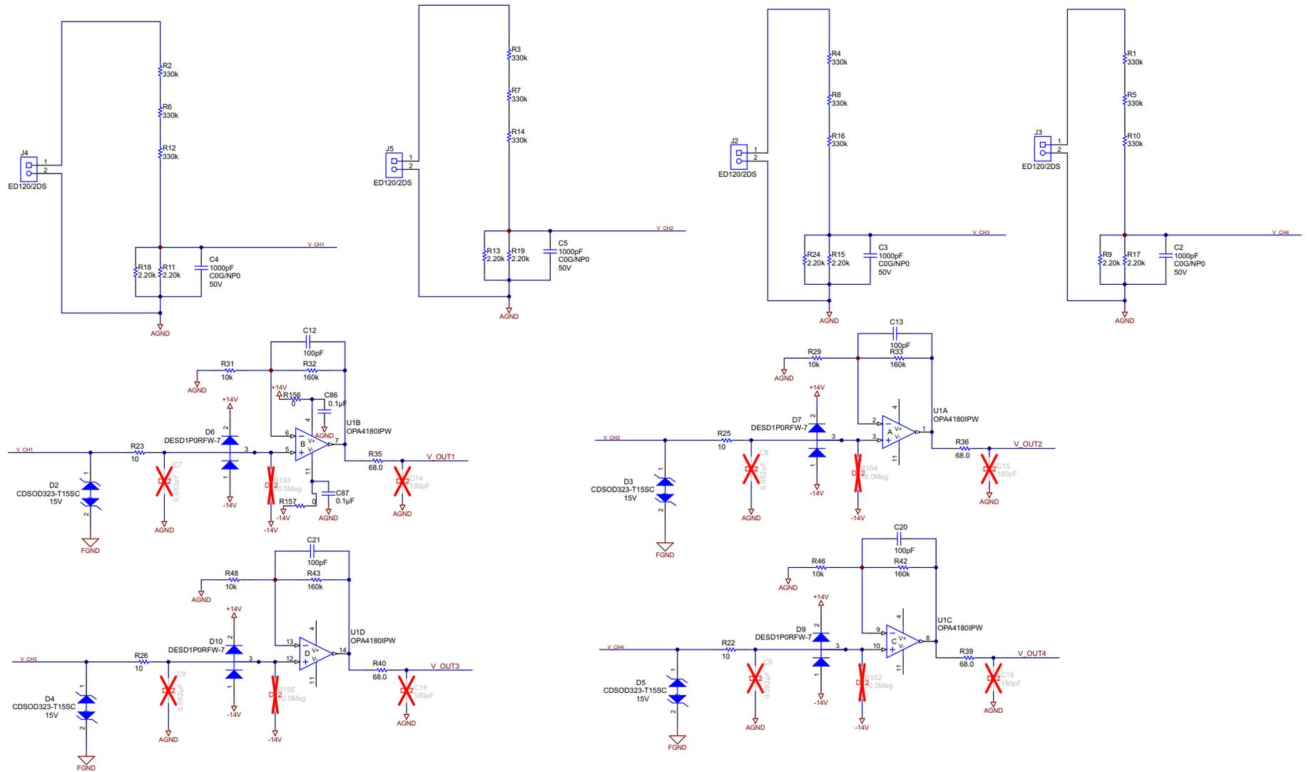
Figure 31. 350-V AC Voltage Input Measurement
