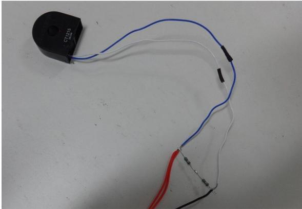
Figure 19. Voltage Output Current Transformer
