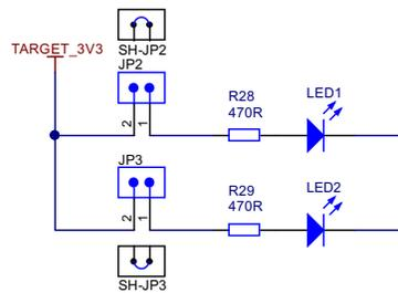
**Figure 9. Jumpers JP2 and JP3 Connect Onboard LED**
