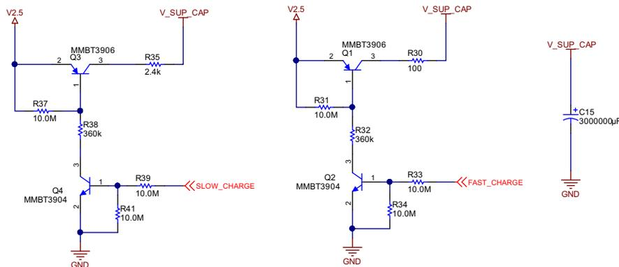
Figure 19. Resistive Charging Circuit for Super Capacitor
