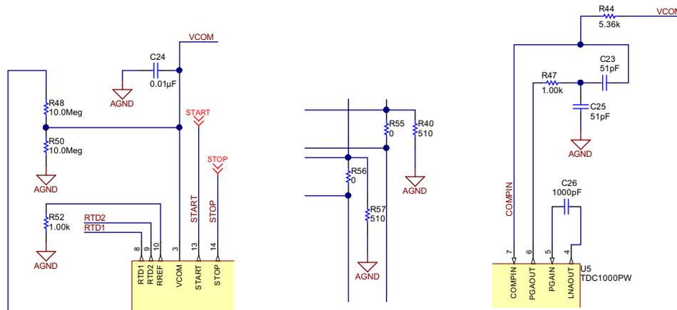
Figure 22. Critical External Passive Circuits of TDC1000
