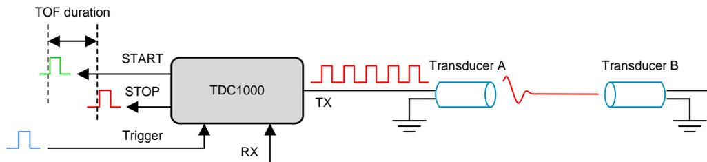
**Figure 2. Time of Flight Measurement**
