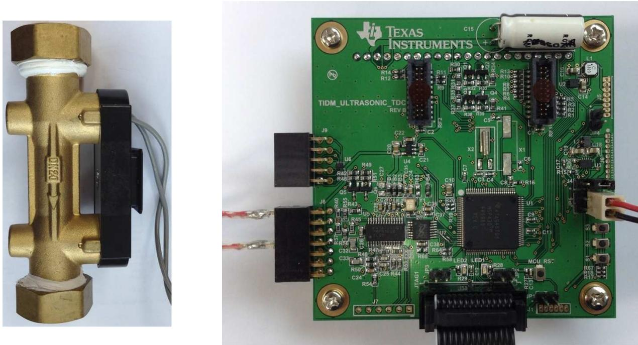
**Figure 30. System Setup to Measure Accuracy of Differential Time of Flight**
