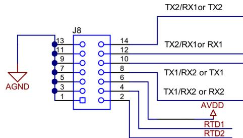
**Figure 8. Socket (J8) Connecting Transmitting and Receiving Pins of TDC1000**
