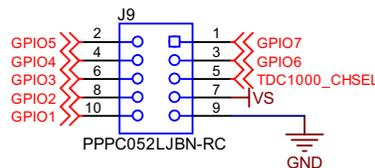
Figure 7. Socket (J9) Connecting to I/O of MCU
