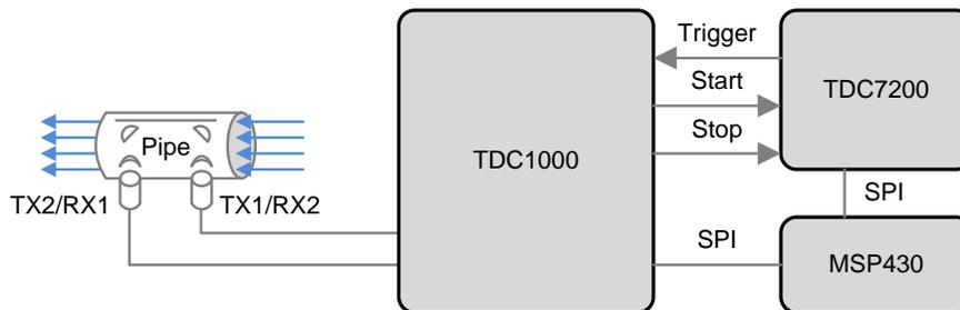
**Figure 1. Measurement Front End**
