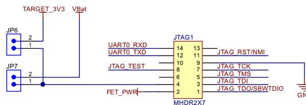
**Figure 11. JTAG Interface for MSP430 FET Tool to Program MCU**
