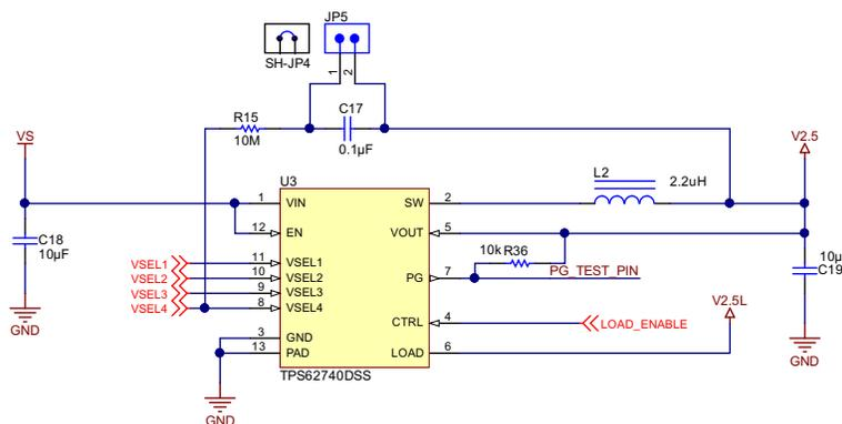
Figure 17. Buck Converter Using TPS62740 to Provide  $V_{CC}$  to the System
