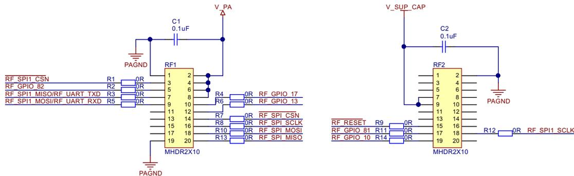
**Figure 20. Socket for Connection of Communication Module (Wired or Wireless Type)**
