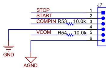
**Figure 10. Test Pins of TDC1000**
