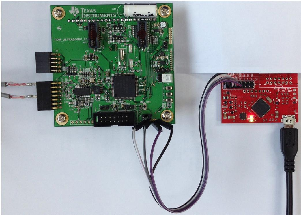
**Figure 31. System Setup to Measure of Current Consumption**
