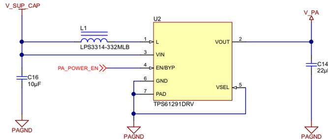
Figure 18. Boost Converter With Super Capacitor (in [Part 13](#))
