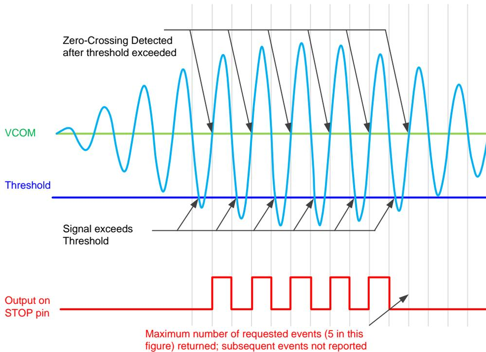
**Figure 3. Received Signal to Stop Pulses Conversion**
