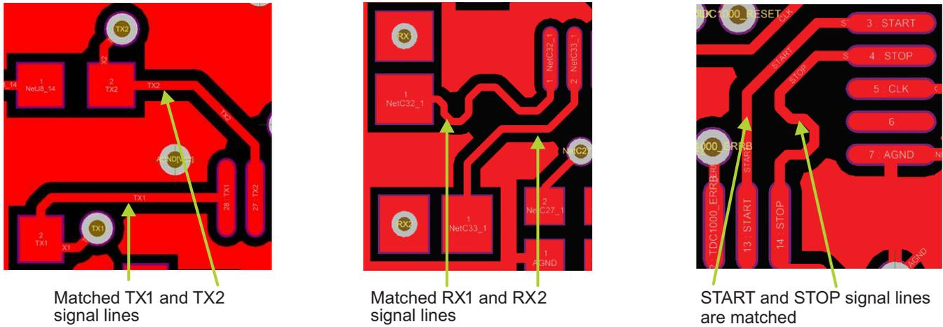
**Figure 23. PCB Layout of Matched Signal Lines**
