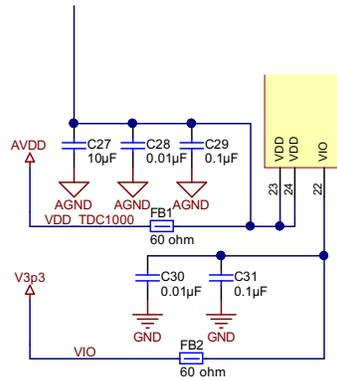
Figure 21. Low-Pass Filters for Power Supplies of TDC1000
