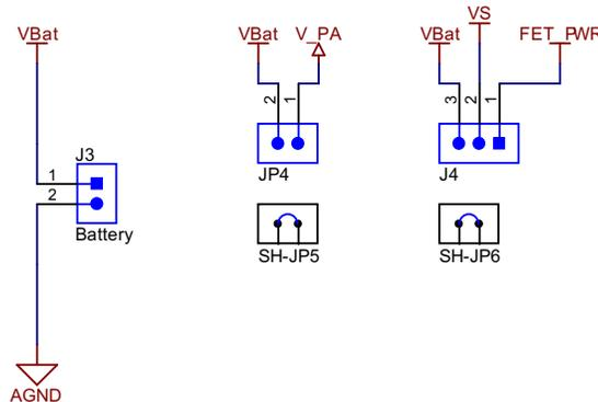
Figure 16. Battery Connector Using 3.6-V Lithium Battery
