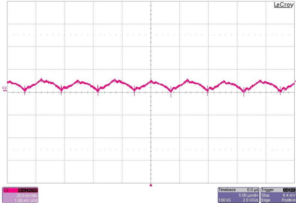
The 13.2V output ripple voltage (AC coupled) is shown in the figure below. The image was taken with the output loaded to 3A. The input voltage is set to 6V. (20mV/DIV, 5uS/DIV)
