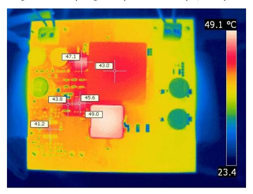
A thermal image is shown below operating at 12V input and 13.2V@4A output (room temp, no airflow).
