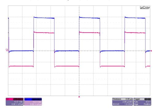
The photo below shows the two switching node voltages for an input voltage of 6V and a 3A load. Blue is the bottom FET (TP7) and Red is the top FET (TP3). (10V/DIV, 2uS/DIV)
