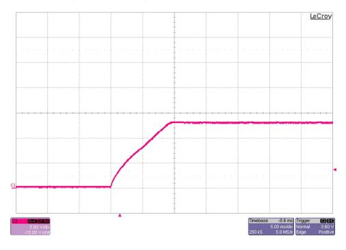
The photo below shows the output voltage startup waveform after the application of 6V in. The 13.2V output was loaded to 3A. (5V/DIV, 5mS/DIV)
