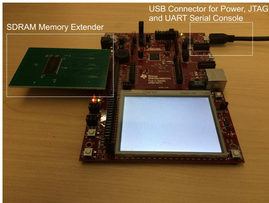
**Figure 4. Full Test Assembly**
