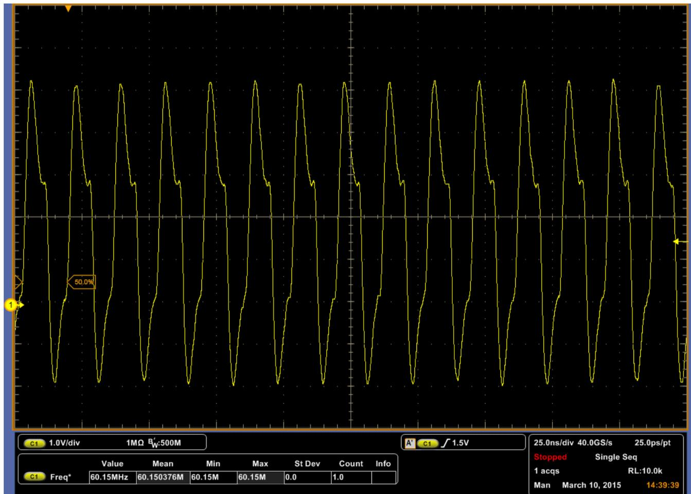
**Figure 8. SDRAM Clock Signal Integrity**
