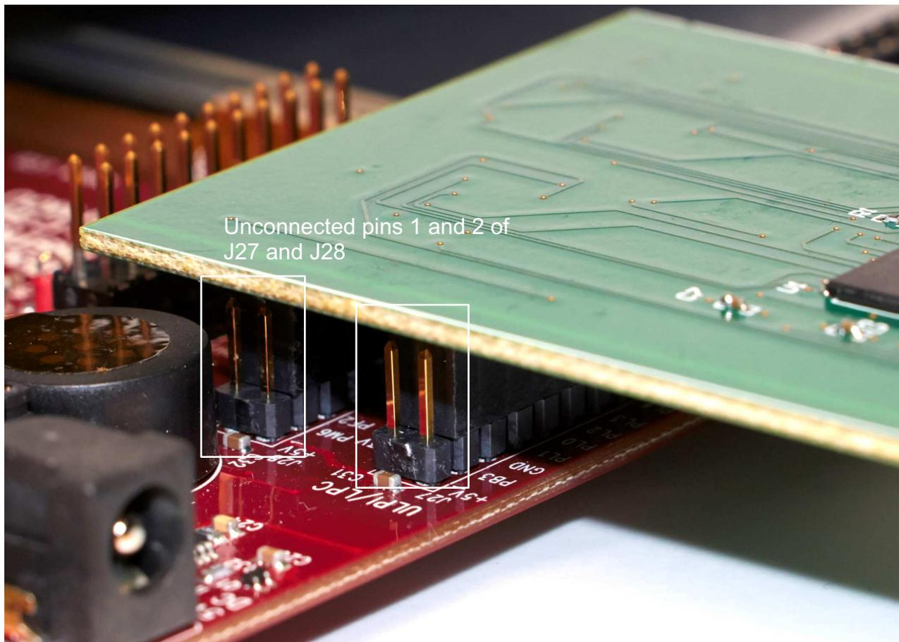
**Figure 3. SDRAM Connector Mounting**
