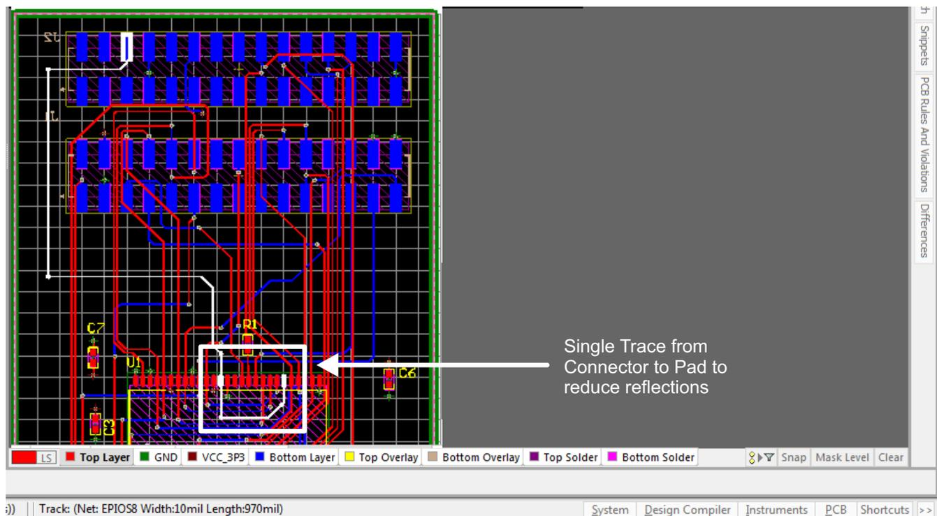
**Figure 9. Layout Guidelines for Reducing Reflections**
