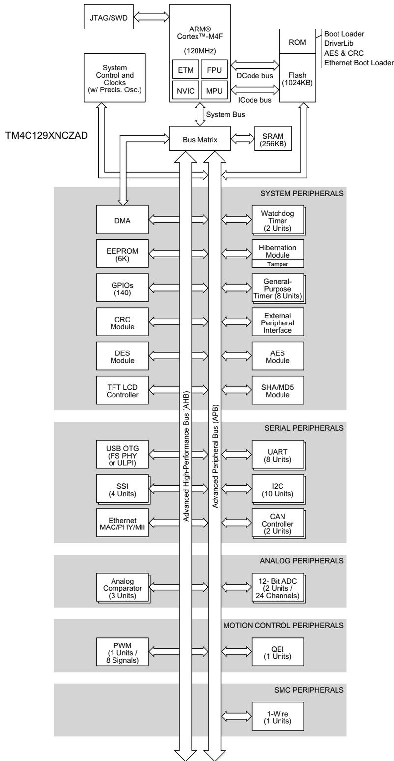
Figure 1. TM4C129XNCZAD Microcontroller High-Level Block Diagram
