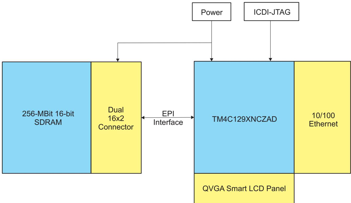
Figure 2. SDRAM Extender Block Diagram
