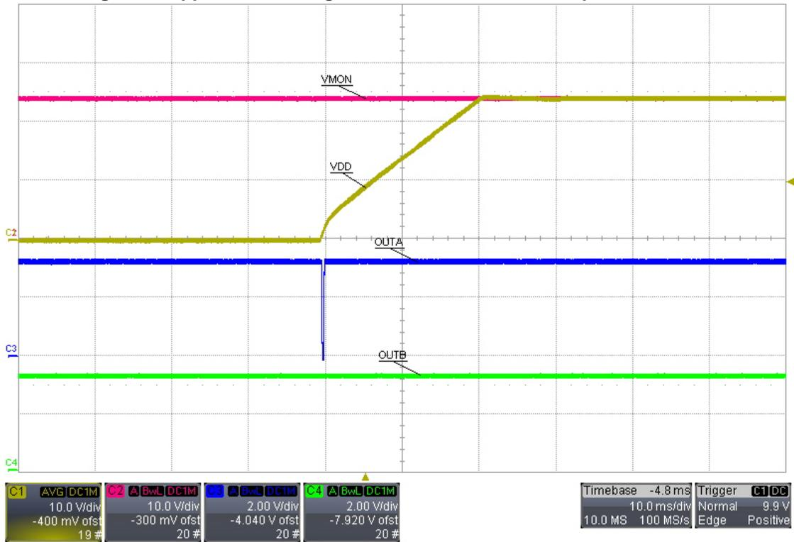
Figure 7: Startup with  $V_{DD}$ ,  $V_{MON}$  Independent,  $V_{PULLUP} = 3.3$
