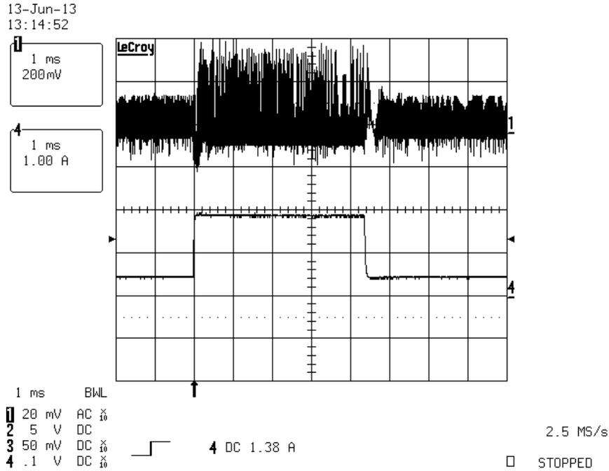
The lower is a .5 to 2 amp current load step and the upper is the voltage output response
