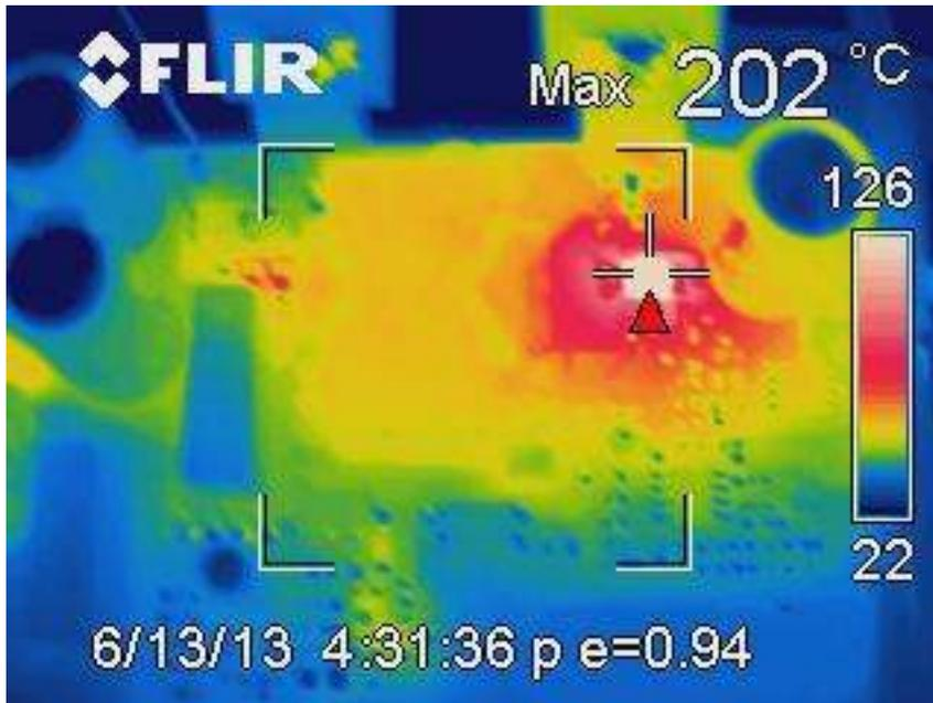
Image taken at full load in still air at 24 deg C. the hottest part on the board is the load current sense R at 202 deg C. **Customer should consider a smaller value to reduce this power dissipation (  $2^2 \cdot 24 = .96$  watts)**
