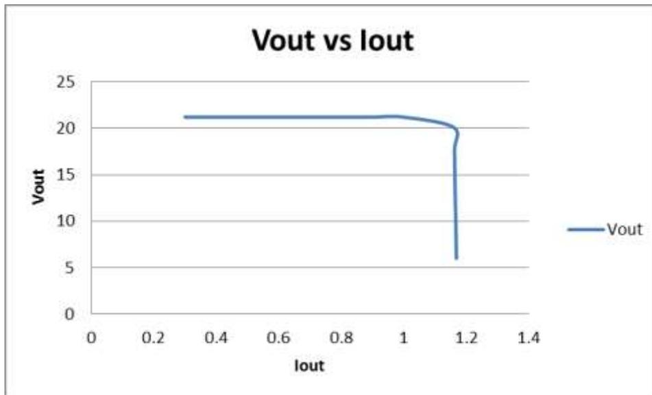
V vs I for an output current limit selected at about 1 amp
