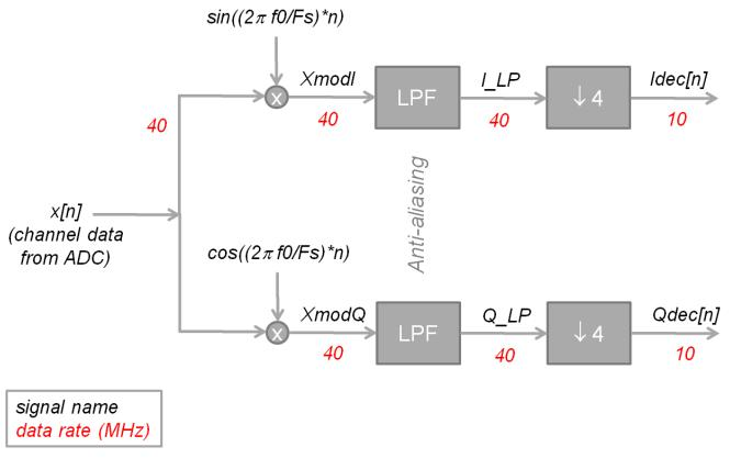
Figure 5. Envelope Detector Block Diagram
