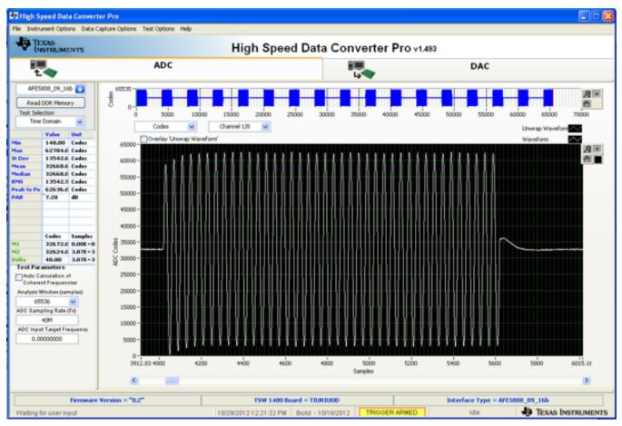
Figure 24. Sine Burst Waveform at Frequency of 5 MHz (Fs/8, where Fs=40MSPS)
