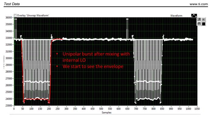
Figure 25. AFE5809 LVDS Output for Sine Burst After I/Q Demodulation at Fs/8 and Decimation of 4
