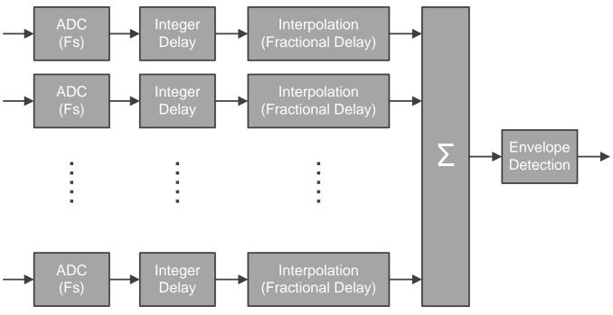
Figure 4. Conventional Time-Delay Beamformer Block Diagram
