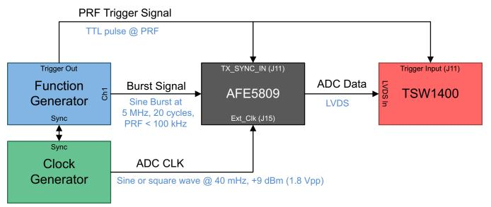
Figure 17. Block Diagram of Envelope Detection
