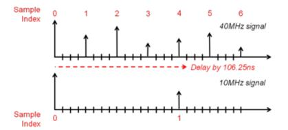
Figure 7. Schematic Comparison of Delaying 40-MHz and 10-MHz Signals
