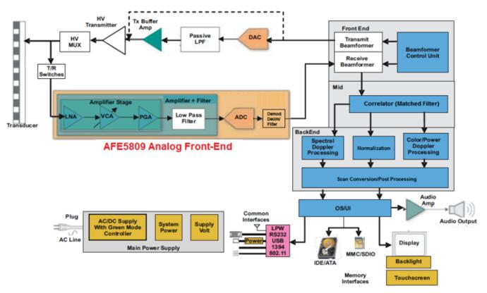
Figure 13. AFE5809 in SONAR System
