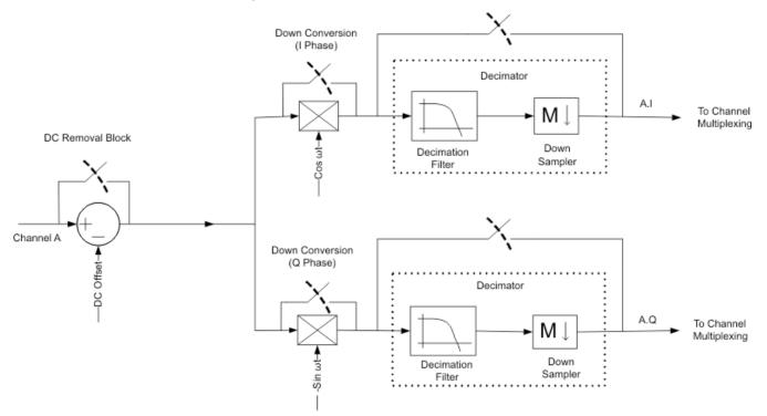
Figure 20. Signal Chain of Demodulator Sub-Blocks
