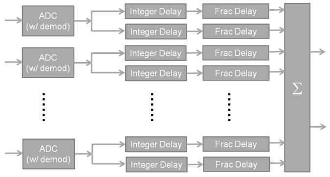
Figure 6. Time-Delay Beamformer for Demodulated Channel Data [2]
