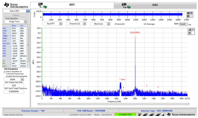
Figure 23. FFT 200-kHz Signal Sampled at 20 MSPS With Decimation = 32
