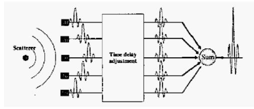
Figure 1. Principle of Delay-and-Sum Beamforming [2]
