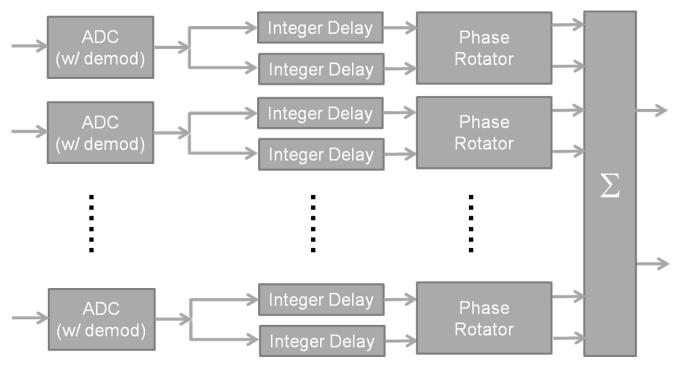
Figure 11. Demodulation Before Beamformer with Phase Rotation
