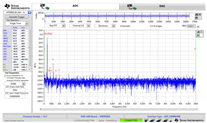
Figure 22. FFT 200-kHz Signal at 20 MSPS With No Decimation
