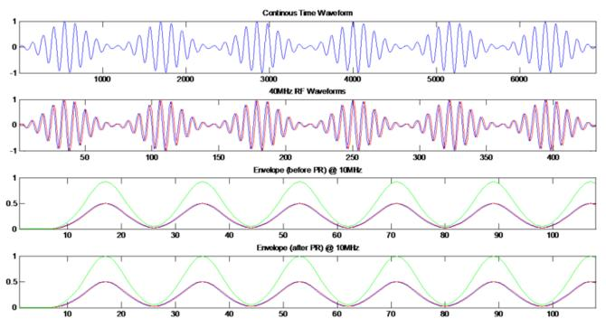
Figure 9. Delaying an Envelope Signal Using Phase Rotation
