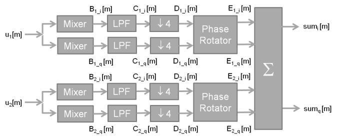
Figure 8. Block Diagram for Phase Rotator Functionality Verification
