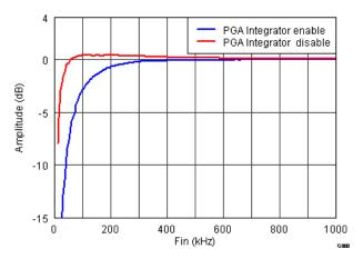
Figure 19. Signal Chain Low Frequency Response With INM Capacitor = 1 µF
