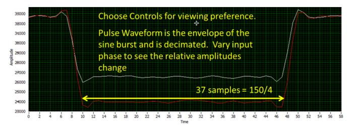
Figure 27. Separated Data After Receiver Processing Shows Decimated Envelope
