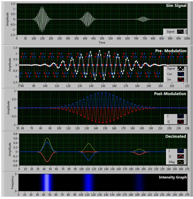
Figure 14. Simulation of AFE5809 Demodulated and Decimated Echo Train
