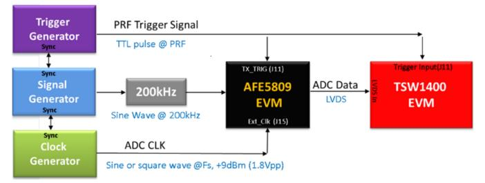
Figure 15. Block Diagram of Sonar Setup
