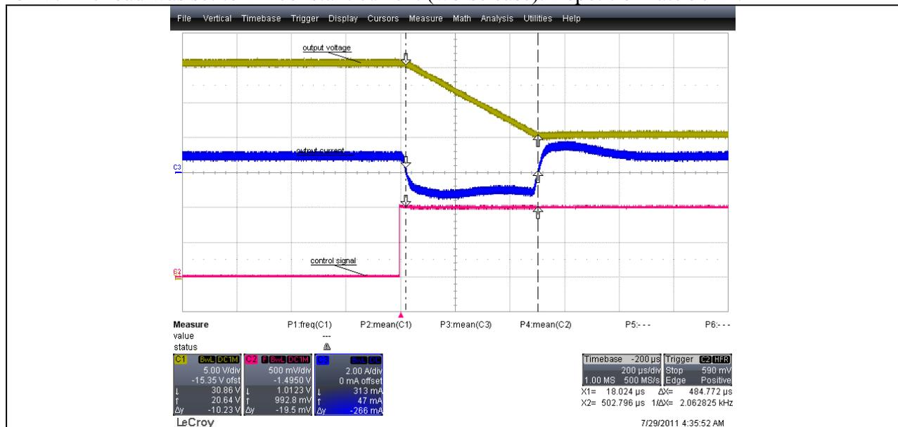
**Load = 1A, 32Vout to 20Vout (maximal down slope limited internally to 500us)**
