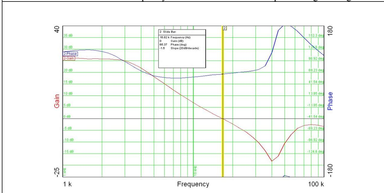
Frequency loop response of the converter – 200uF capacitive load
