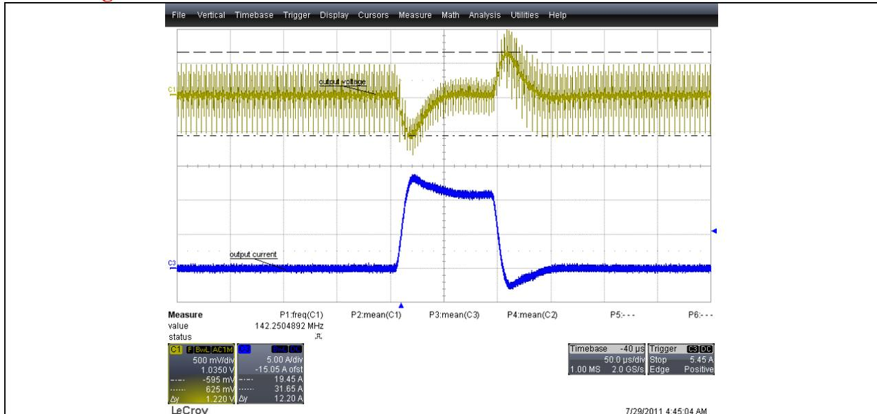
Yellow – Output voltage AC coupled 200MHz band with – 1.2V
