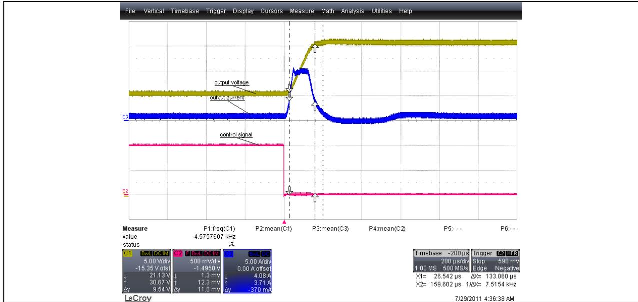
**Load = 1A, 20Vout to 32Vout (maximal up slope limited internally ~ 100us)**
