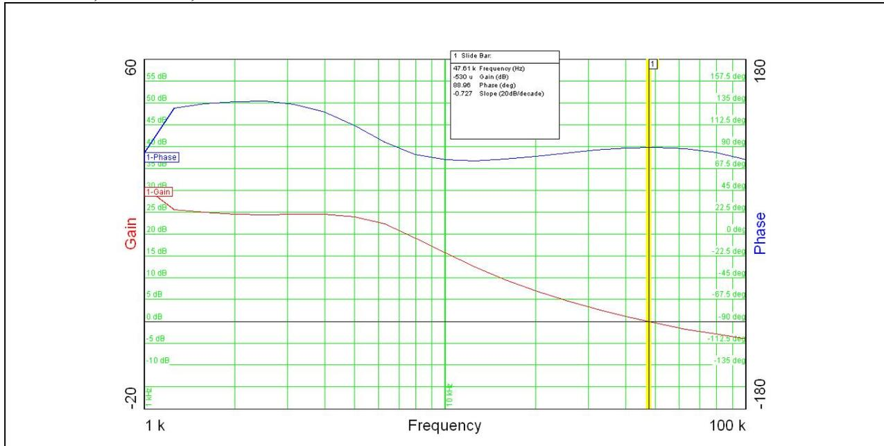
Frequency loop response of the converter – no capacitive load
