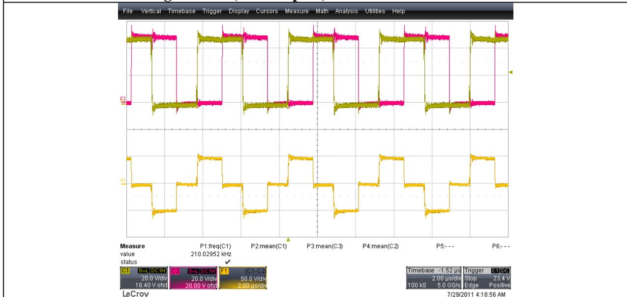
The same, in addition CH1-CH2 (Voltage across the transformer)
