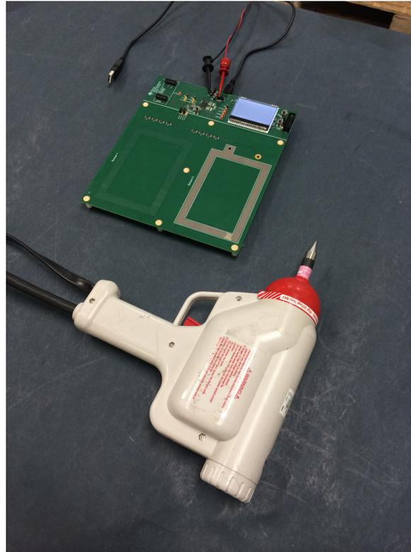
**Figure 19. ESD Test Setup**
