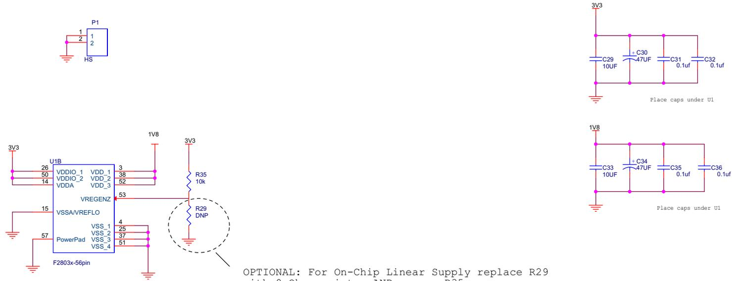
OPTIONAL: For On-Chip Linear Supply replace R29 with 0 Ohm resistor AND remove R35.
