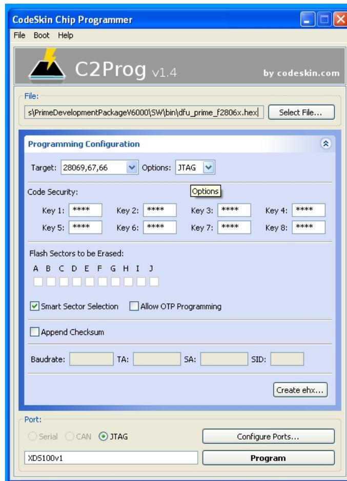
Figure 2. Selecting PLC-Lite Binary to be Flashed (through XDS100)
