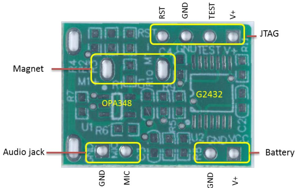
Figure 4. PCB Layout
