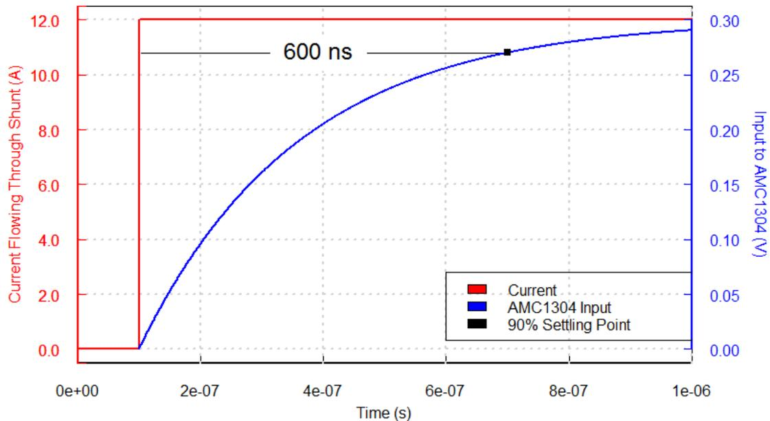
Figure 12. Typical Step Response of RC Passive Filter
