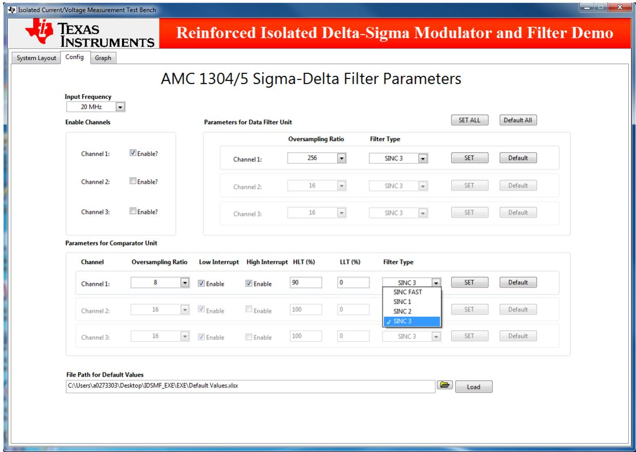
Figure 41. GUI - Comparator Unit Filter Selection - Config Tab
