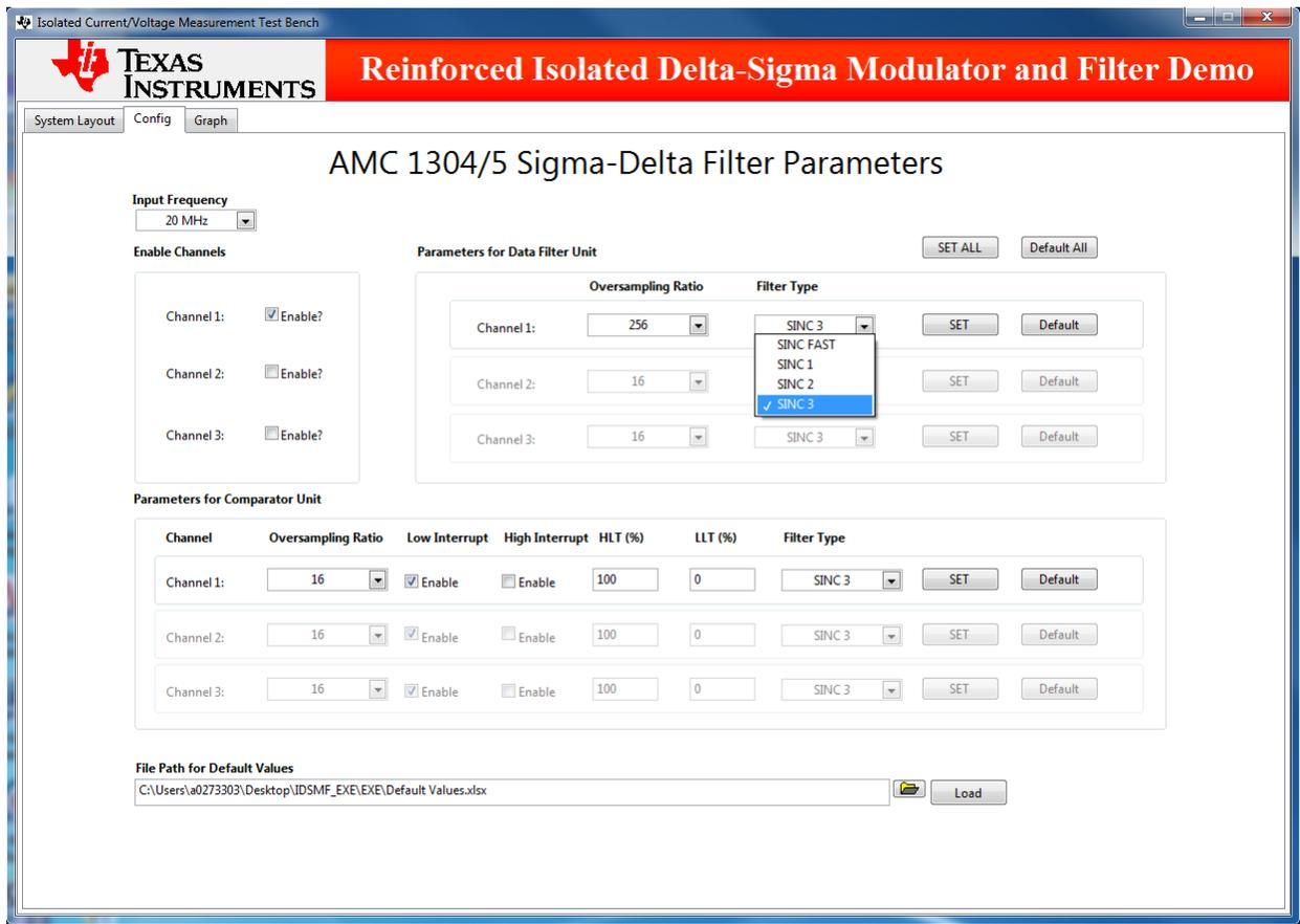
Figure 38. GUI - Data Path Filter Selection - Config Tab
