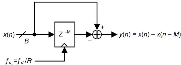
**Figure 9. CIC Comb Filter Section**
