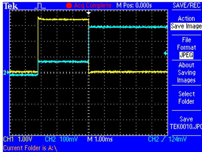
Figure 32. Response of GPIO-00 to Over-current Event
