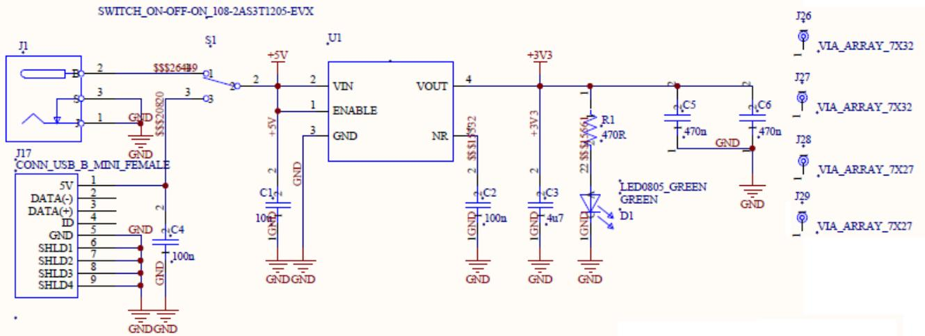
Figure 53. Schematic for Docking Station - Part 2
