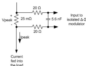
Figure 13. RC Passive Filter Selected
