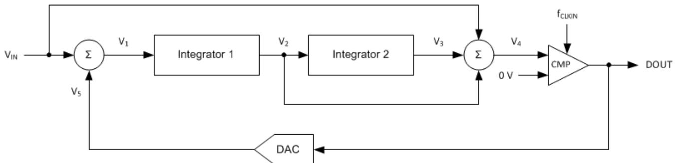
**Figure 5. Block Diagram of a Second-Order  $\Delta\Sigma$  Modulator**
