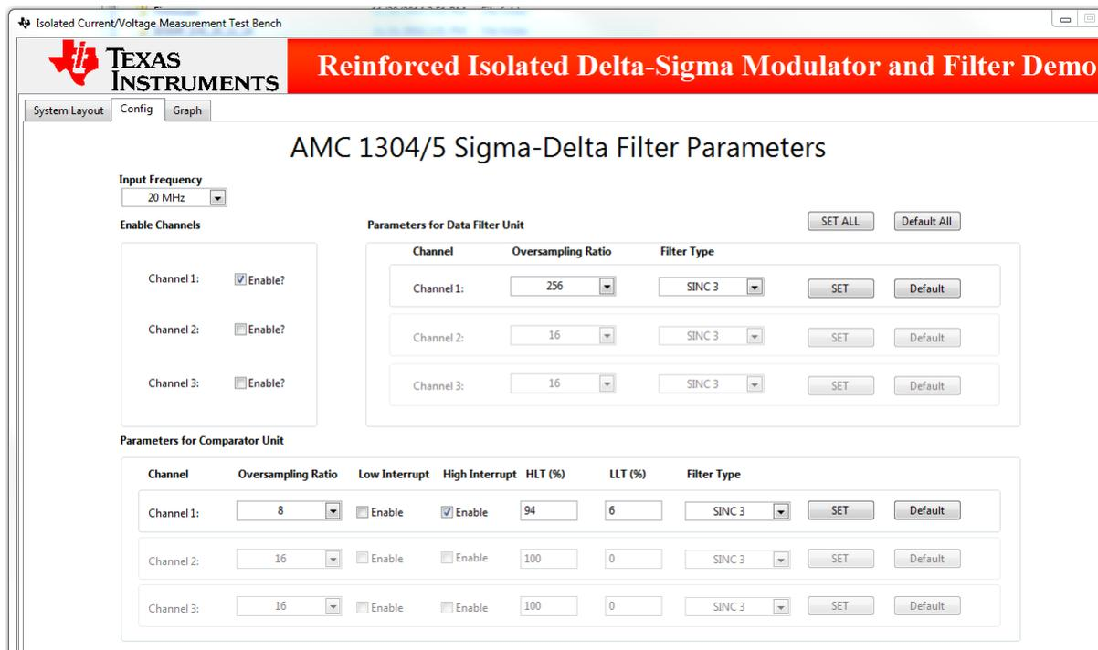
**Figure 31. Threshold Settings for Over-current Detection**
