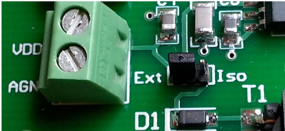
**Figure 49. Jumper Setting for External Supply to AMC1304M25**
