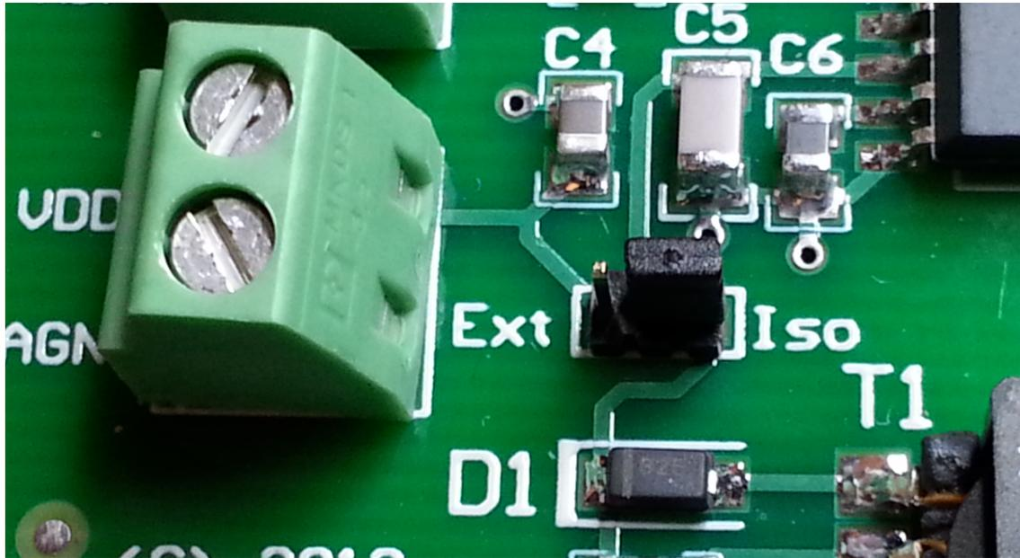
Figure 23. High Side of AMC1304 Supplied from T1
