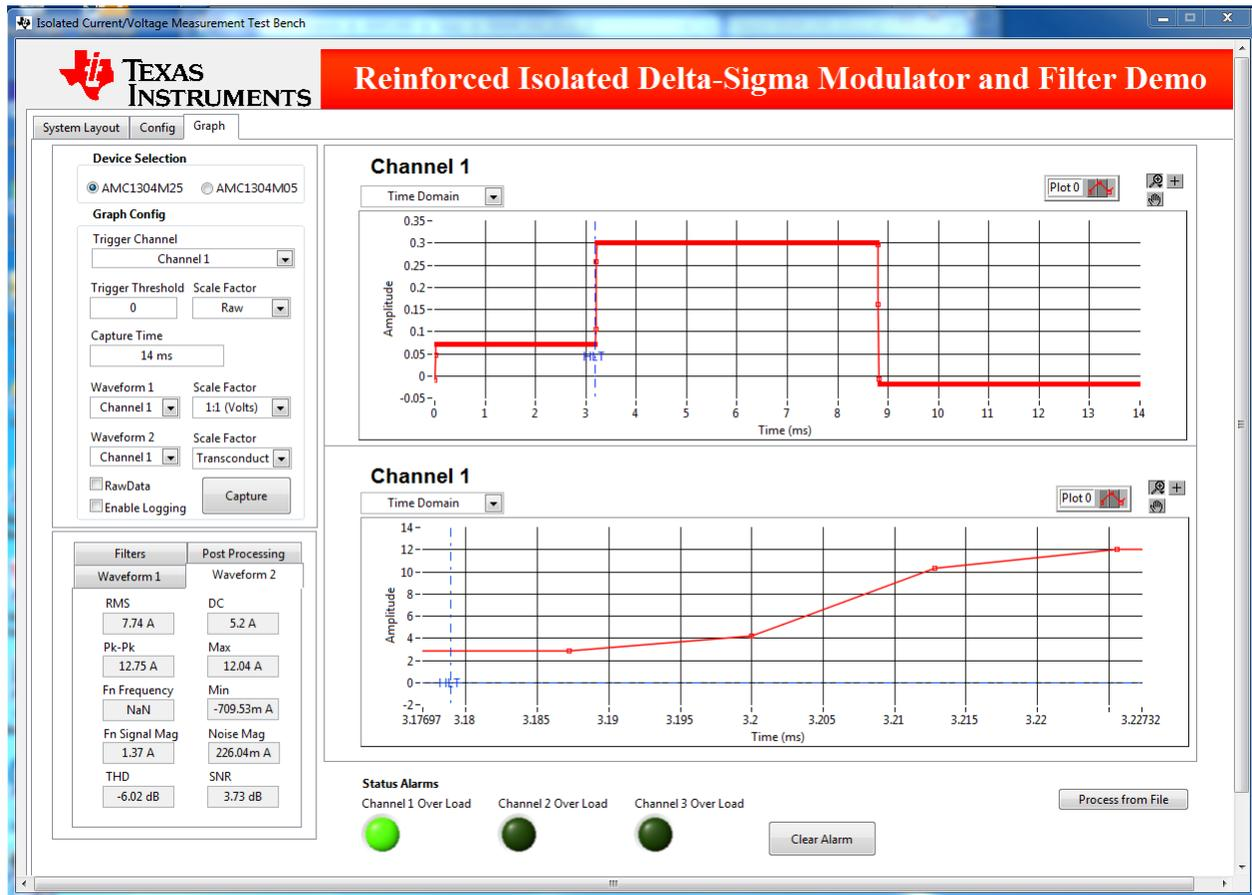
Figure 34. GUI Indicator of Comparator Threshold Crossing
