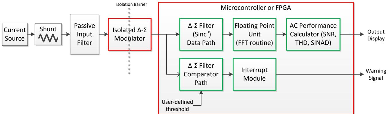
Figure 2. Data Acquisition System Using Isolated Delta-Sigma Modulator
