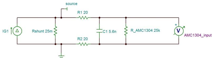
Figure 19. TINA-TI™ Schematic - Input Passive Filter
