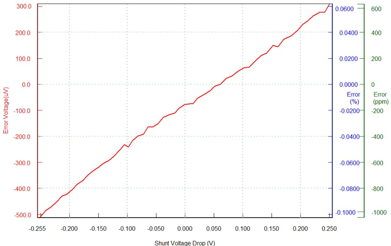
Figure 28. Measured Uncalibrated System Error
