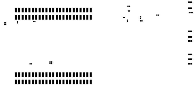
Figure 30. Secondary Side Solder Stencil
