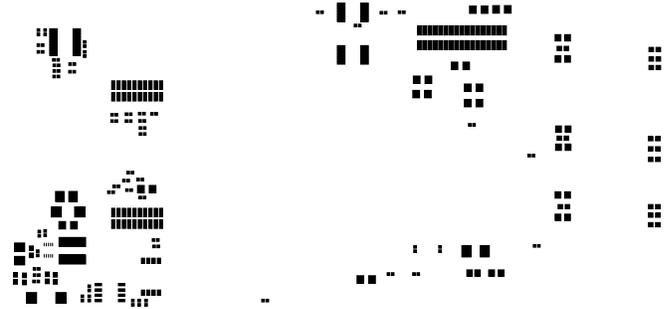
Figure 28. Primary Side Solder Stencil
