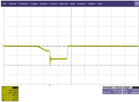
Figure 23. CH1: Maximum Voltage Across 12 V Output Diode
