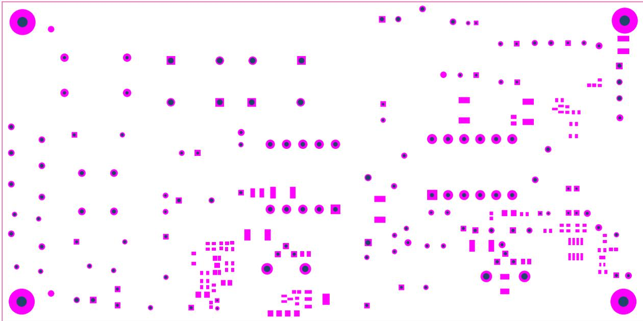
Figure 40. Bottom Solder Mask
