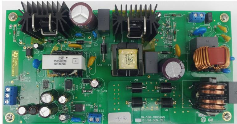
Figure 1. 30-W Ultra-Wide Range Power Supply for Protection Relay
