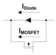
Figure 6 – MOSFET and diode in parallel.
