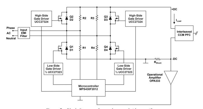
Figure 7 – Block diagram of a synchronous bridge rectifier.
