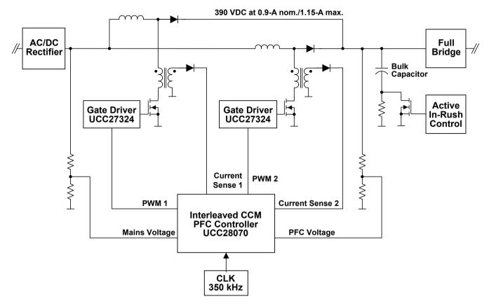
Figure 12 – Block diagram of the interleaved PFC.
