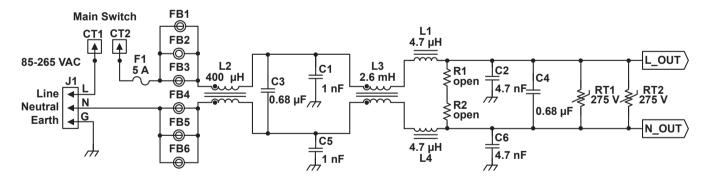
*Figure 3 – Input EMI filter.*
