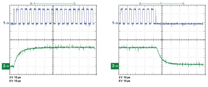
Figure 9 – Ramp-up and ramp-down of the gate-source voltage, 10 μs/div.
