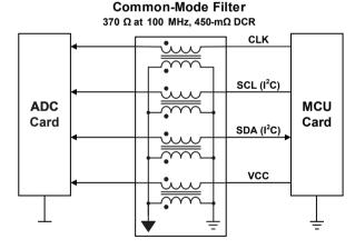
Figure 28 – Common-mode filter on the ADC card.
