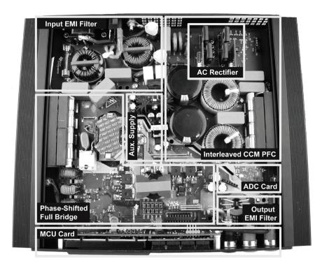
*Figure 37 – Top view of the power supply.*
