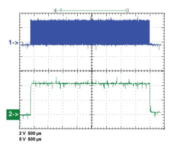
Figure 10 – Gate-source voltage, 500 µs/div.
