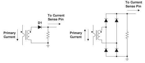
Figure 20 – Unipolar and bipolar current sense.
