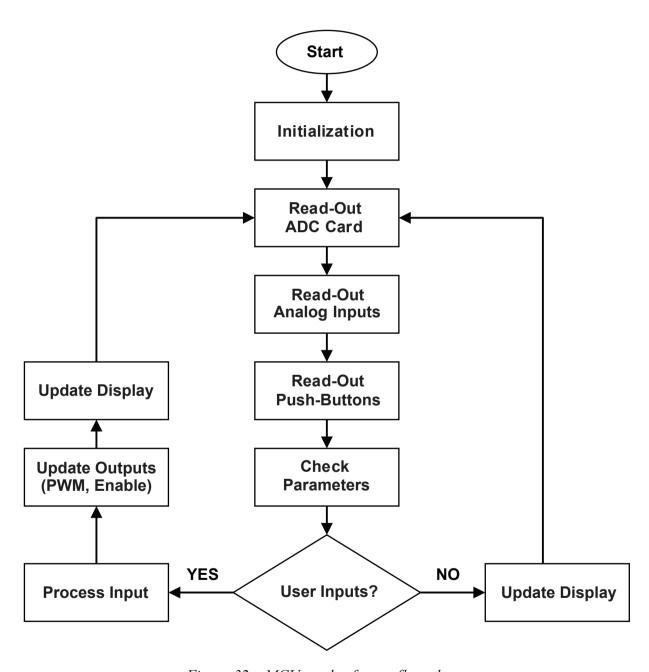
*Figure 32 – MCU card software flow chart.*
