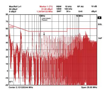
Figure 35 – Conducted emissions at 230-VAC input and 25-A load at 13.8 V.
