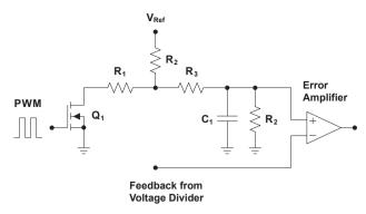
Figure 30 – Modulation of the reference voltage for an error amplifier by a PWM signal.
