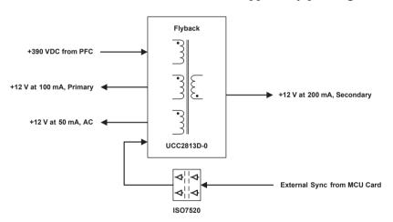
Figure 25 – Auxiliary power supply.
