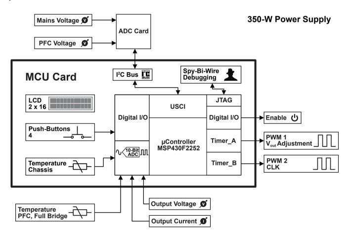
Figure 29 – Block diagram of the MCU card.
