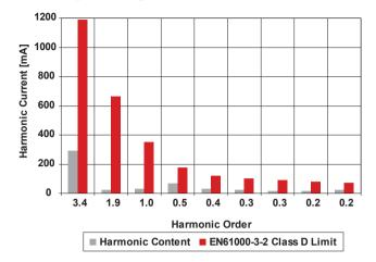
Figure 14 – Harmonic content according to EN61000-3-2.
