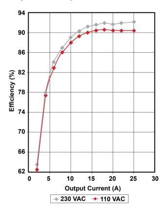
Figure 33 – Plug-to-plug efficiency at 13.8-V output voltage.
