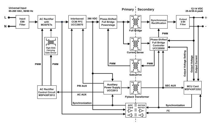
Figure 36 – Detailed block diagram of the system.
