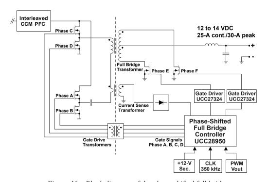
Figure 16 – Block diagram of the phase-shifted full bridge.
