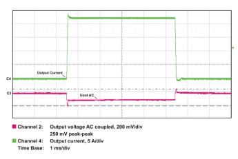
Figure 24 – Load step from 2 to 90 percent load.
