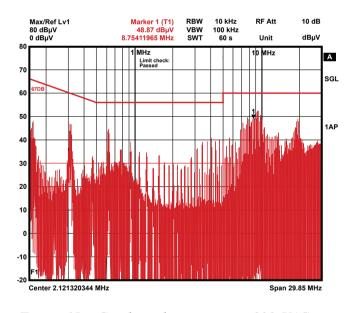
Figure 15 – Conducted emissions at 230-VAC input and 0.9-A load at 390 V.
