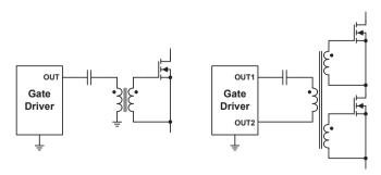
Figure 17 – Single- and double-side-ended gate-drive transformer.
