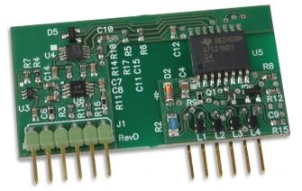
Figure 27 – Photo of the ADC card.
