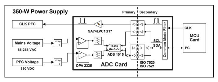
Figure 26 – Block diagram of the ADC card.
