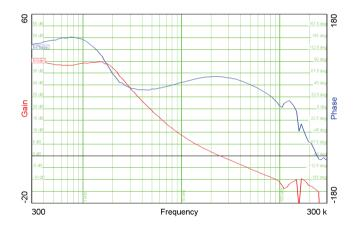
*Figure 23 – Bode plot of the control loop.*
