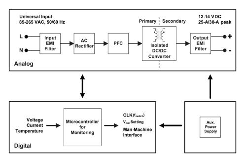
Figure 2 – Simplified system block diagram.
