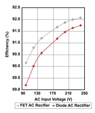
Figure 34 – Efficiency diode bridge rectifier vs. synchronous rectifier.
