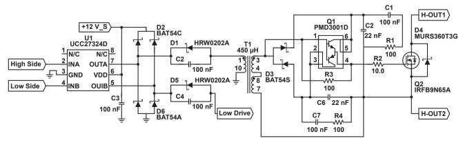
Figure 18 – Gate driver for phase-shifted full bridge.
