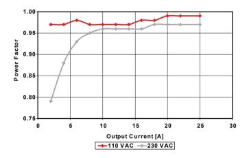
Figure 13 – Power factor of the interleaved PFC at 13.8-V output voltage.
