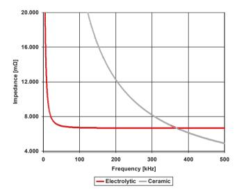
*Figure 22 – Impedance vs. switching frequency.*
