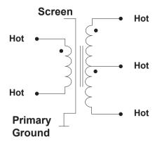
Figure 21 – Transformer with integrated screen.
