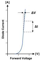
*Figure 5 – Diode forward characteristic.*
