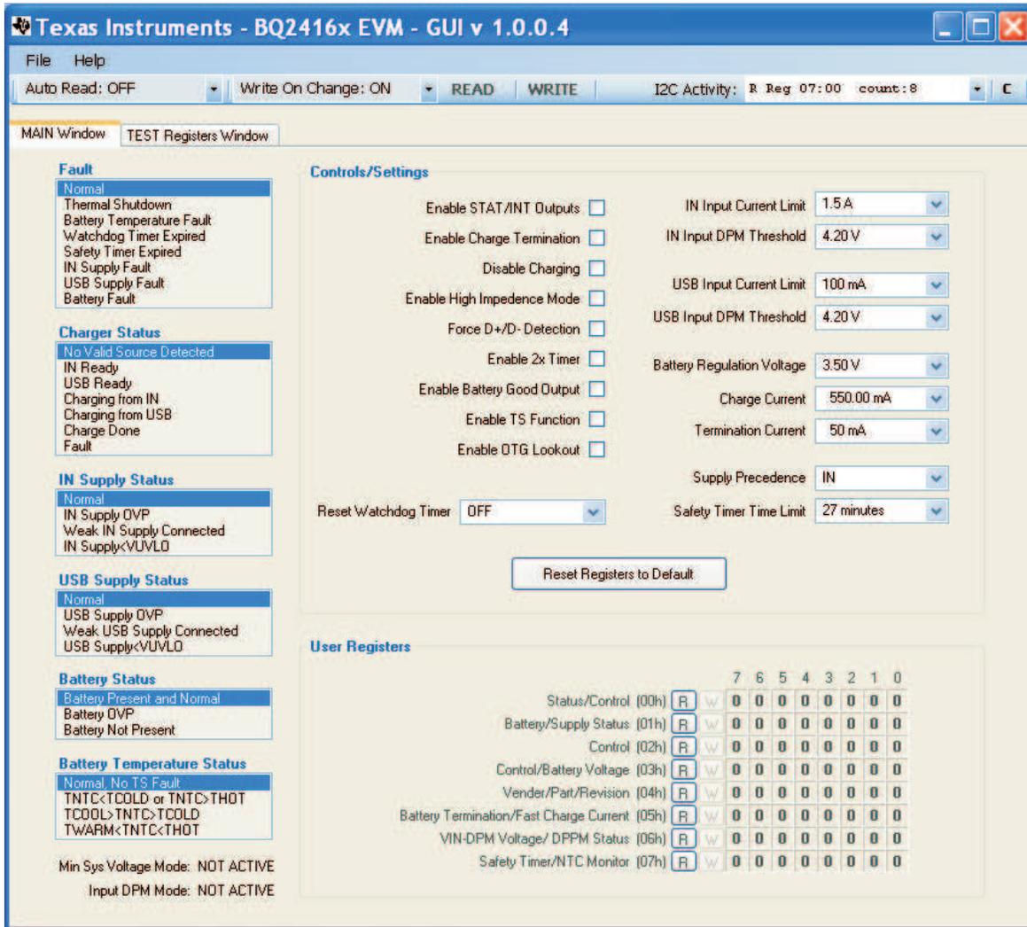
Figure 5. Main Window of bq2416xSW Evaluation Software
