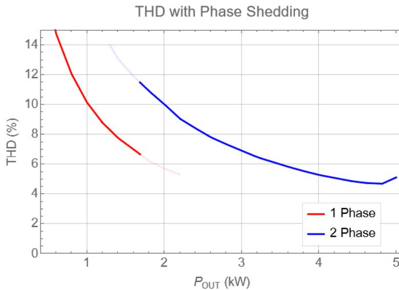
$$V_{IN} = 230 V_{RMS}$$
