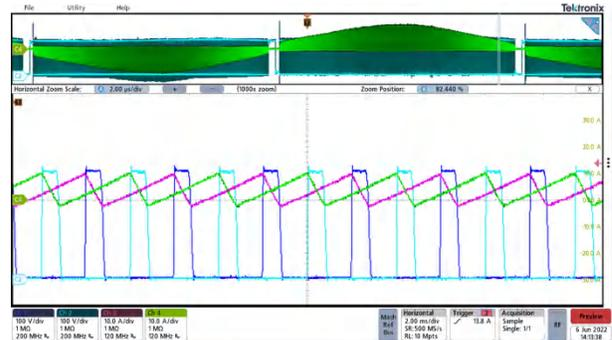
**Figure 3-6.  $V_{IN} < \frac{1}{2} V_{OUT}$**
