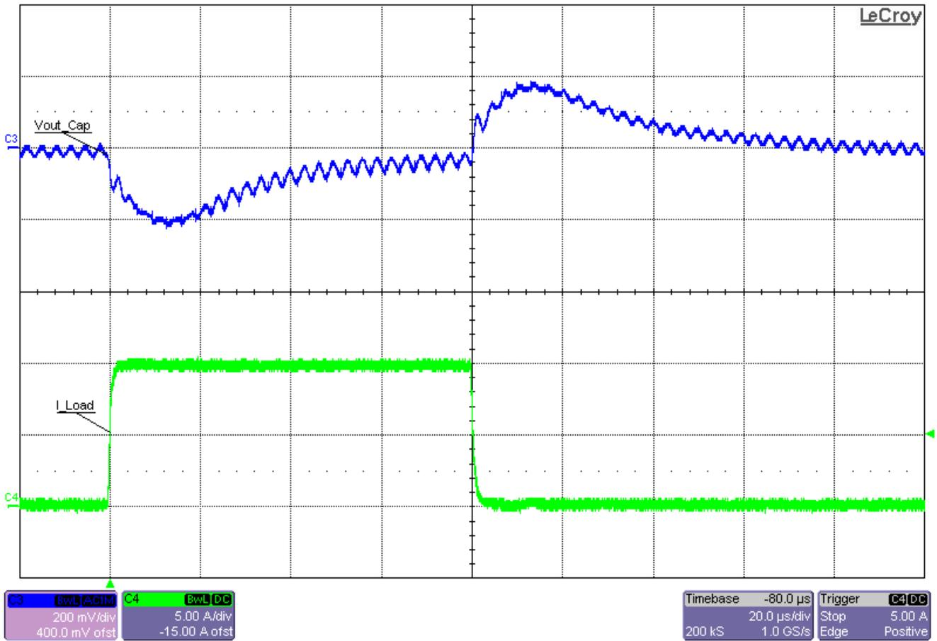
**Figure 3-4. Load Transient Test on 12-V Output Synchronous Buck**
