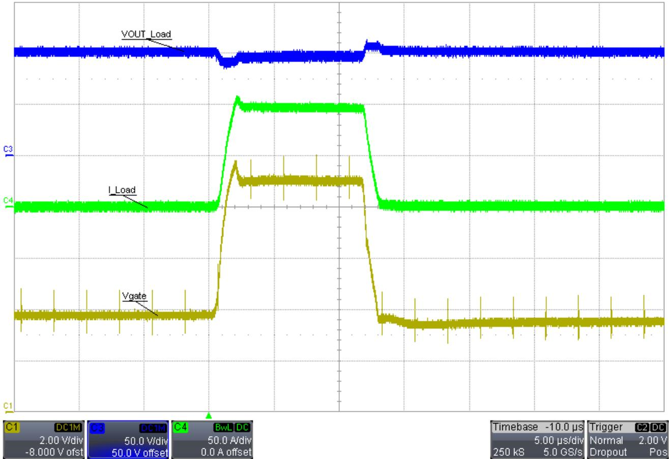
Figure 3-17. PSMN035-150B 100-V Output, 1-A to 100-A Load Transient
