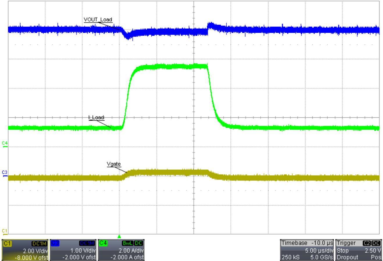
Figure 3-19. Minimum 11- $\mu\text{s}$  High-Level Pulse Width
