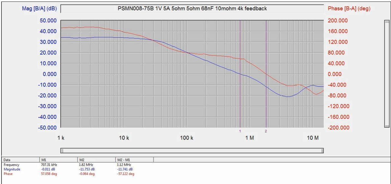
**Figure 3-29. PSMN008-75B, 125-A Variant, 1-V, 5-A**
