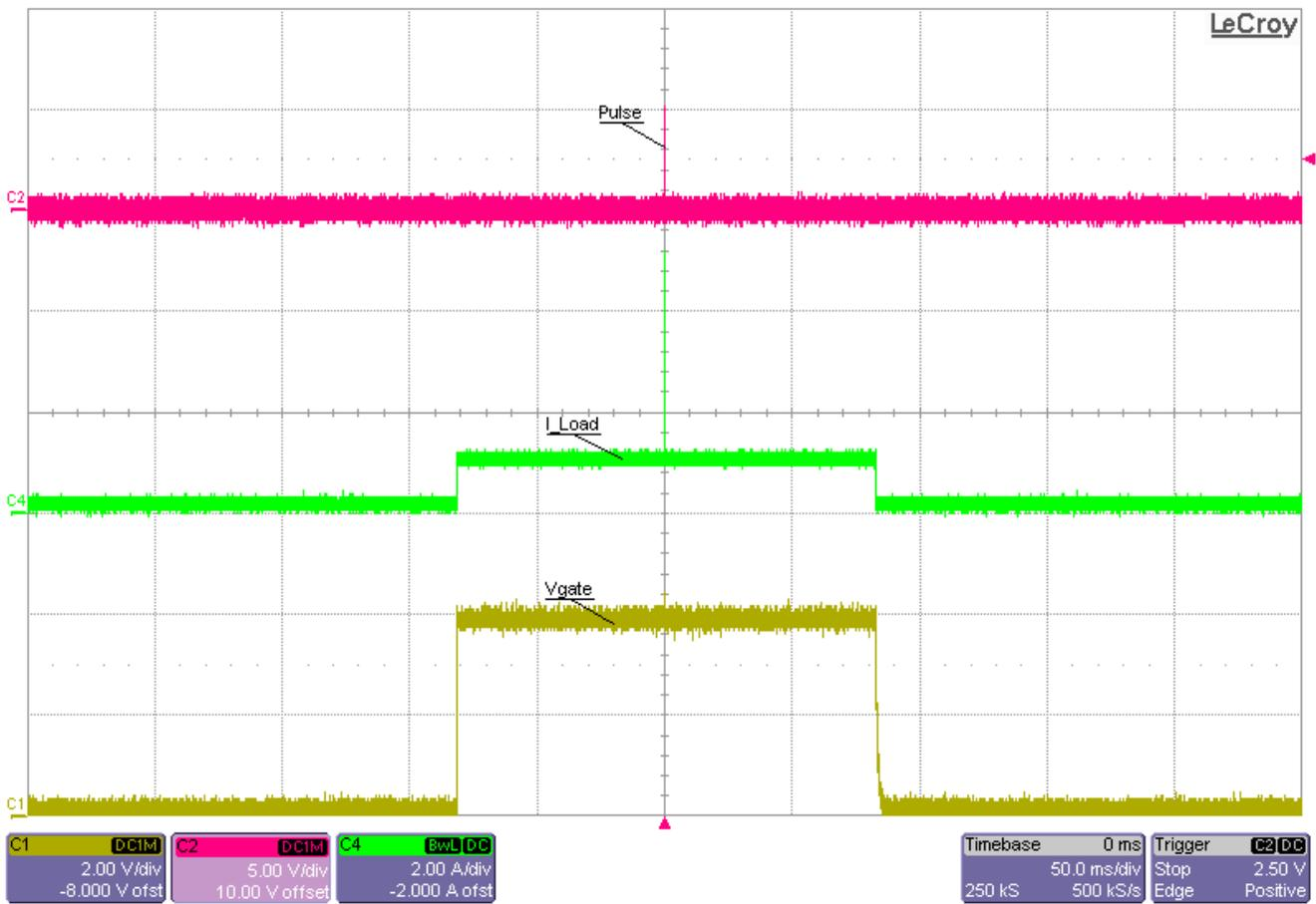
Figure 3-22. Maximum Delay and Maximum Period 160 ms
