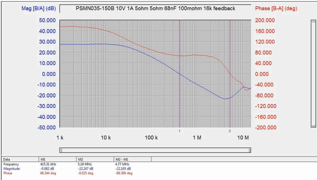
Figure 3-26. PSMN035-150B, 25-A Variant, 10-V, 1-A
