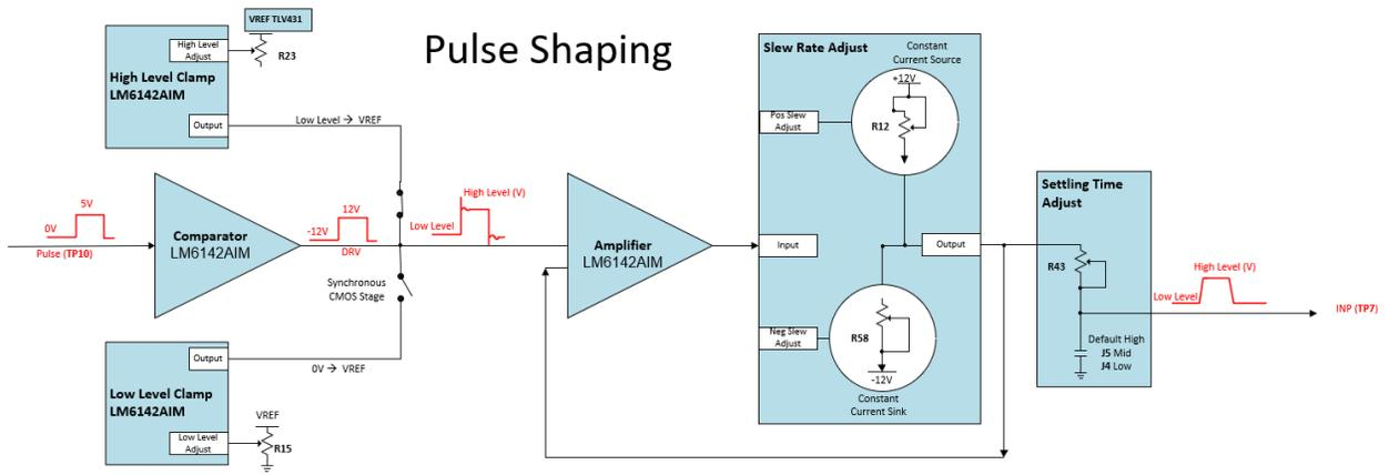
Figure 2-4. Pulse Shaping
