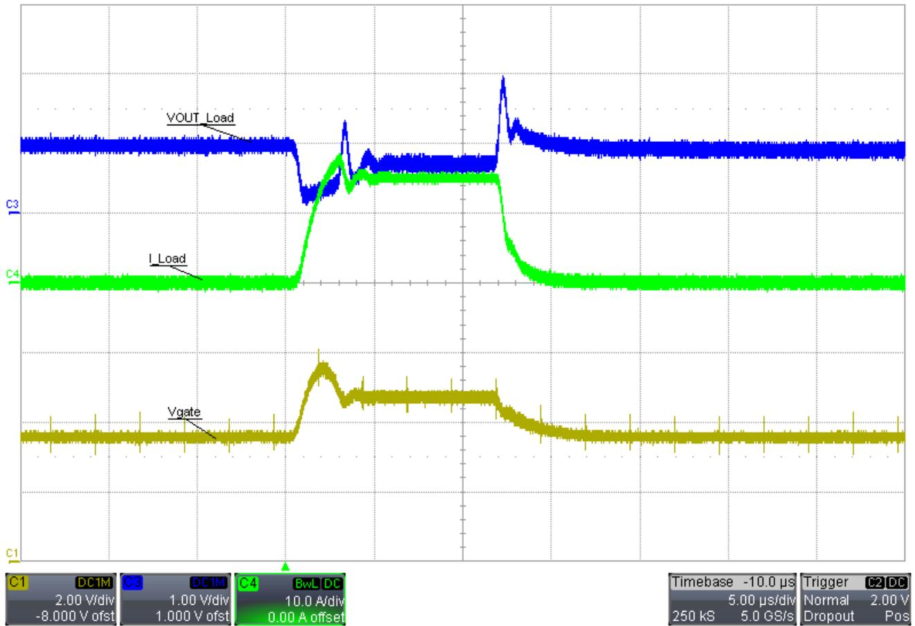
Figure 5-2. Wiring Inductance Voltage Drop 1 A to 15 A, 1-V Output Load Transient
