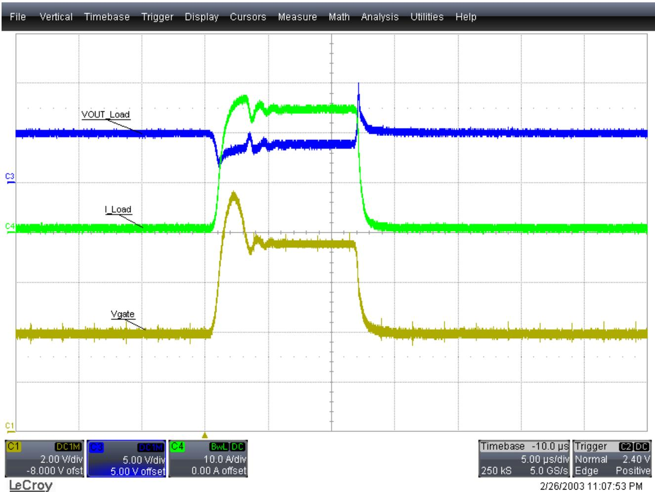
Figure 5-3. 1 A to 25 A, 5-V Output Load Transient
