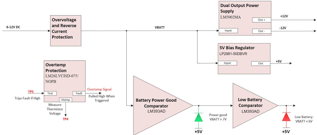
Figure 2-2. Power Supply and Protection
