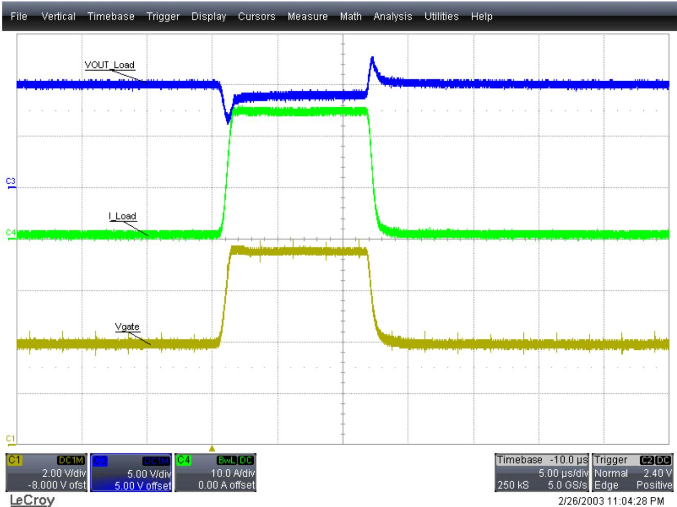
Figure 5-4. 1-A to 25-A, 10-V Output Load Transient
