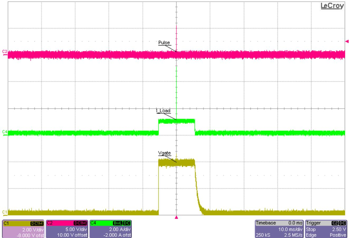
Figure 3-21. Minimum Delay and Minimum Period 11 ms
