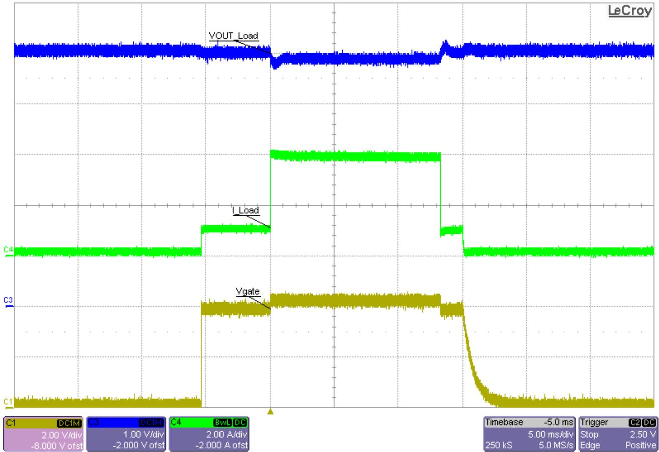
Figure 3-20. Maximum 13-ms High-Level Pulse Width
