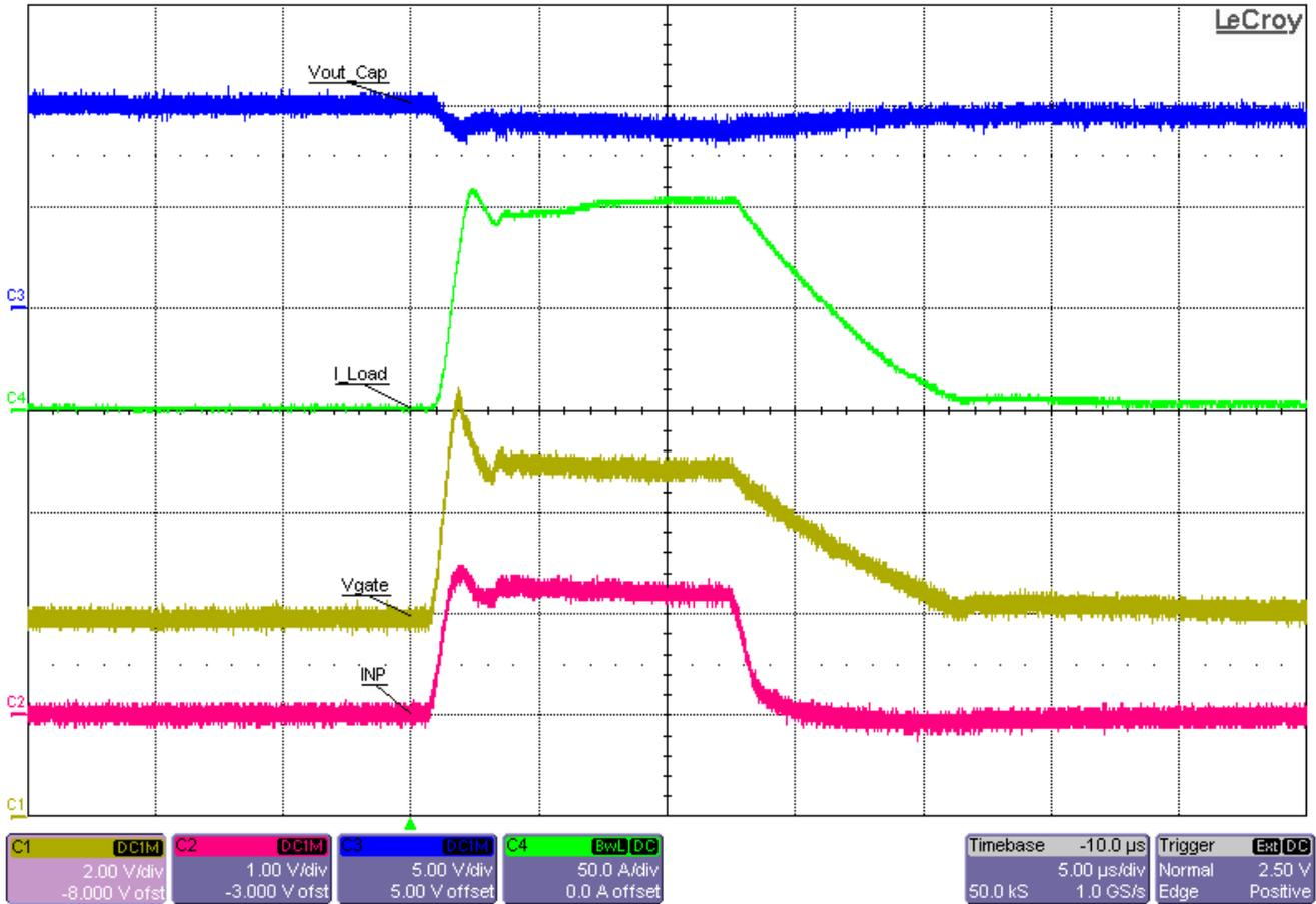
Figure 6-1. 1-A to 100-A Step, 10-V Output, Maximum Slew Rate, Damaged U4
