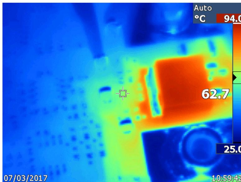
**Figure 3-12. LM26LVCISD-075, PSMN008-75B Load Step Board Thermal Recovery**
