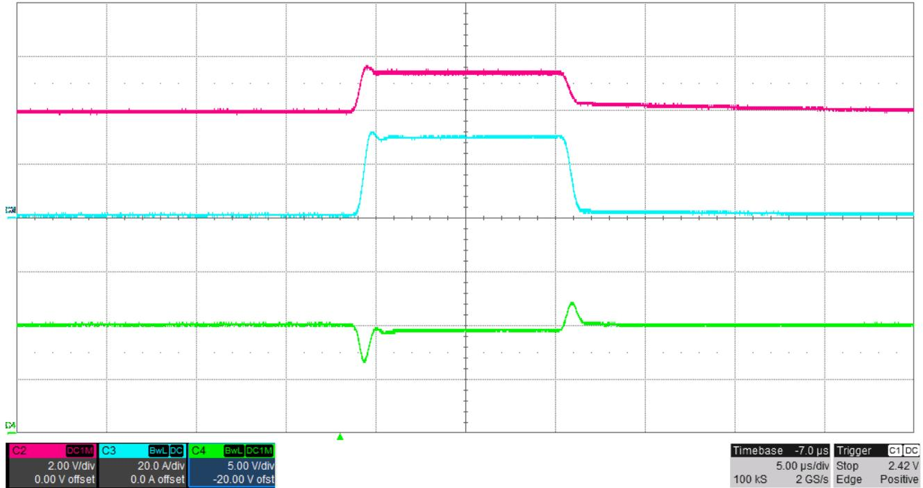
**Figure 3-16. Maximum Slew Rate, 10-V Output, 1-A to 30-A Critically Damped Load Transient**
