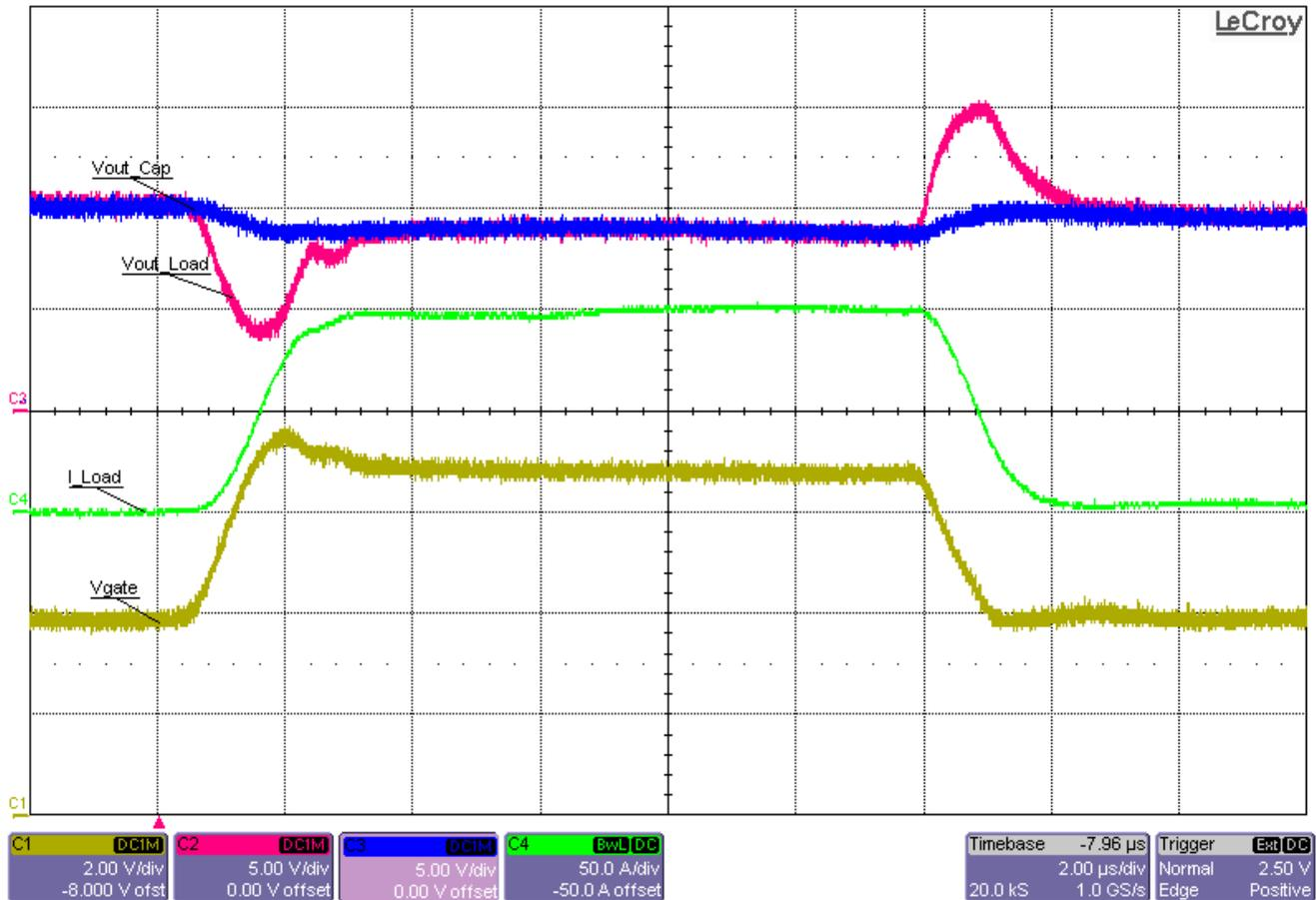
Figure 3-2. The Difference in Measuring Both Sides of the Capacitor Bank When Testing With the Chroma 62000p
