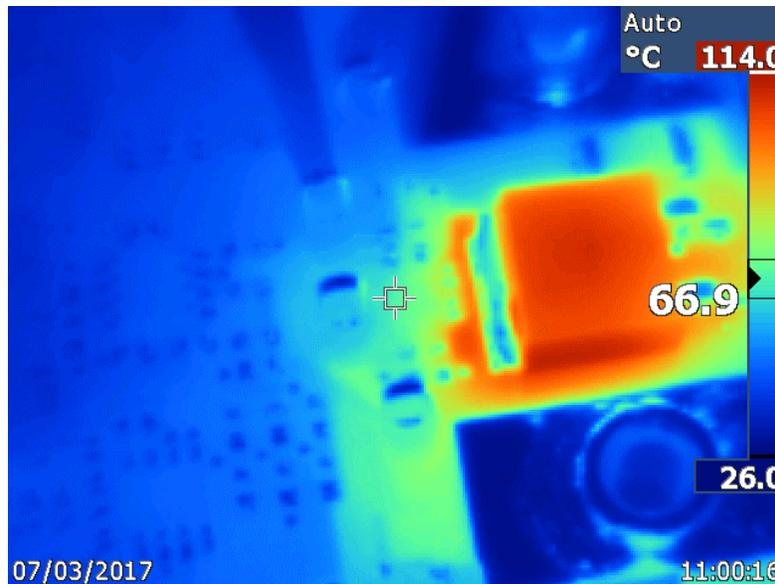
**Figure 3-11. LM26LVCISD-075, PSMN008-75B Load Step Board Thermal Shutdown**
