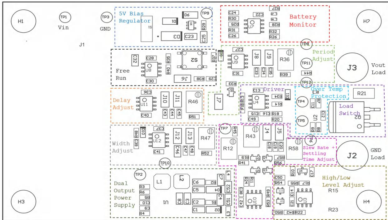
**Figure 2-1. Board Subcircuits**
