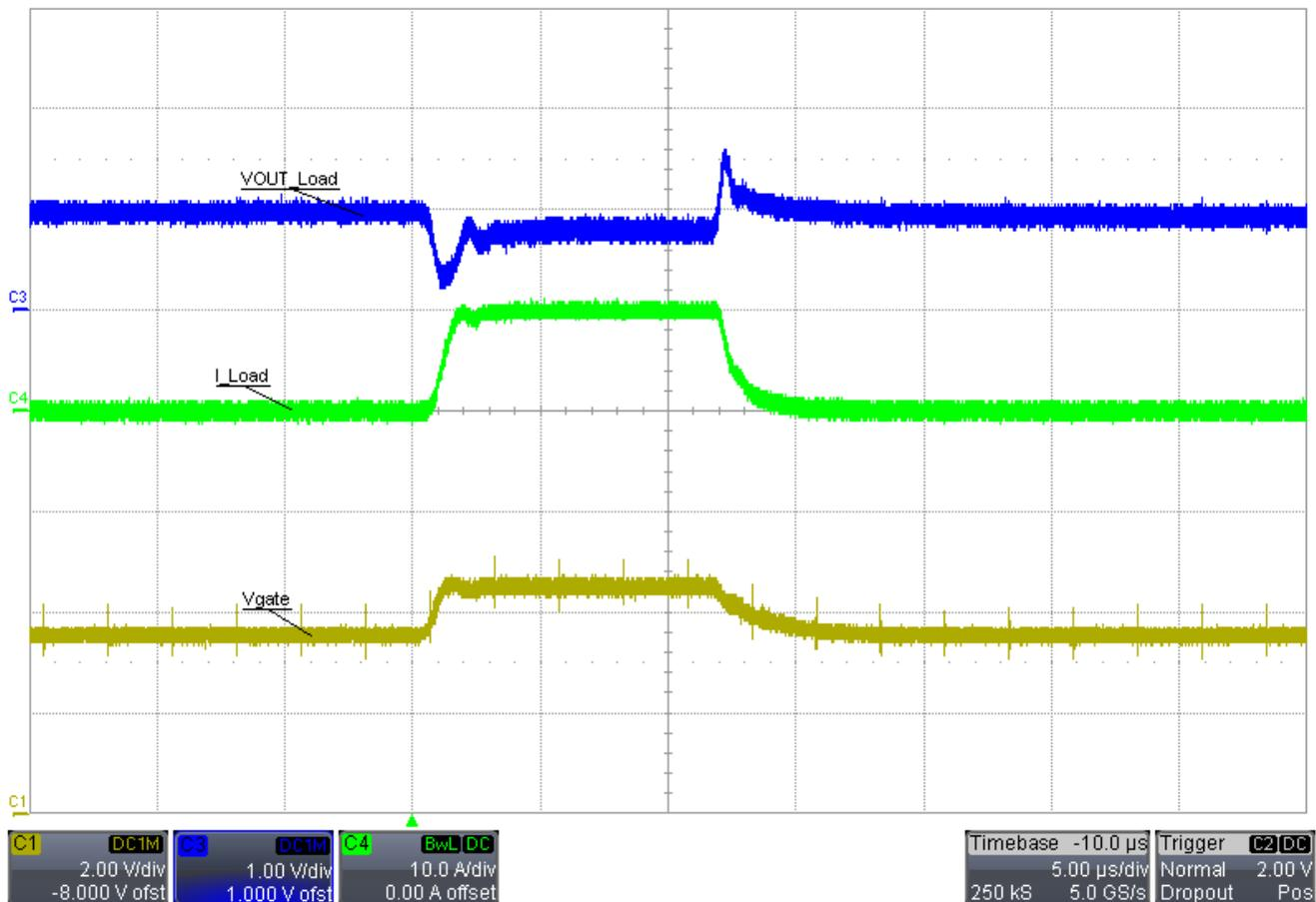
**Figure 5-1. Wiring Inductance Voltage Drop 1 A to 10 A, 1-V Output Load Transient**
