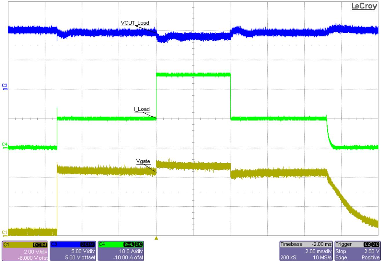
Figure 3-6. High-, Low-, Zero-Level Step, 10 A to 25 A, 10-V Output Load Transient
