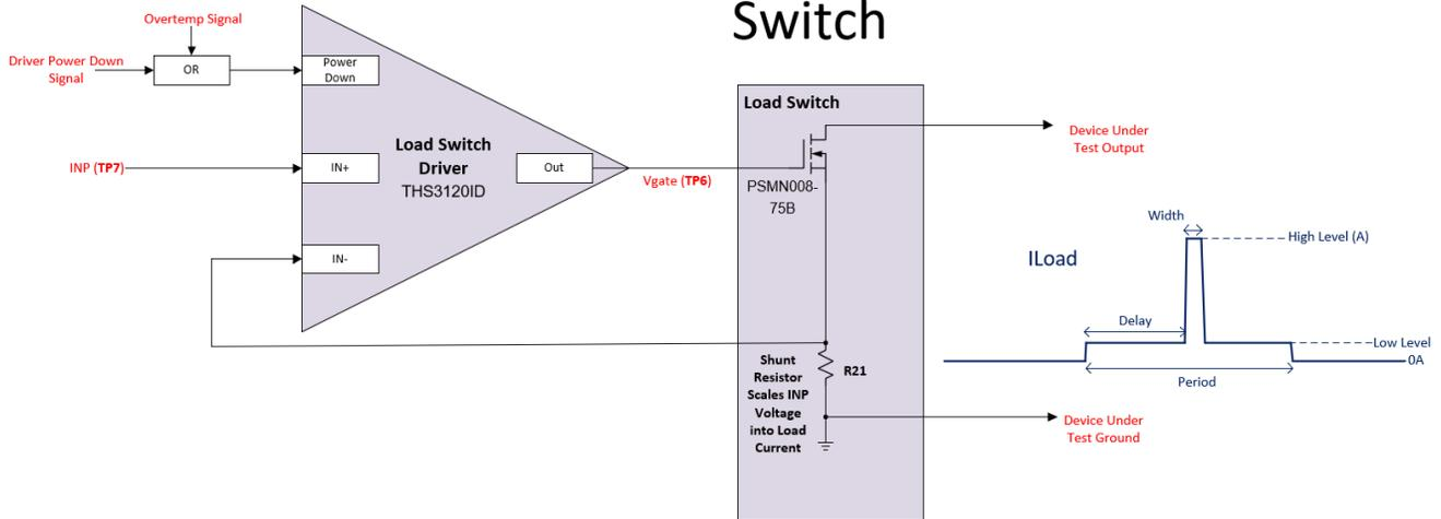
Figure 2-5. Driver and Load Switch
