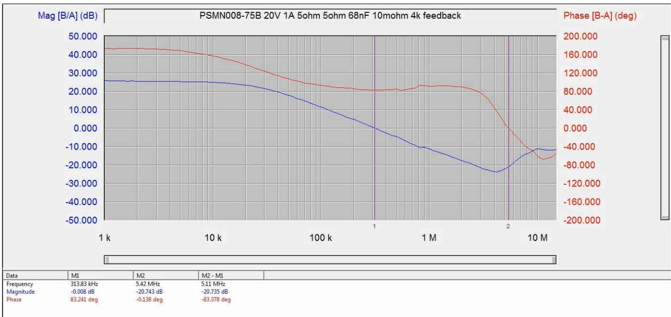
Figure 3-31. PSMN008-75B, 125-A Variant, 20-V, 1-A
