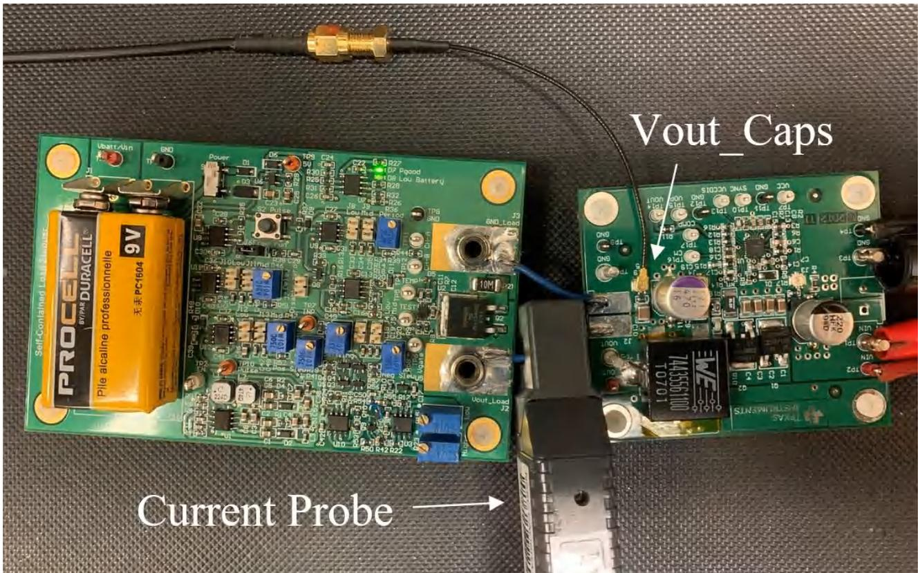
Figure 3-3. Setup for Using the Load Step Board With a Converter Under Test
