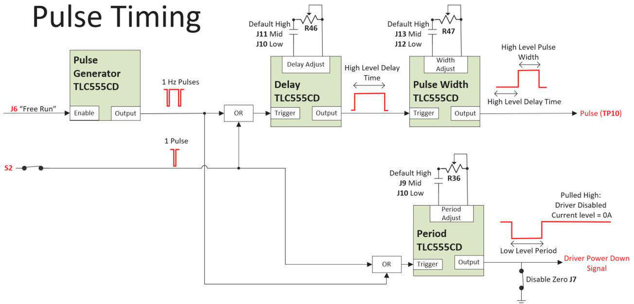
Figure 2-3. Pulse Timing
