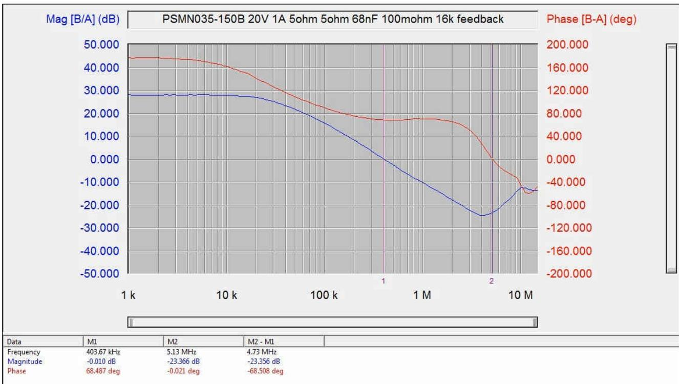
Figure 3-27. PSMN035-150B, 25-A Variant, 20-V, 1-A
