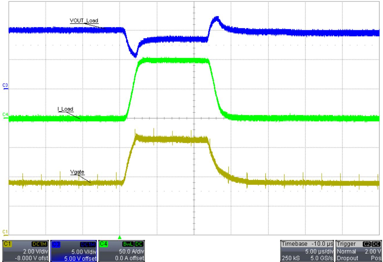
**Figure 3-13. 10-V Output, 1-A to 100-A Load Transient, 1  $\mu$ s Rise Time, Max Slew Rate**
