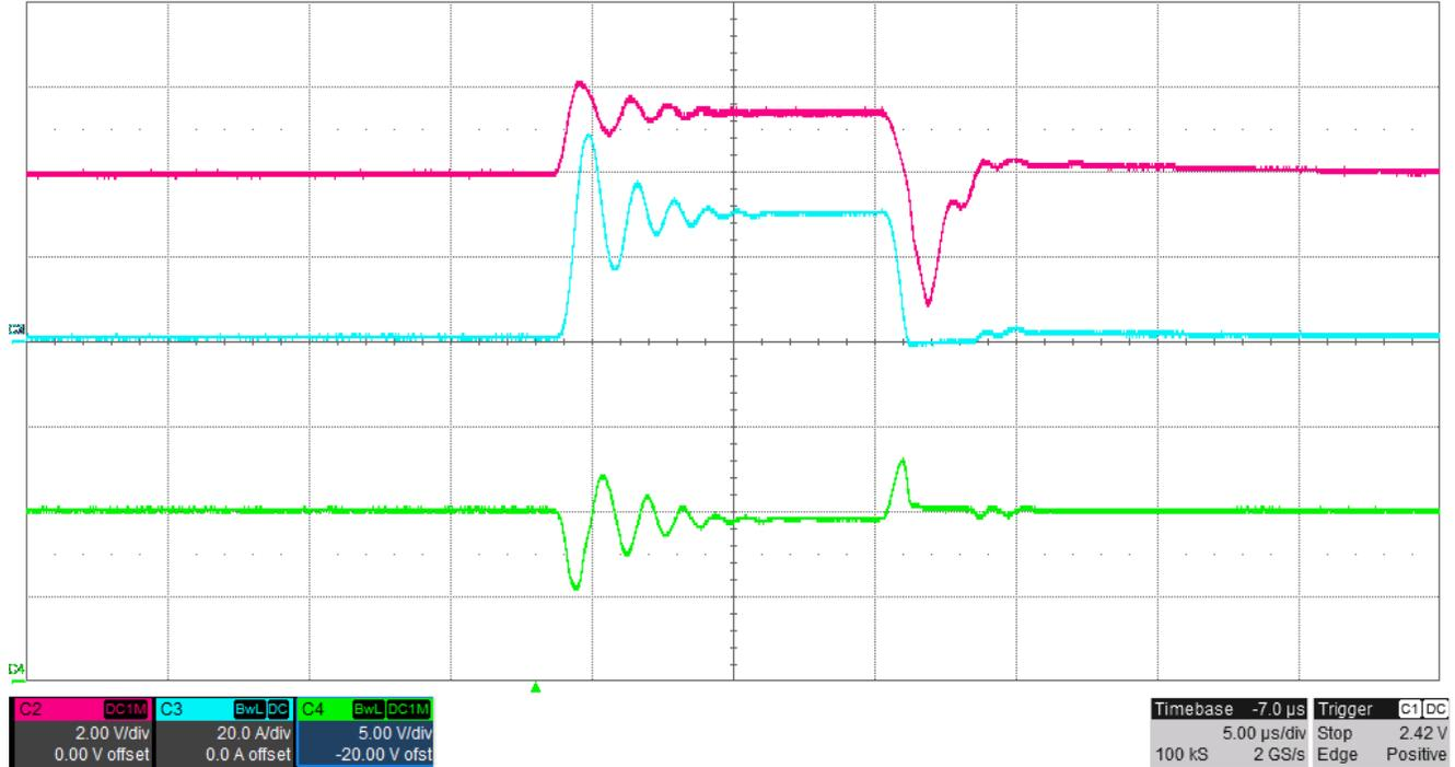
Figure 3-14. Maximum Slew Rate, 10-V Output, 1-A to 30-A Underdamped Load Transient
