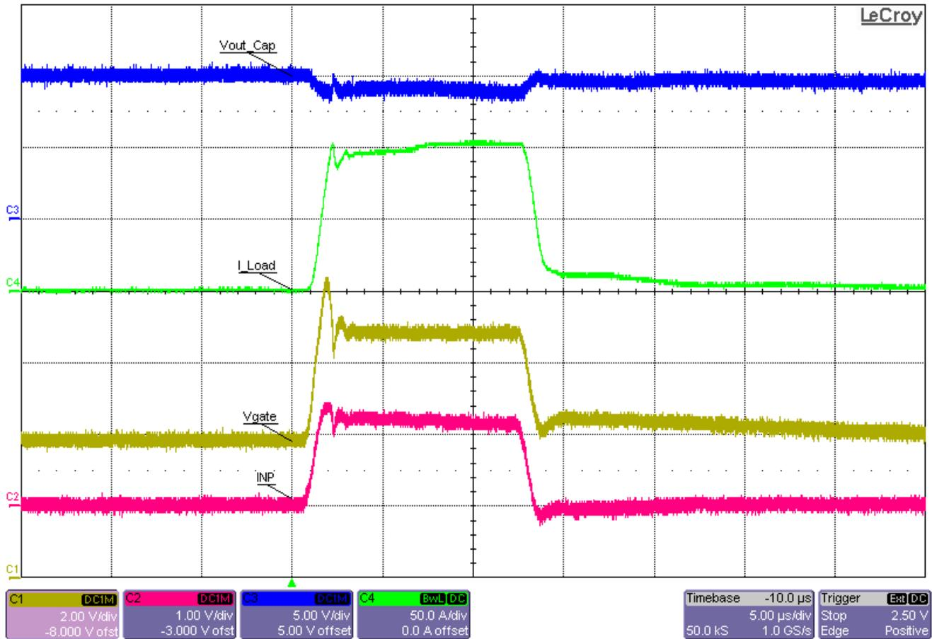
Figure 6-2. 1-A to 100-A Step, 10-V Output, Maximum Slew Rate, Replaced U4
