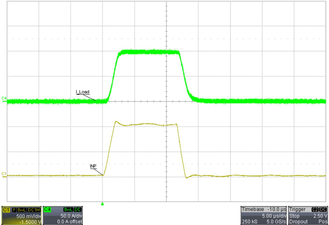
Figure 3-9. INP TLV431, 1 A to 100 A, 10-V Output Load Transient
