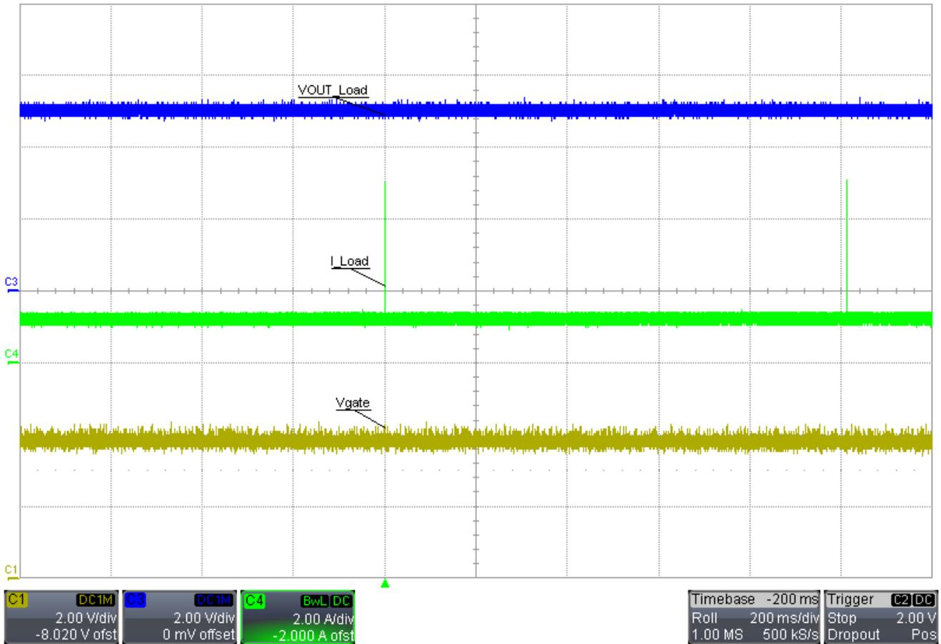
Figure 3-8. Disable Zero, 1 A to 5 A, 11  $\mu$ s, 5-V Output Load Transient
