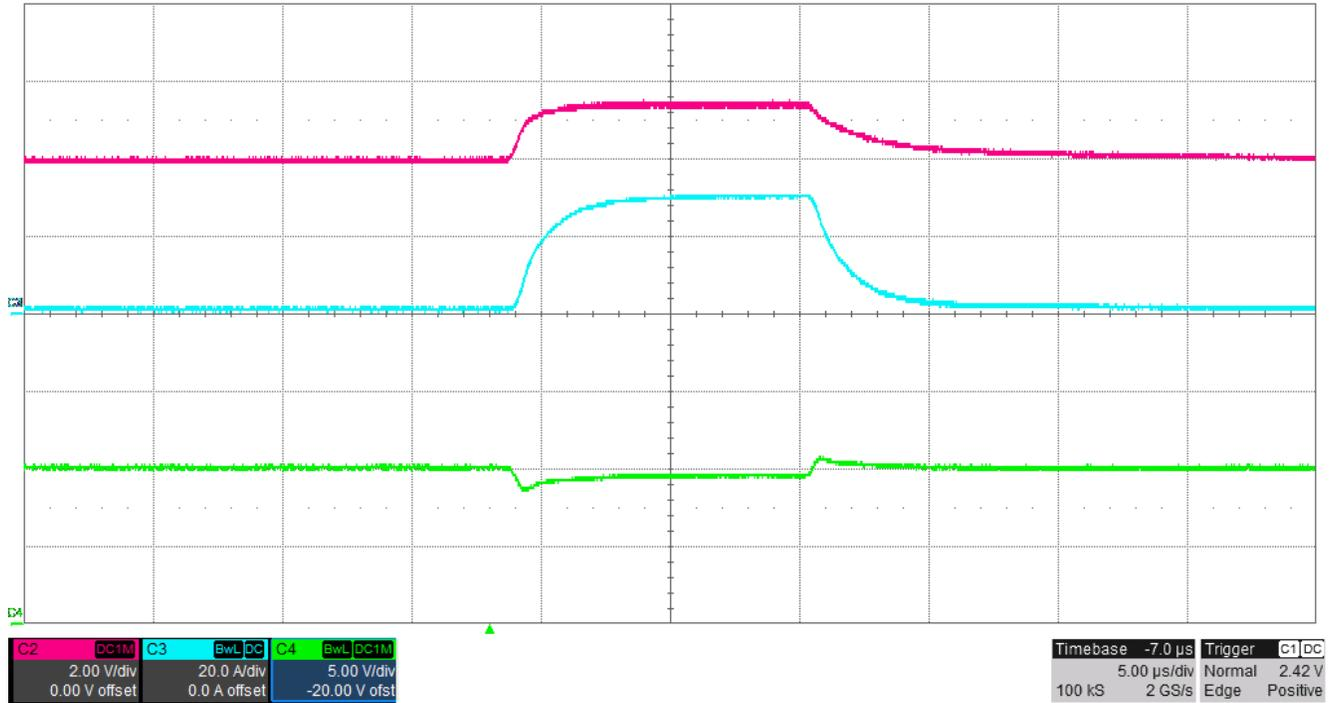
**Figure 3-15. Maximum Slew Rate, 10-V Output, 1-A to 30-A Overdamped Load Transient**
