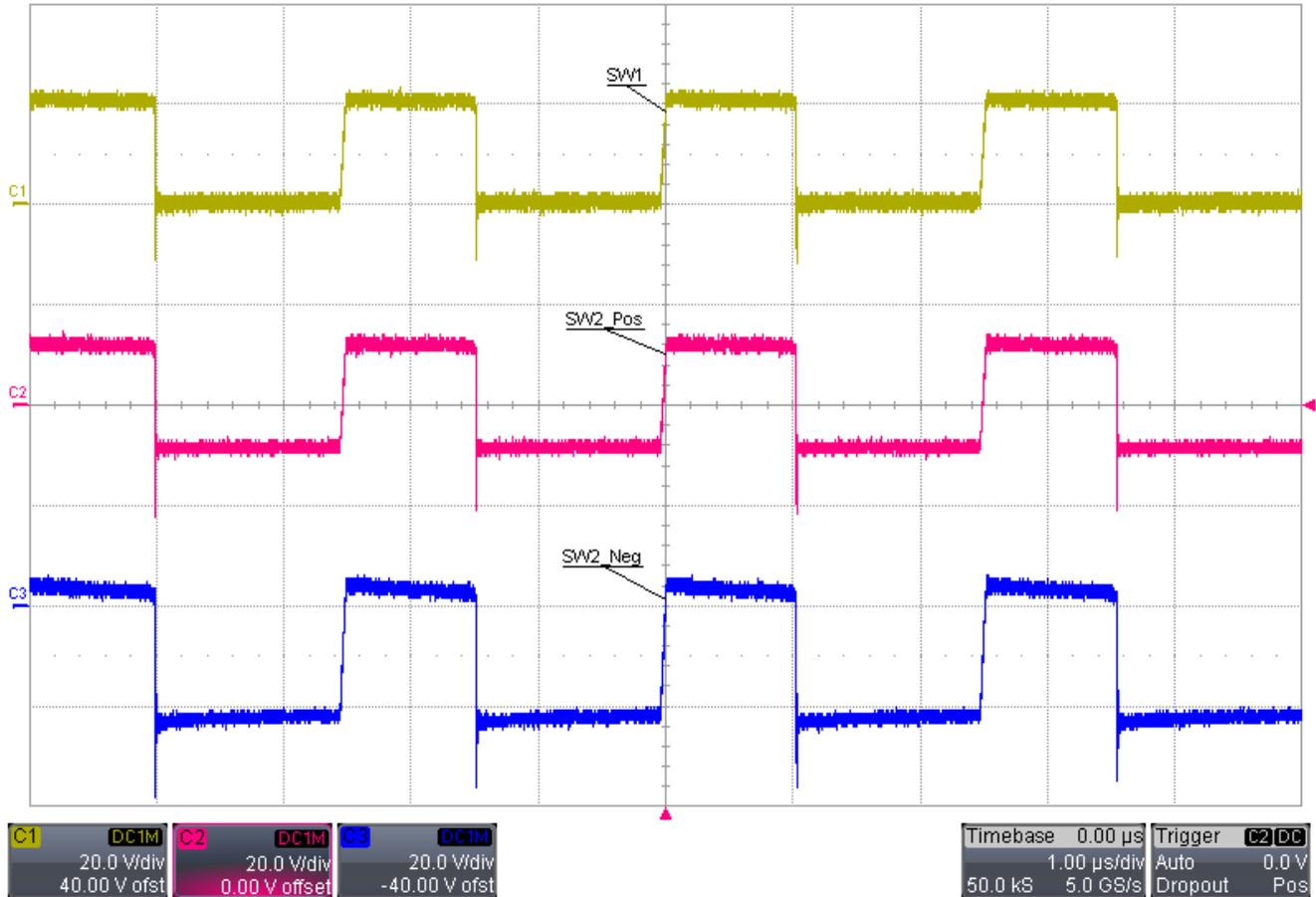
Figure 3-10. LM5002, 9-V Input, 12-V Positive and Negative Dual-Output Power Supply Switch Nodes
