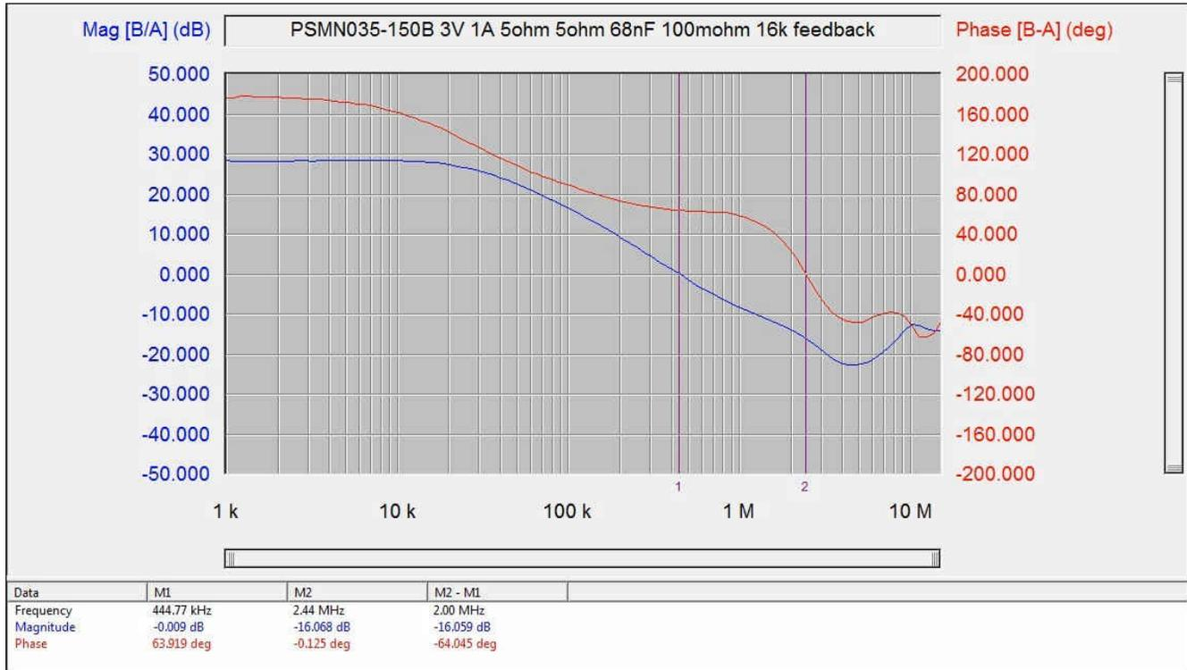
Figure 3-24. PSMN035-150B, 25-A Variant, 3-V, 1-A
