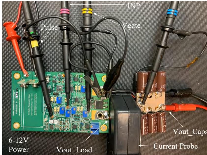
**Figure 3-1. Setup for Testing the Load Step Board Using a Power Supply**
