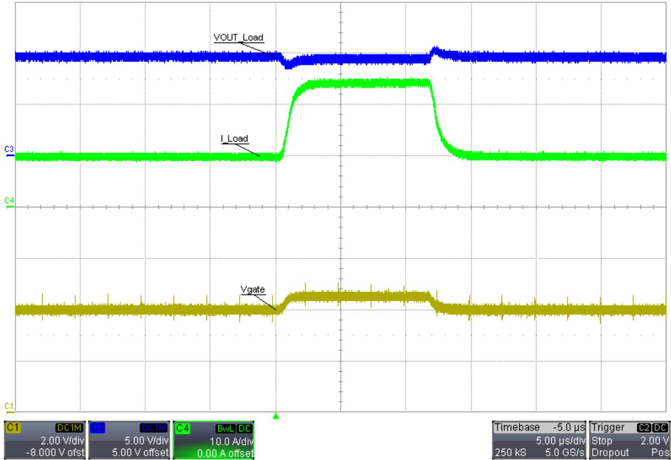
Figure 3-18. PSMN008-75B, 10-V Output, 10-A to 25-A Load Transient
