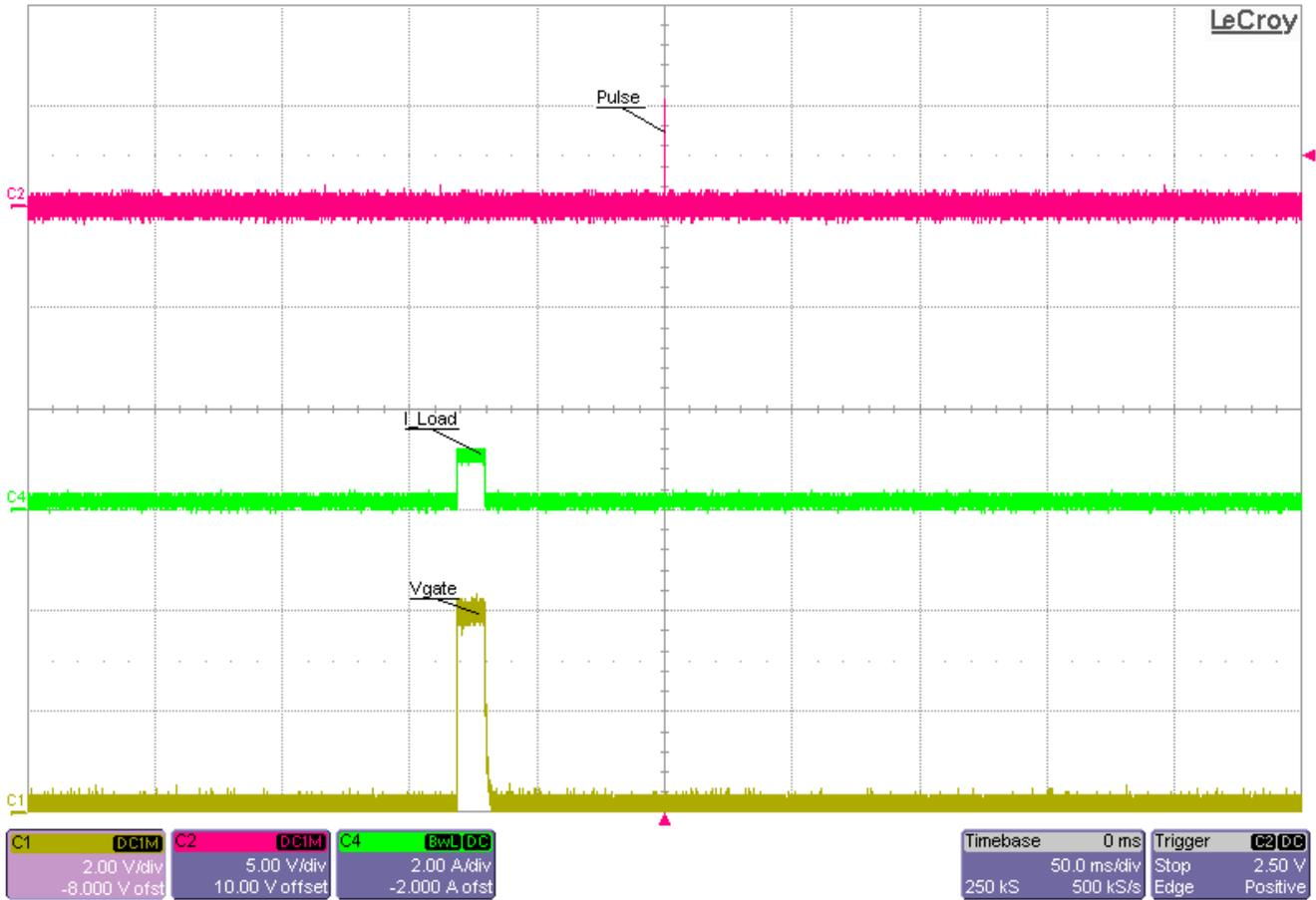
**Figure 3-23. Maximum Delay and Minimum Period Mistiming**
