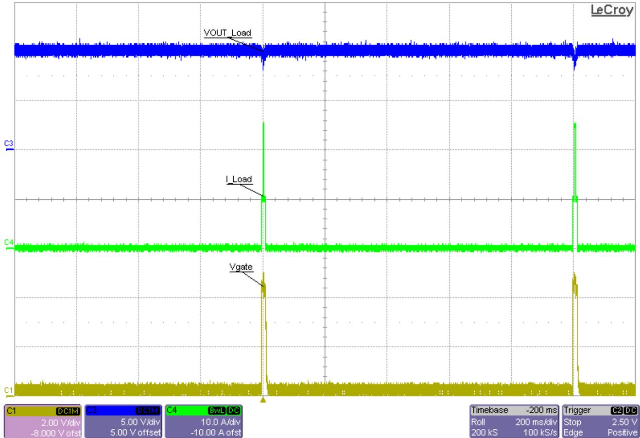
Figure 3-7. Free Run, 10 A to 25 A, 10-V<sub>OUT</sub> Load Transient
