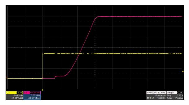
The photo below shows the 12 V output voltage startup waveforms after the application of 12 Vdc input. The output was loaded with to 1 A. (Vin is 5 V/DIV, Vout is 2 V/DIV, 10 mS/DIV)
