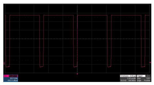
The photo below is the N-ch FET drain waveform. The input voltage is 10 V and the output is loaded to 0.1 A. The converter is operating in DCM. (20 V/DIV, 2 uS/DIV)
