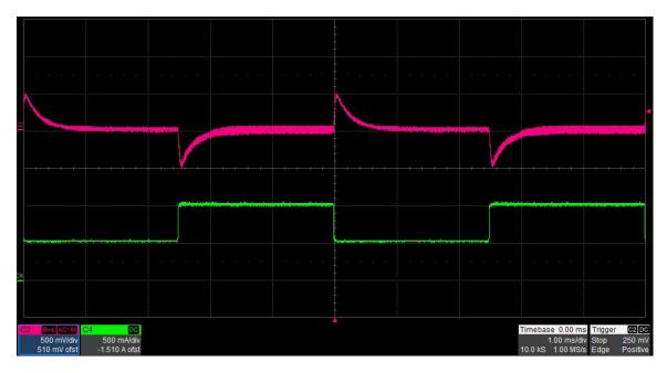
The photo below shows the 12 V output voltage (top, ac coupled) when the load current is stepped between 0.5 A to 1 A. Vin = 100V dc (500 mV/DIV, 500 mA/DIV, 1 mS/DIV)
