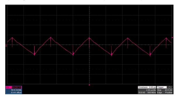
The 12 V output ripple voltage is shown in the figure below. The image was taken with the output loaded to 1 A and the input voltage set to 100 Vdc. (50 mV/DIV, 2 uS/DIV)
