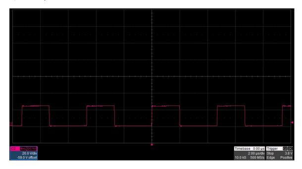
The photo below is the N-ch FET drain waveform. The input voltage is 100 V and the output is loaded to 1 A. (20 V/DIV, 2 uS/DIV)
