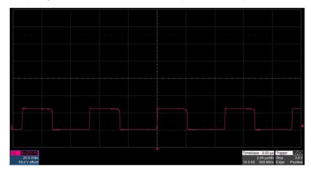
The photo below is the N-ch FET drain waveform. The input voltage is 100 V and the output is loaded to 0.45 A. The converter is operating in DCM. (20 V/DIV, 2 uS/DIV)
