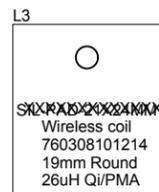
This coil is a stick-on and solder addition to the C02 PCB
