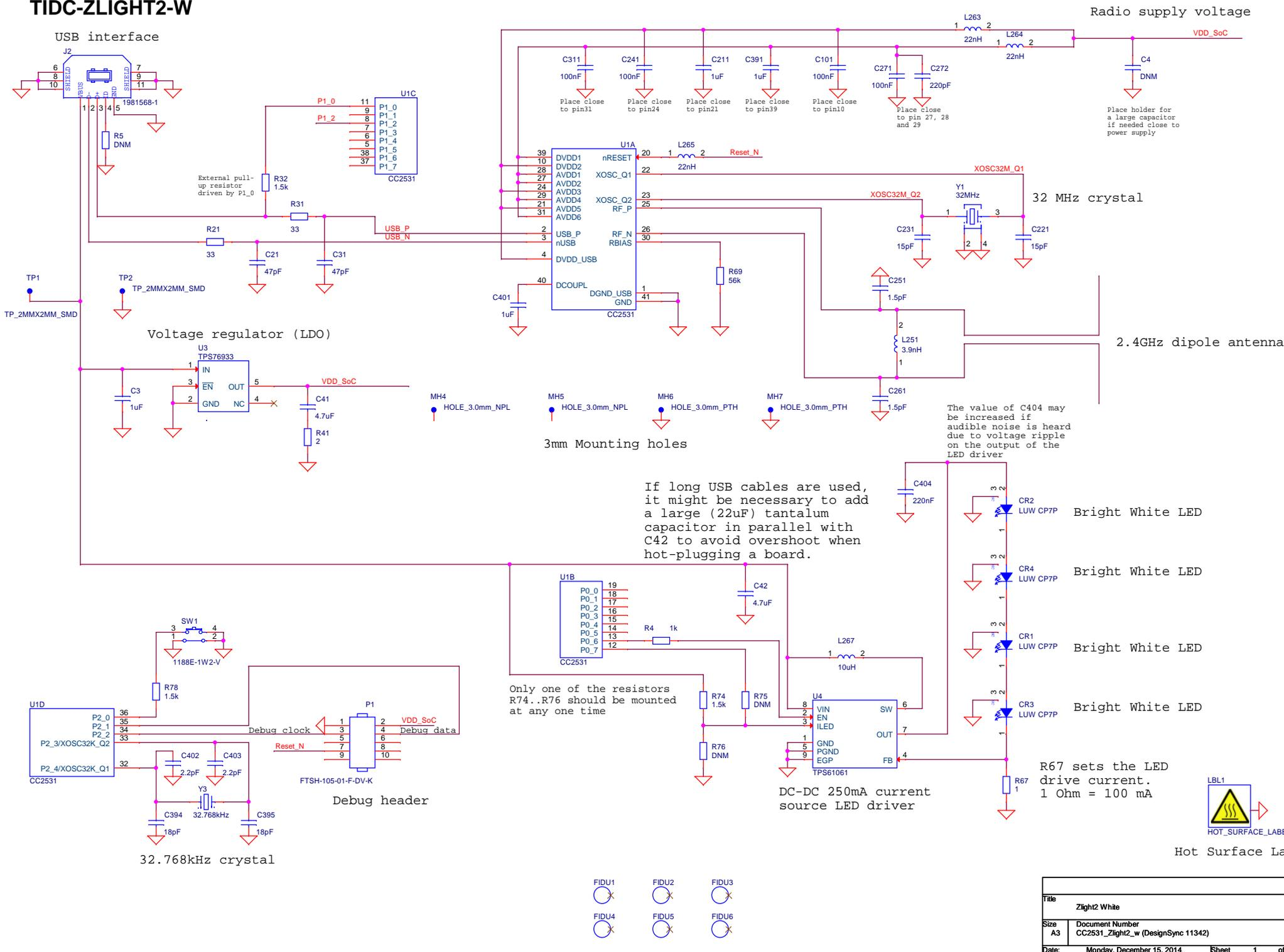
If long USB cables are used, it might be necessary to add a large (22uF) tantalum capacitor in parallel with C42 to avoid overshoot when hot-plugging a board.
