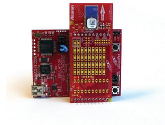
The RF BoosterPack includes an ETSI-compliant and FCC certified module integrating TI's CC110L sub-1 GHz RF value line transceiver, passive components and compact PCB antenna. For more information, visit [www.ti.com/rfboosterpack](http://www.ti.com/rfboosterpack)
