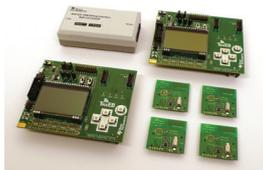
The **CC11xLDK-868-915** and **CC11xLEMK-433** development kits provide complete hardware performance testing and software development platforms for the Sub-1 GHz RF Value Line product family.
