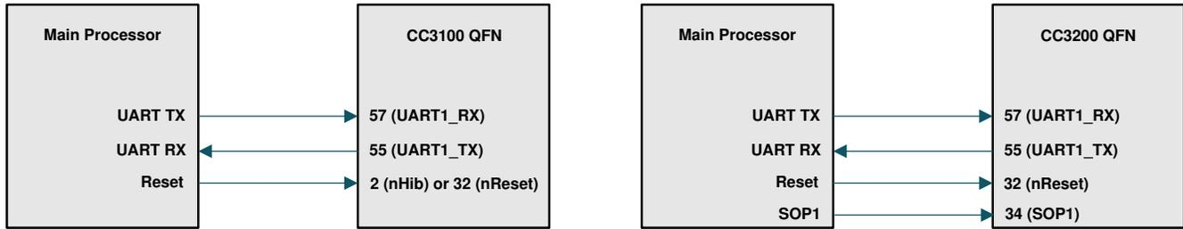
Figure 3-1. CC3100 and CC3200 QFN Programming Setup
