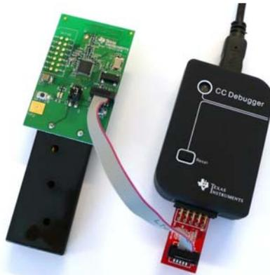
**Figure 7-1 – SmartRF CC2510 target board connected to CC Debugger**
