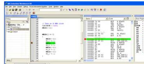
To develop software, program and debug the CC2510, the IAR Embedded Workbench for 8051 is recommended. An evaluation version of IAR EW8051 is included in the kit. This free evaluation version and also a free code size limited version, can also be downloaded from the web, see [www.iar.com/ew8051](http://www.iar.com/ew8051).
