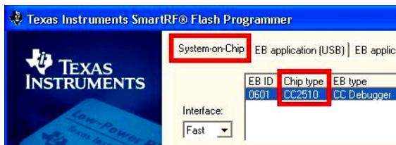
The Flash Programmer application, available on the kit web page <http://focus.ti.com/docs/toolsw/folders/print/flash-programmer.html> can be used to program Intel HEX files, read the contents of CC2510 flash, and several other operations.
