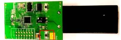
Note that the board only responds to the first button push. To reconfigure the board, the board must be reset, see point 2.8 in this manual.
