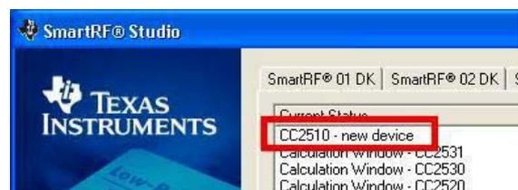
SmartRF Studio can be used for RF testing, evaluation of CC2510 and to find optimal register settings. It is available on <http://www.ti.com/smrtfstudio>.
