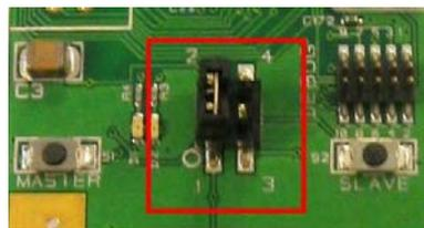
Applying power to the SmartRFCC2510 starts the preprogrammed link test on the CC2510 and the two LEDs on the board are on for 1 s.
