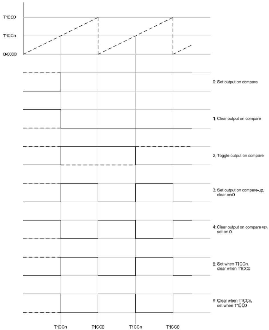
**Figure 2. Pulse Width in Modulo Mode**
