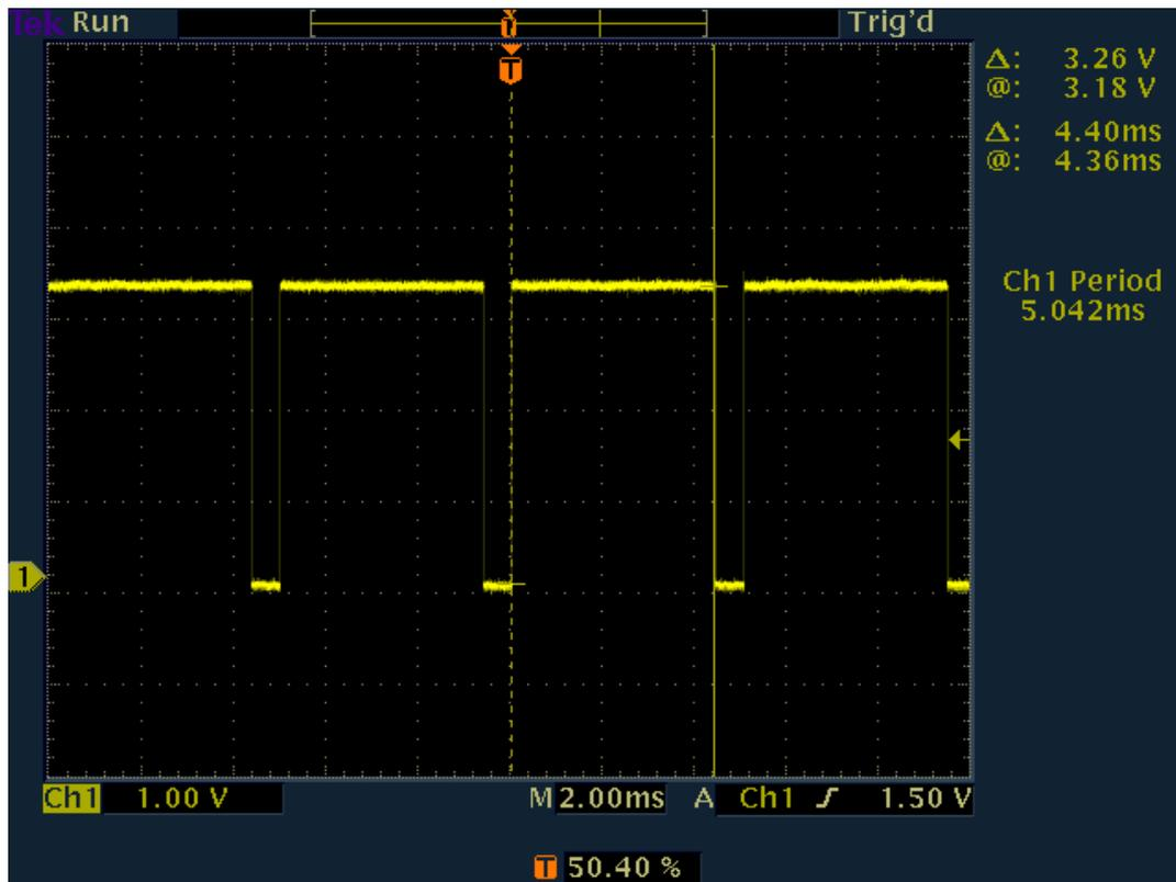
Figure 4. 7/8 duty PWM Signal
