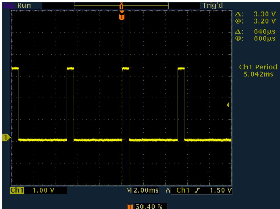
Figure 3. 1/8 duty PWM Signal
