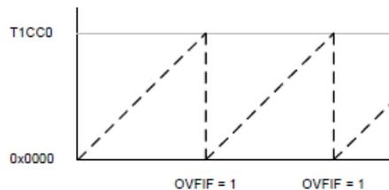
Figure 1. Frequency in Modulo Mode
