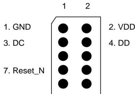
**Figure 15: Recommended debug connector layout (Top view)**
