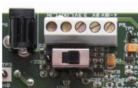
**Figure 4. SmartRF04EB Power Switch, Power On**
