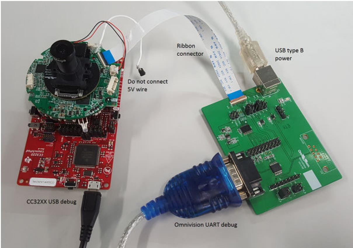
**Figure 2-6. RS232 Debug Board Setup**
