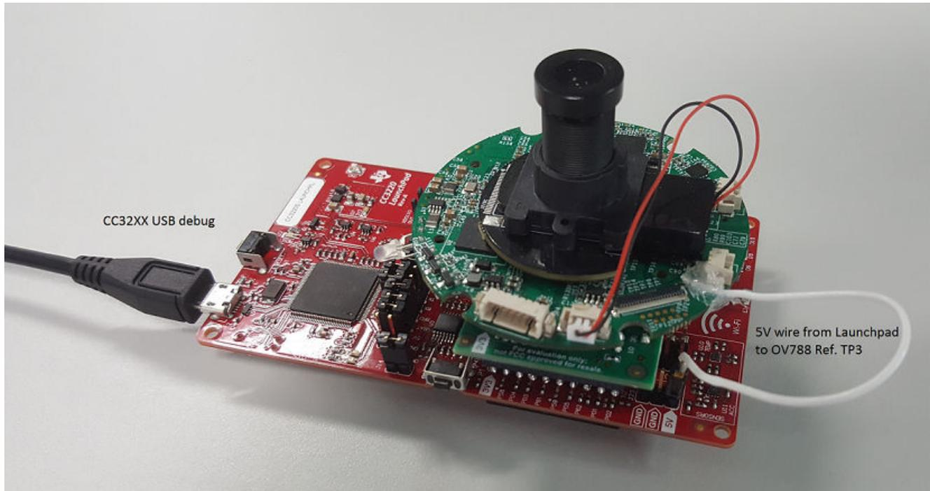
**Figure 2-5. CC3220 LaunchPad Setup**
