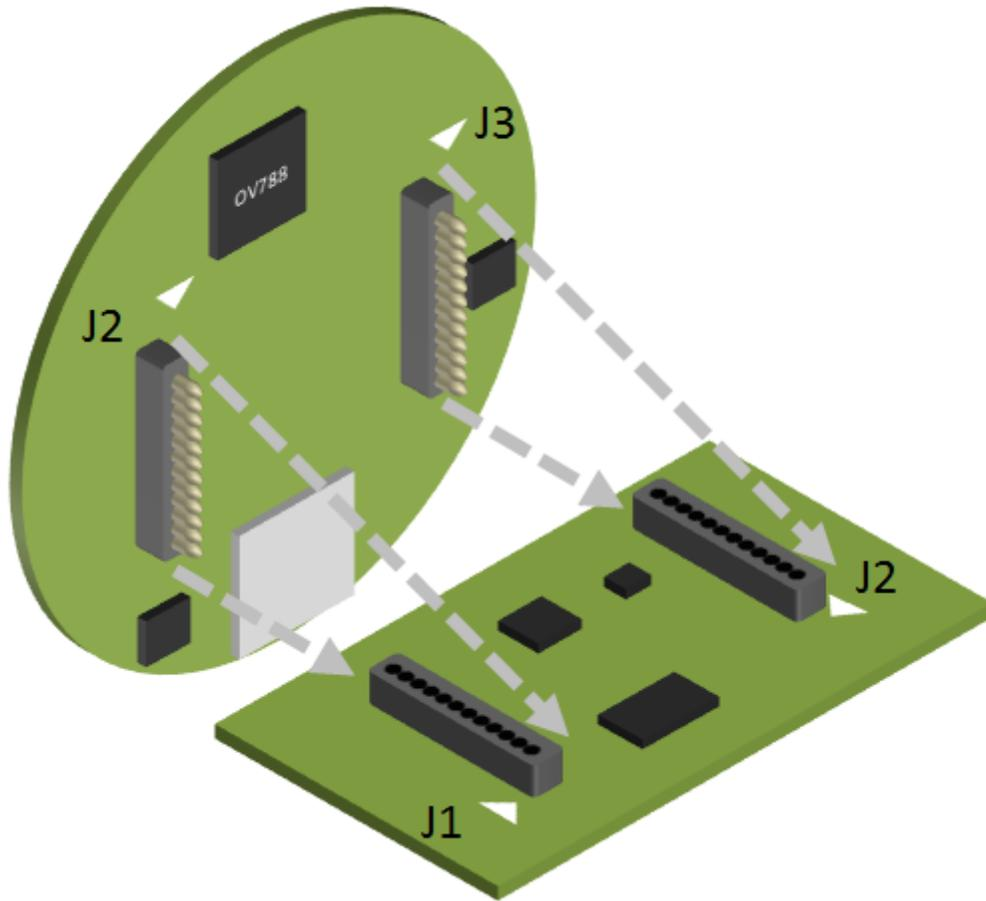
**Figure 2-4. OV788 Adapter Booster Pack Connection**
