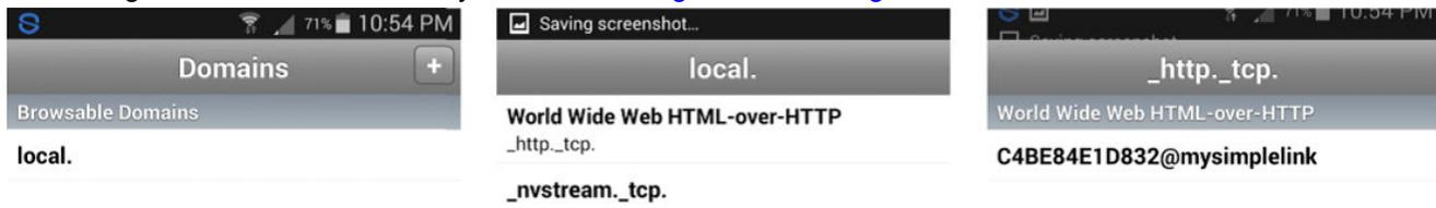
**Figure 3-5. mDNS Device Discovery**
