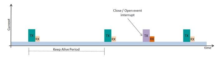
Figure 2. Power Profile for Door and Window Sensor
