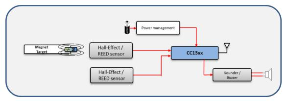
Figure 1. Wireless Door and Window Sensor Block Diagram
