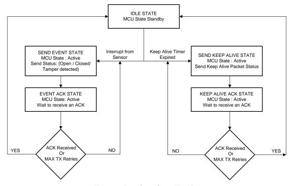
Figure 3. Test-Case State Machine
