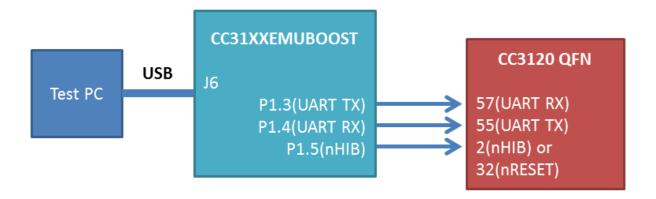
Figure 5. Programming Through USB
