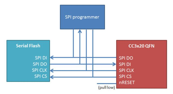
Figure 2. Programming Through SPI
