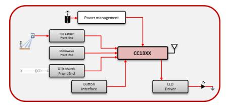
Figure 3-1. Motion Detection System Block Diagram
