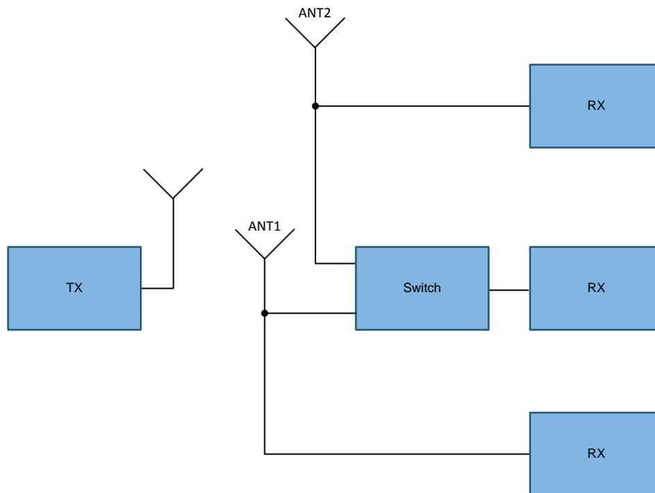
**Figure 7. Block Diagram of Antenna Diversity Test Setup**
