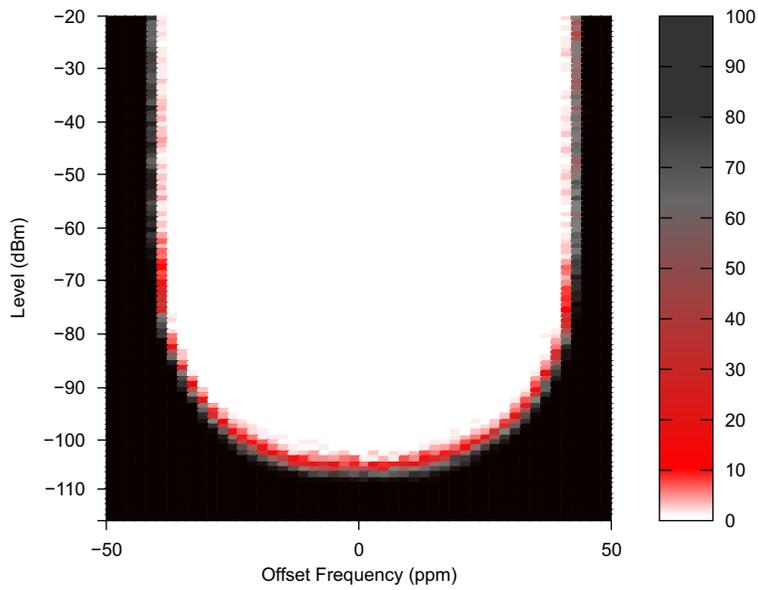
**Figure 6. PER vs Input Power Level
