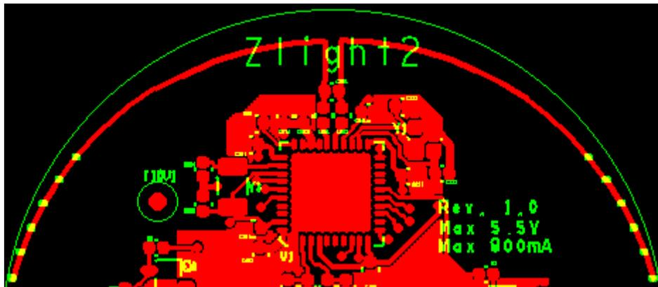
Figure 8. First Prototype Layout with Tuning Marks and Filtering Components
