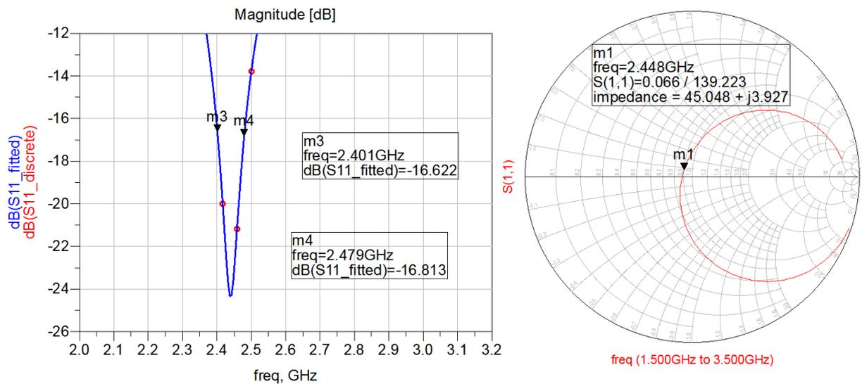
**Figure 5. S11 Looking into the Curved Dipole**
