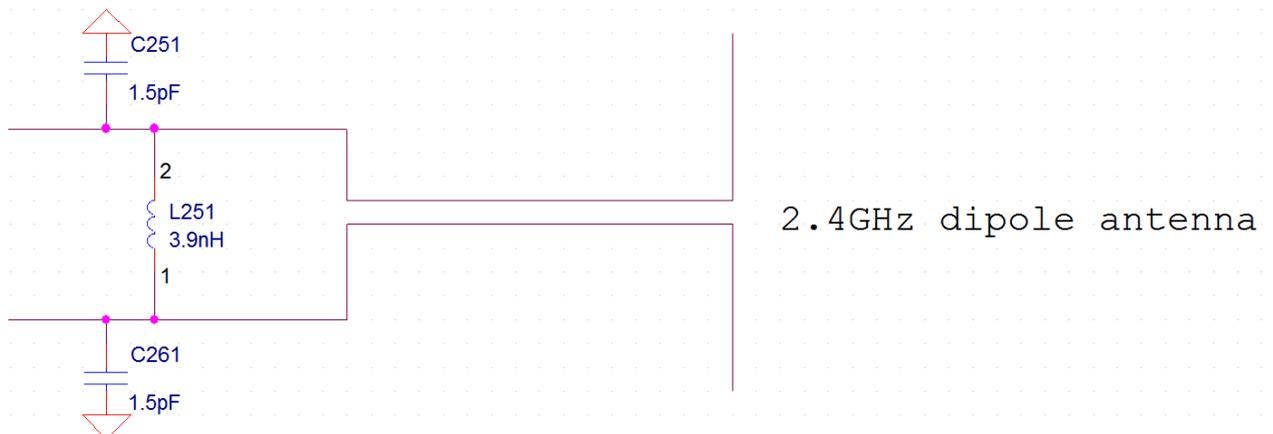
Figure 10. Parallel Resonant Circuit with Differential as well as Common Mode Rejection
