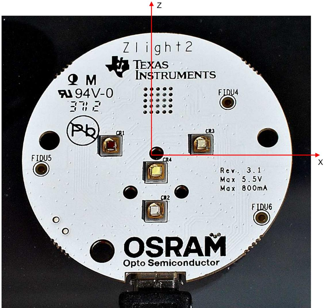
Figure 12. Board Orientation During the Antenna Measurements
