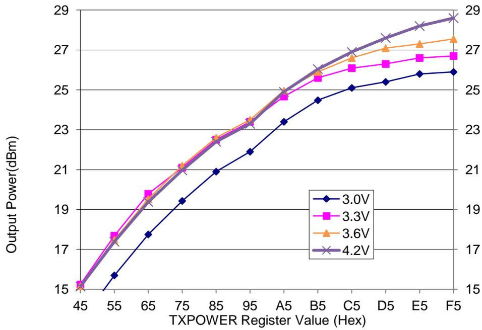
**Figure 4-2 Typical Output Power vs. CC2530 TXPOWER Setting over Voltage**
