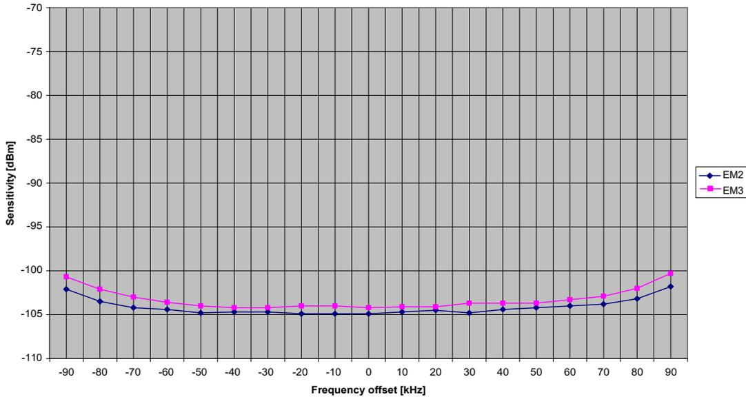
Figure 5. Sensitivity at PER 20 % versus Frequency Offset
