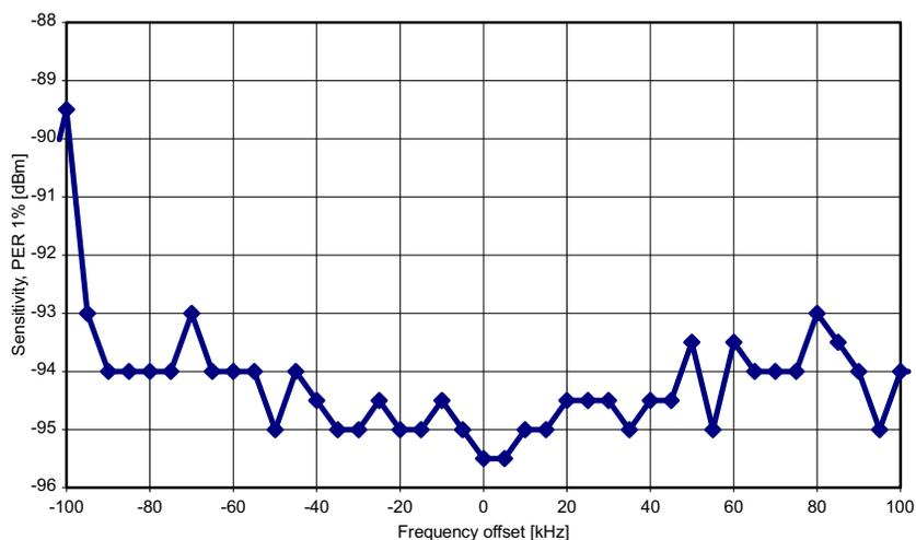
**Figure 10. 250 kbps, MDMCFG2.DEM\_DCFILT\_OFF = 0**
