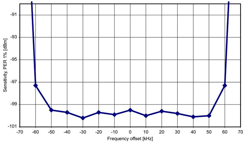
**Figure 9. 38.4 kbps, MDMCFG2.DEM\_DCFILT\_OFF = 1**
