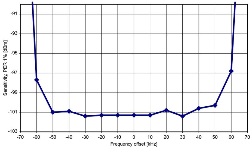
**Figure 8. 38.4 kbps, MDMCFG2.DEM\_DCFILT\_OFF = 0**
