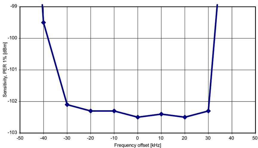
Figure 6. 10 kbps, MDMCFG2.DEM\_DCFILT\_OFF = 0
