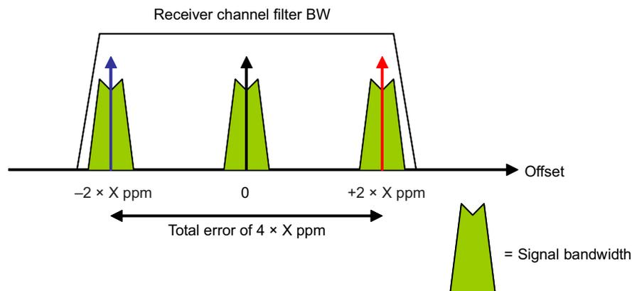
**Figure 1. Plot of IF Versus Frequency Error**
