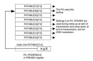
Figure 2. PA\_POWER and PATABLE
