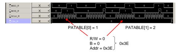
Figure 5. Single Byte Access with CSn Kept Low
