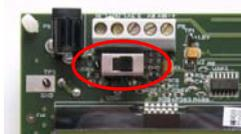
Figure 4. Power Switch S3 on SmartRF<sup>®</sup>04EB
