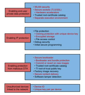
Figure 6-5. E-Lock Security Challenges and SimpleLink™ Wi-Fi Security Enablers
