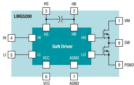
**Figure 9.** LMG5200: 80 V/10 A GaN Half-Bridge Power Stage.
