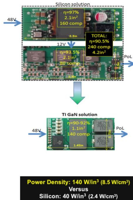
Figure 5. Two POL stages to a single stage.
