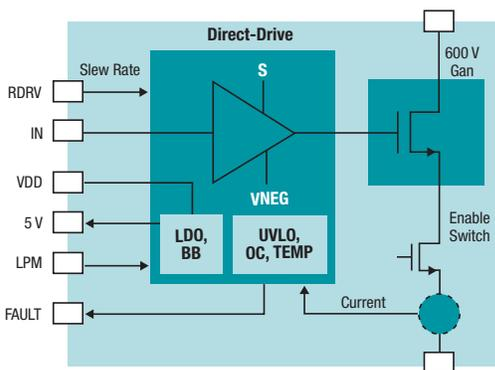
**Figure 8.** LMG3410: 600V/70 mΩ 12A GaN Power Stage.
