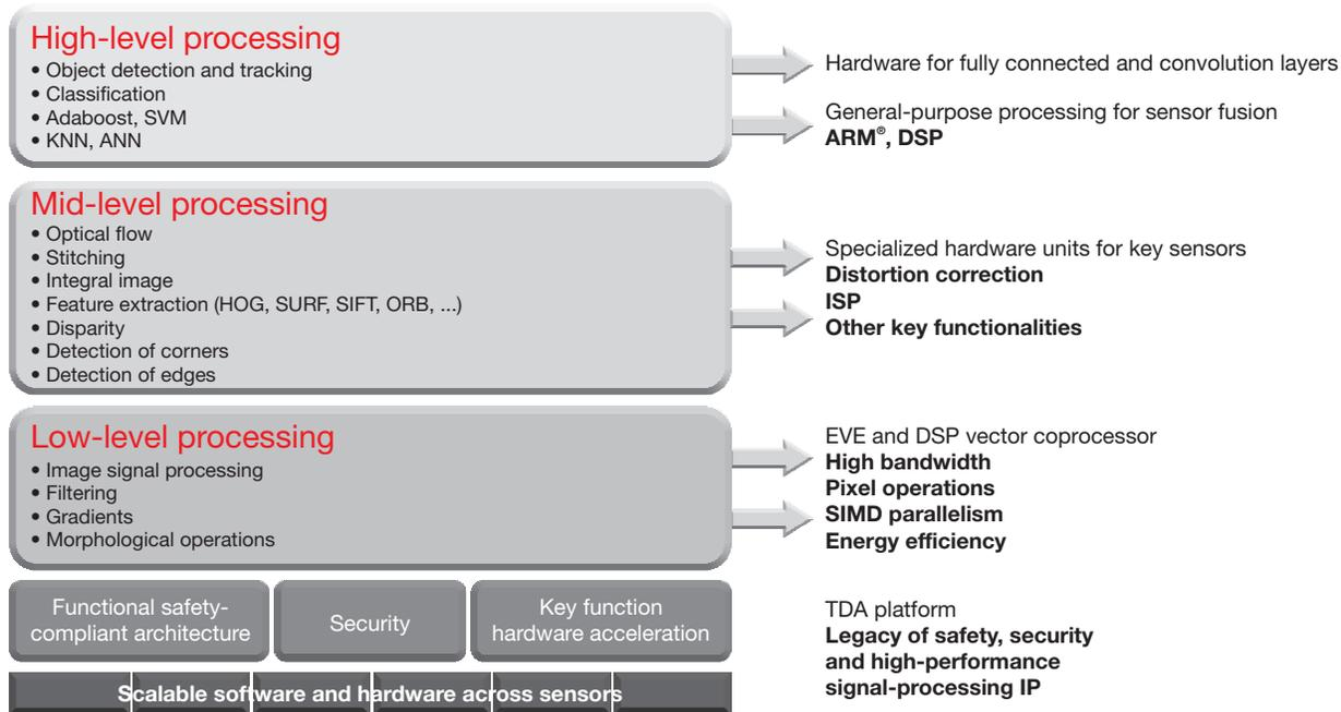
**Figure 3.** Mapping functions to the right processing architecture.
