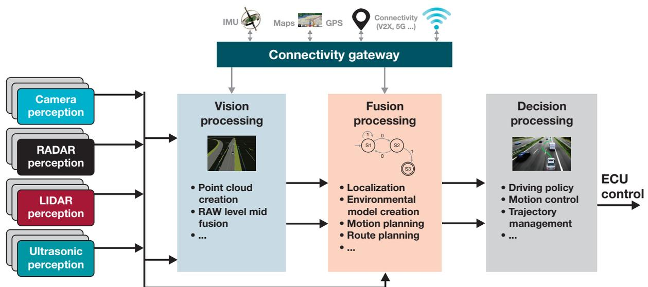
**Figure 2.** Typical Level 3 to Level 5 system architecture.
