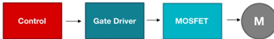
**Figure 1. Basic motor-control block diagram**
