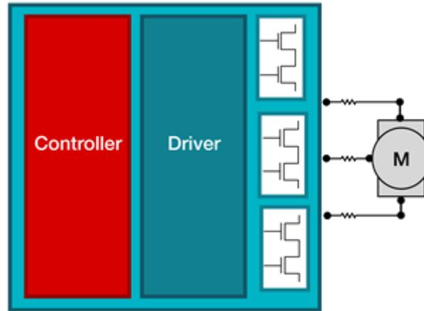
**Figure 6. Fully integrated – motor control plus driver plus FETs**
