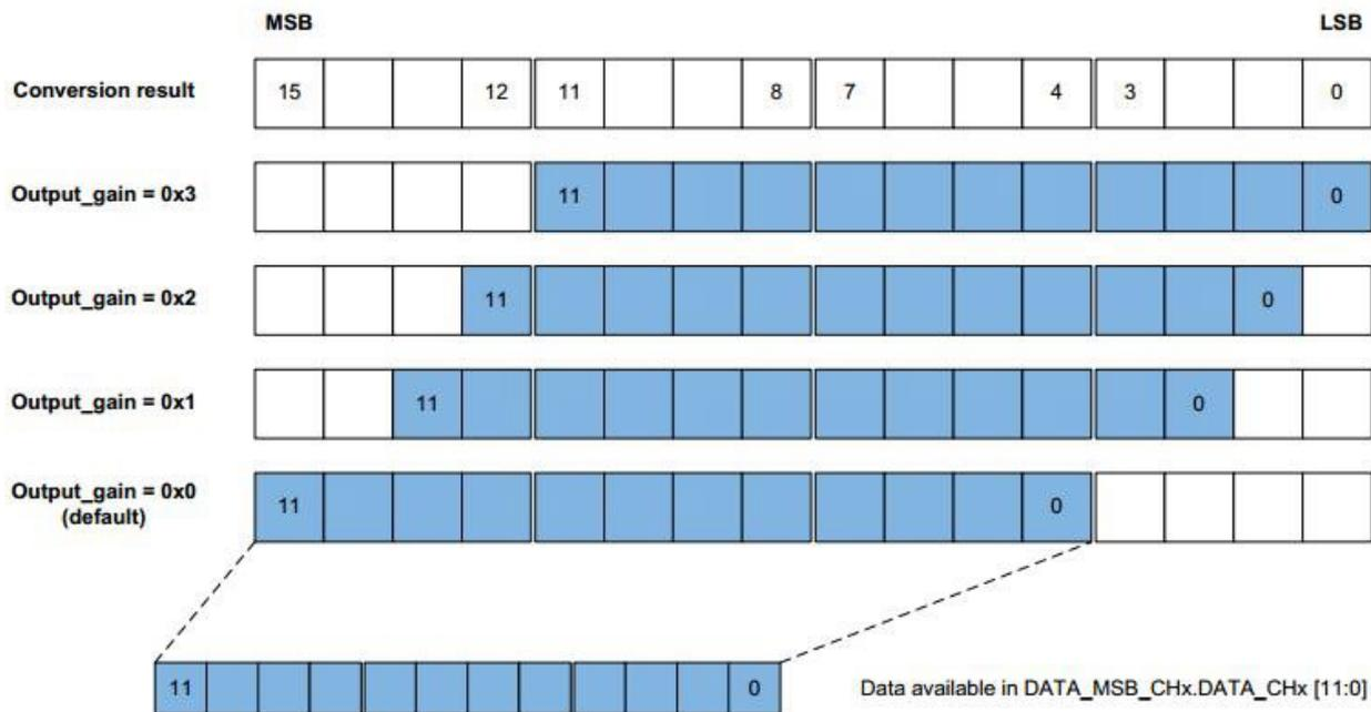
Figure 1. Conversion Data Output Gain
