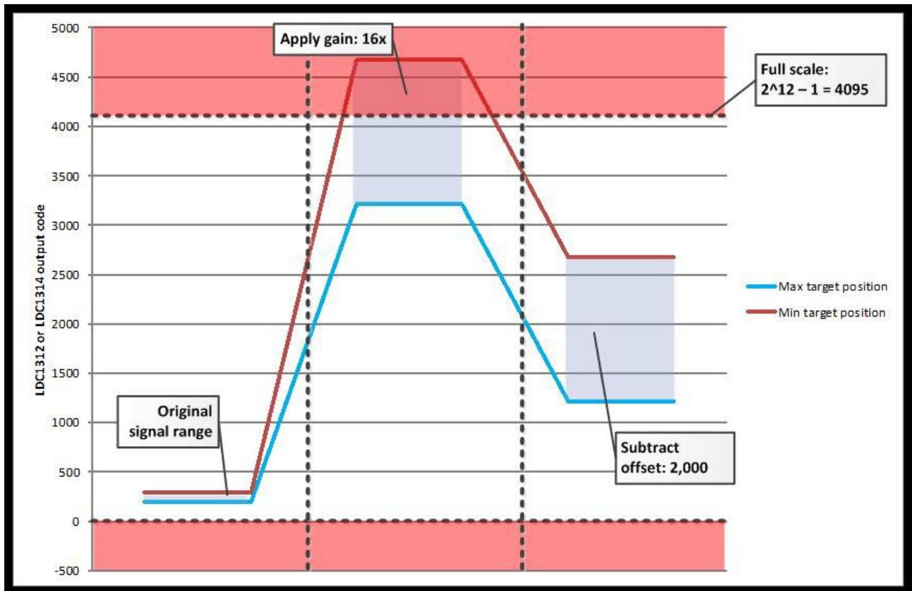
**Figure 2. Conversion Signal Range Increases after Applying Gain and Offset**
